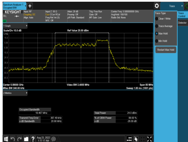
Plot 7-27. 26dB BW & 99% OBW Antenna 3c (20MHz BW 11ax Index 40 – RU52 – Ch.116)
