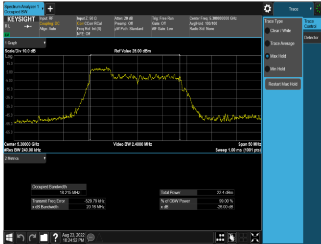
Plot 7-49: 26dB BW & 99% OBW Antenna 3a (20MHz BW 11ax Index 37 – RU52 – Ch.60)
