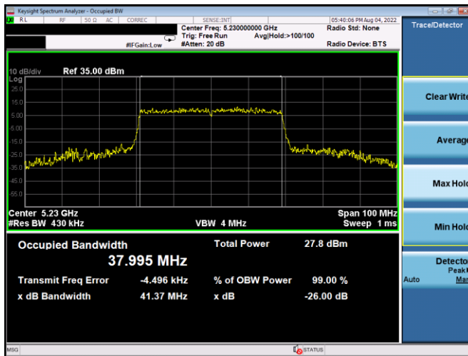
Plot 7-8. 26dB BW & 99% OBW Antenna 3c (40MHz BW 11ax - RU484 - Ch.46)
