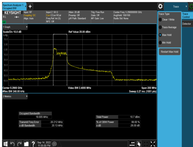
Plot 7-21. 26dB BW & 99% OBW Antenna 3c (80MHz BW 11ax Index 37 – RU52 – Ch.58)
