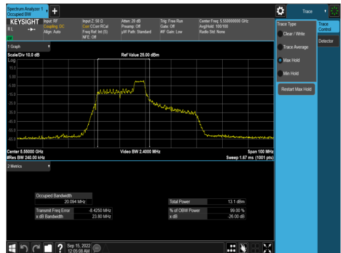
Plot 7-30. 26dB BW & 99% OBW Antenna 3c (40MHz BW 11ax Index 40 – RU52 – Ch.110)
