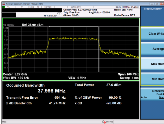
Plot 7-20. 26dB BW & 99% OBW Antenna 3c (40MHz BW 11ax – RU484 – Ch.54)
