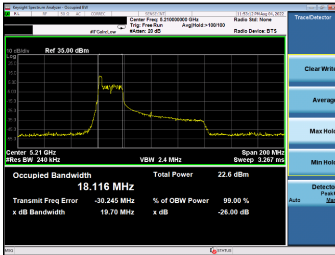
Plot 7-45. 26dB BW & 99% OBW Antenna 3a (80MHz BW 11ax Index 0 – RU26 – Ch.42)
