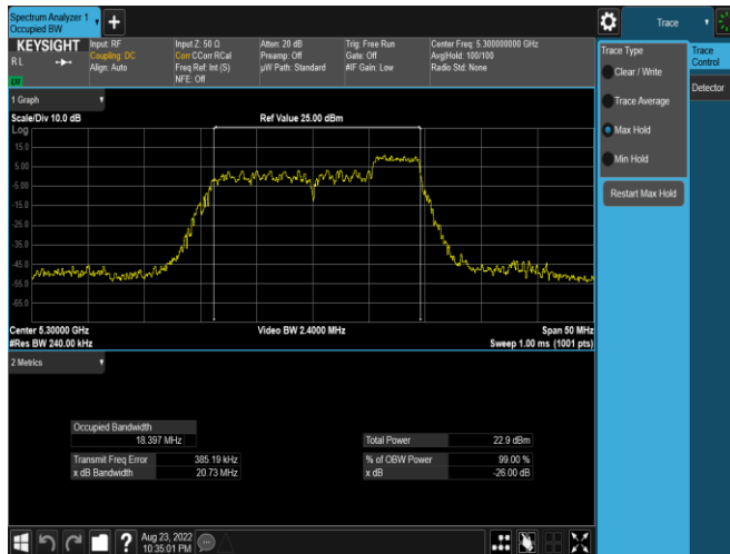
Plot 7-51: 26dB BW & 99% OBW Antenna 3a (20MHz BW 11ax Index 40 – RU52 – Ch.60)
