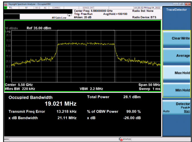
Plot 7-28. 26dB BW & 99% OBW Antenna 3c (20MHz BW 11ax – RU242 – Ch.116)
