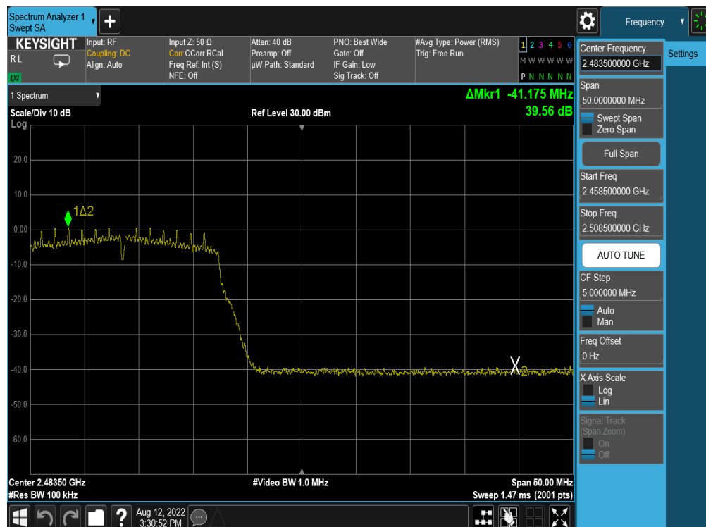
Plot 7-200. Band Edge Plot Antenna 3a (802.11n – Ch. 12) – MCS2
