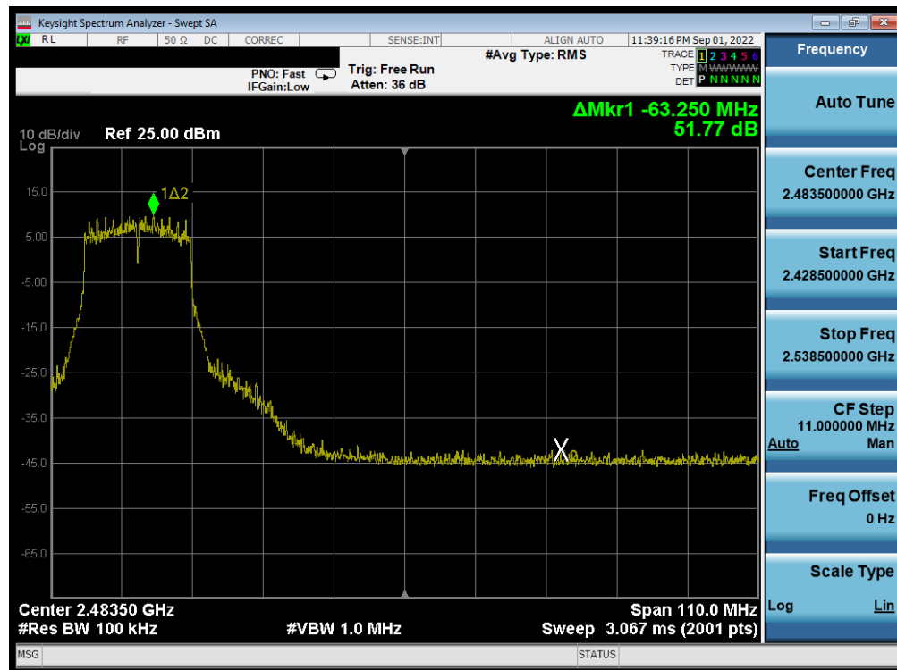
Plot 7-222. Band Edge Plot Antenna 3a (802.11g - Ch. 7) – 24Mbps
