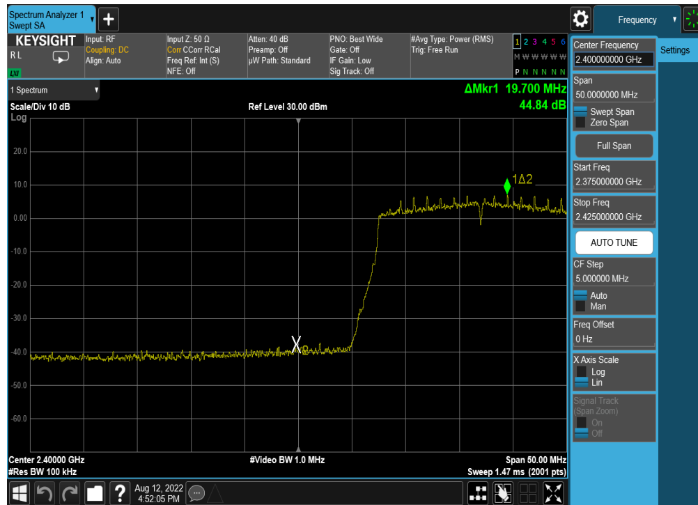
Plot 7-203. Band Edge Plot Antenna 3a (802.11ax(SU)– Ch. 2) – MCS2
