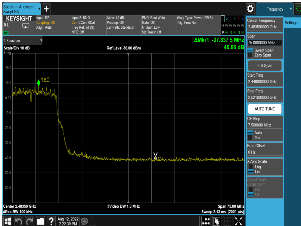
Plot 7-272. Band Edge Plot Antenna 3a (802.11g - Ch. 9) - 36Mbps
