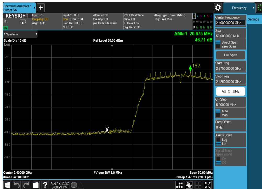
Plot 7-190. Band Edge Plot Antenna 3a (802.11n- Ch. 2) – MCS2
