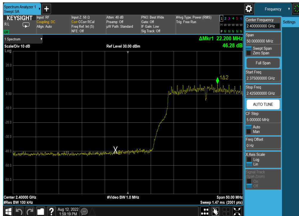
Plot 7-264. Band Edge Plot Antenna 3a (802.11g- Ch. 2) – 36Mbps
