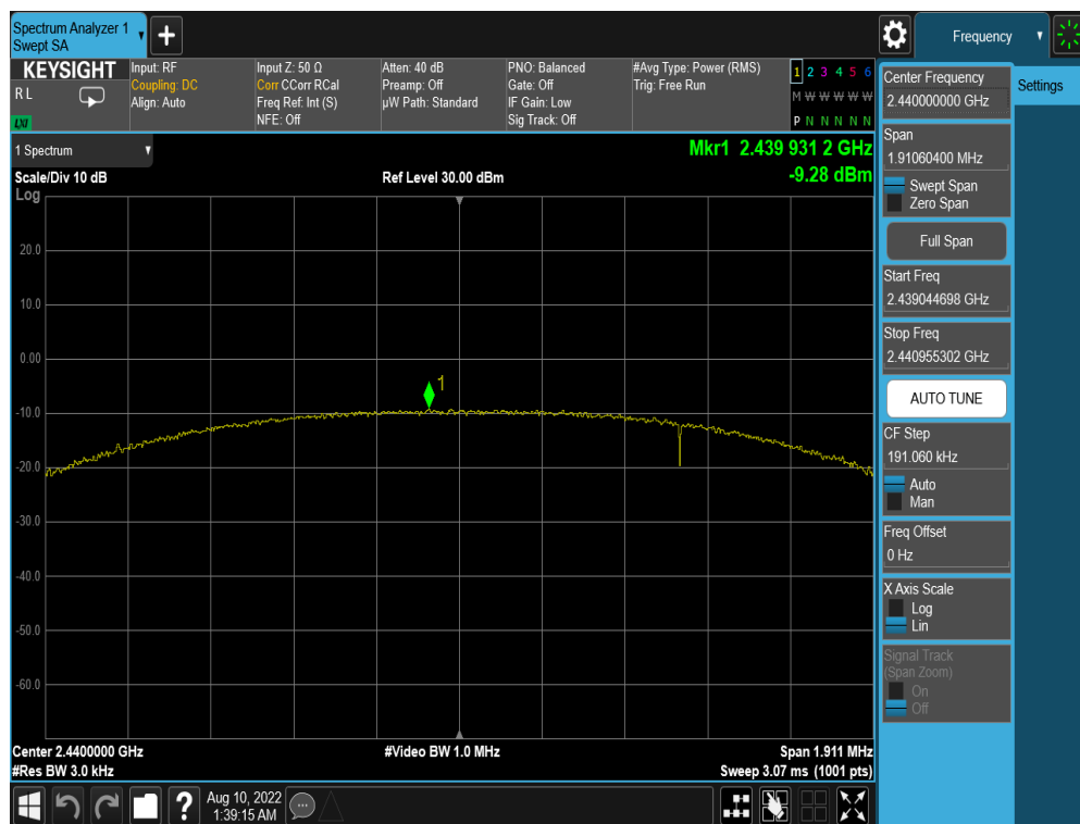
Plot 7-20. Power Spectral Density Plot Antenna 3a (Bluetooth (LE), 2Mbps, ePA – Ch. 19)
