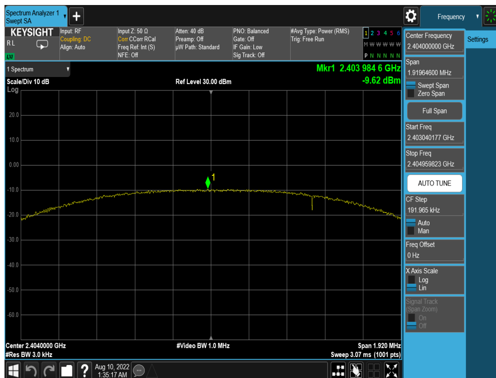
Plot 7-22. Power Spectral Density Plot Antenna 3a (Bluetooth (LE), 2Mbps, iPA – Ch. 1)
