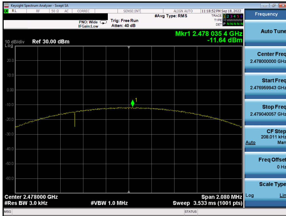
Plot 7-53. Power Spectral Density Plot Antenna 3a (Bluetooth (LE), 2Mbps, ePA – Ch. 38)
