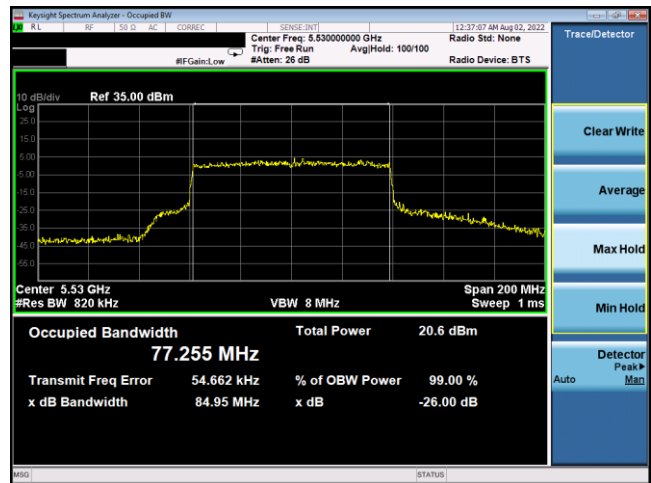
Plot 7-126. 26dB BW & 99% OBW Antenna 1b (80MHz BW 802.11ax(SU) – Ch. 106, MCS0)
