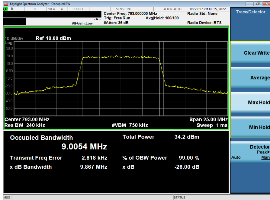
Plot 7-21. Occupied Bandwidth Plot (LTE Band 14 - 10MHz QPSK - Full RB Configuration)
