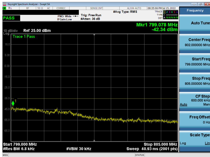
Plot 7-53. Upper Emission Mask Plot (LTE Band 14, 5MHz QPSK - RB Size 25)
