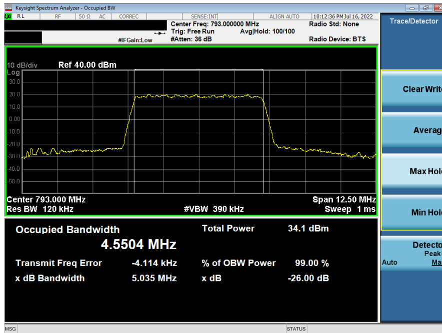
Plot 7-17. Occupied Bandwidth Plot (LTE Band 14 - 5MHz QPSK - Full RB Configuration)
