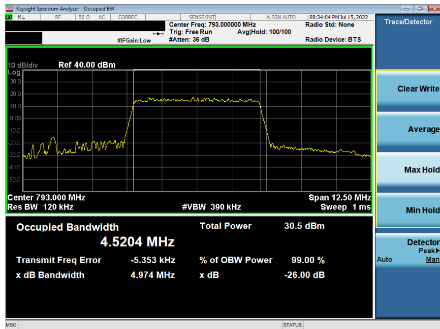
Plot 7-20. Occupied Bandwidth Plot (LTE Band 14 - 5MHz 256-QAM - Full RB Configuration)
