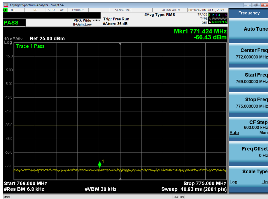
Plot 7-51. Lower Emission Mask Plot (LTE Band 14, 5MHz QPSK - RB Size 25)
