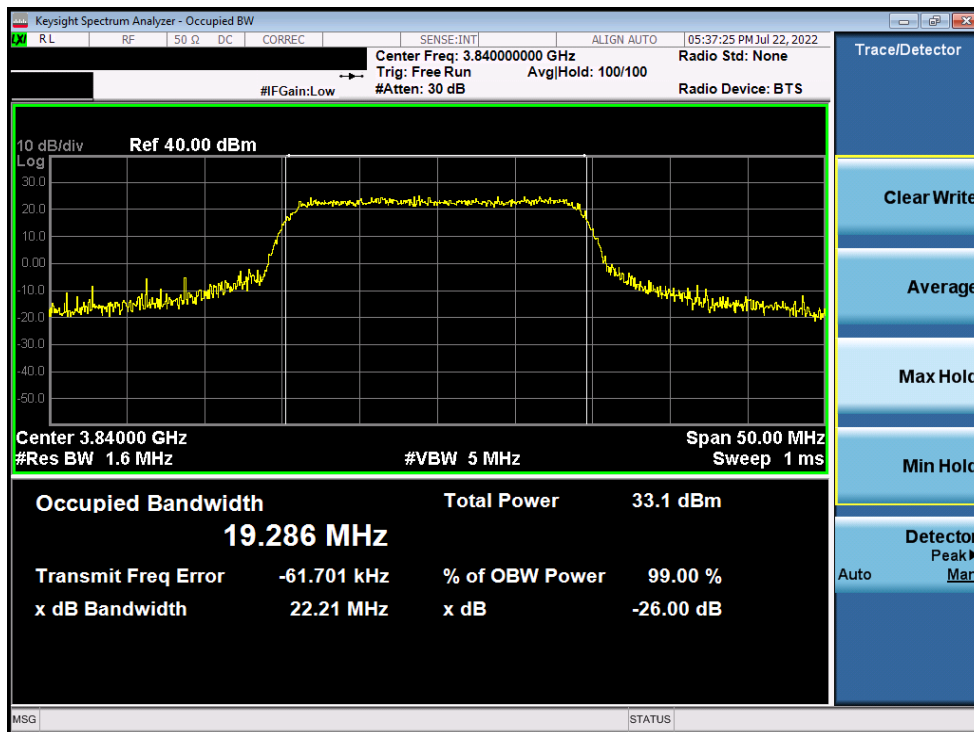
Plot 7-47. Occupied Bandwidth Plot (NR Band n77 C-Band - 20MHz CP-OFDM QPSK - Full RB)
