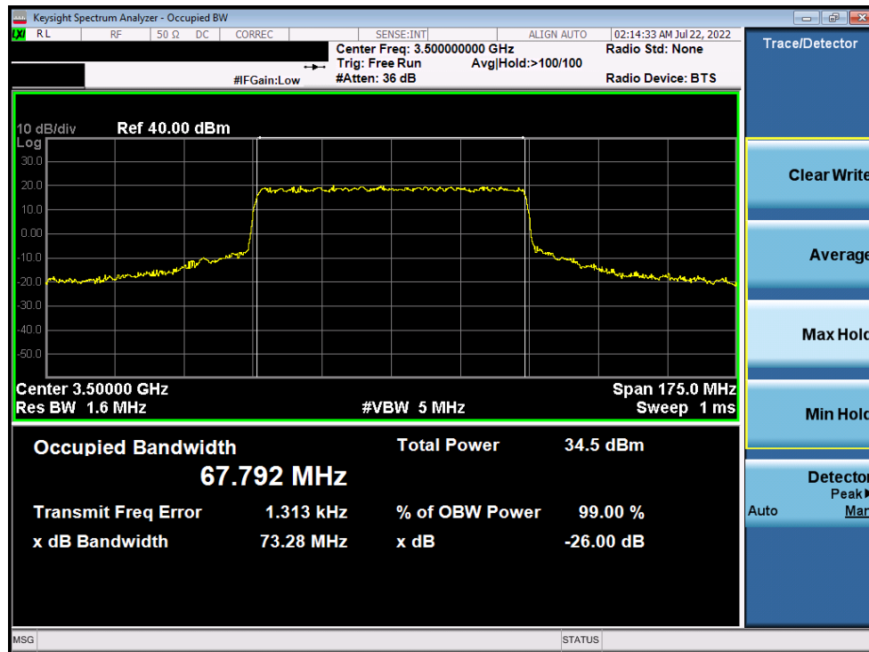
Plot 7-27. Occupied Bandwidth Plot (NR Band n77 DoD Band - 70MHz CP-OFDM QPSK - Full RB)
