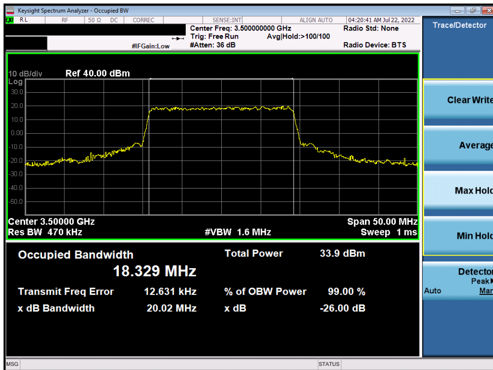
Plot 7-2. Occupied Bandwidth Plot (NR Band n77 DoD Band - 20MHz CP-OFDM QPSK - Full RB)
