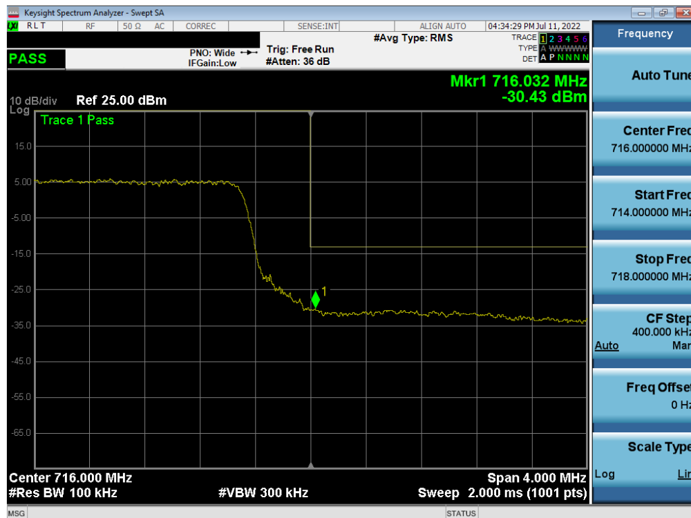
Plot 7-273. Upper Band Edge Plot (LTE Band 12 - 10MHz QPSK - Full RB)
