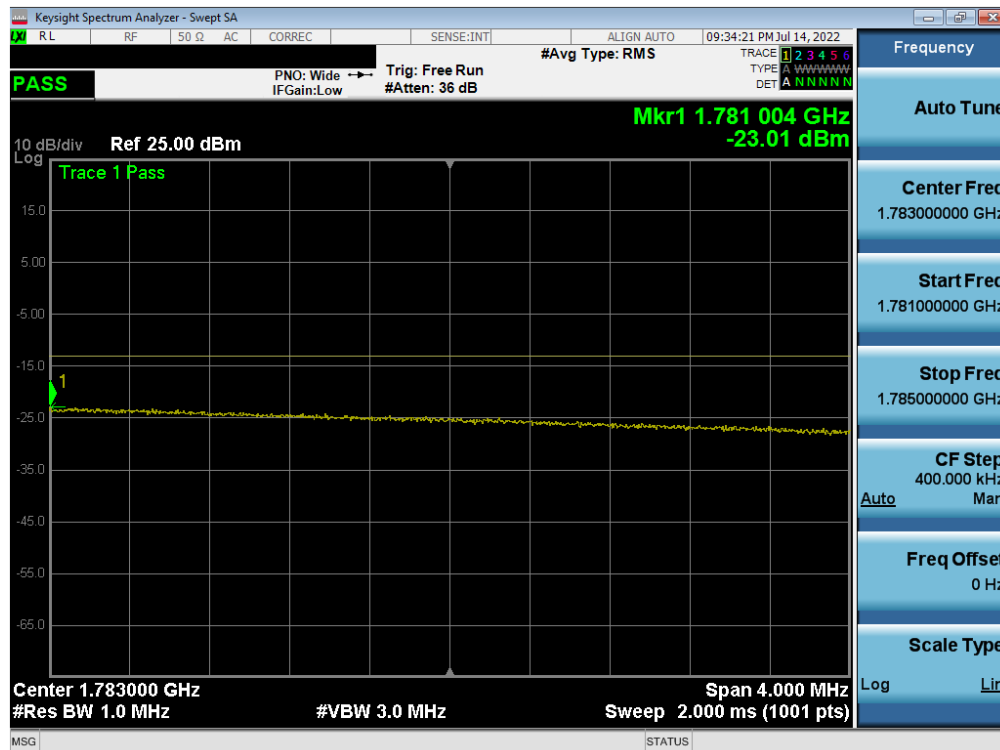
Plot 7-233. Upper Extended Band Edge Plot (LTE Band 66 - 20MHz QPSK – Full RB)
