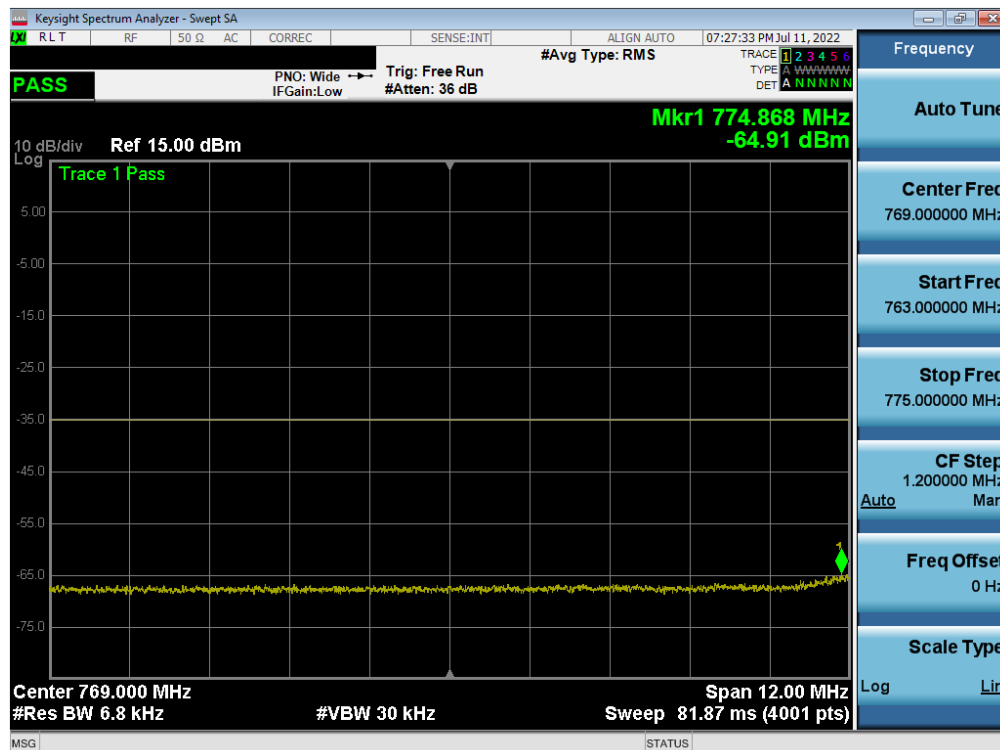
Plot 7-283. Lower Emission Mask Plot (LTE Band 13 - 10MHz QPSK – Full RB)
