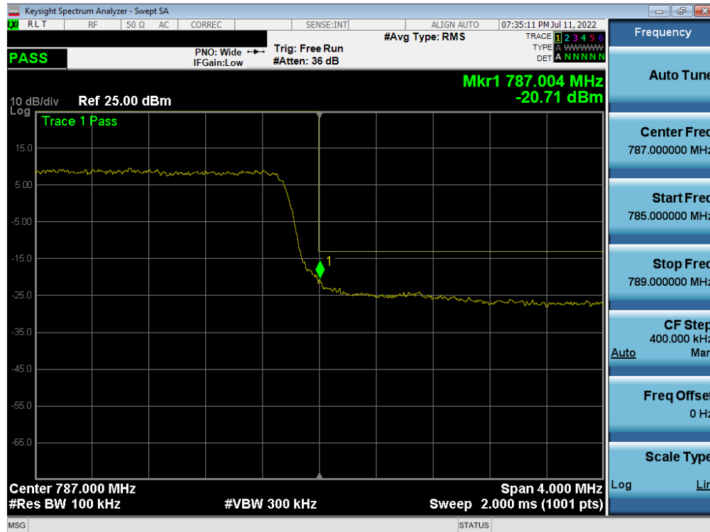
Plot 7-280. Upper Band Edge Plot (LTE Band 13 - 5MHz QPSK – Full RB)
