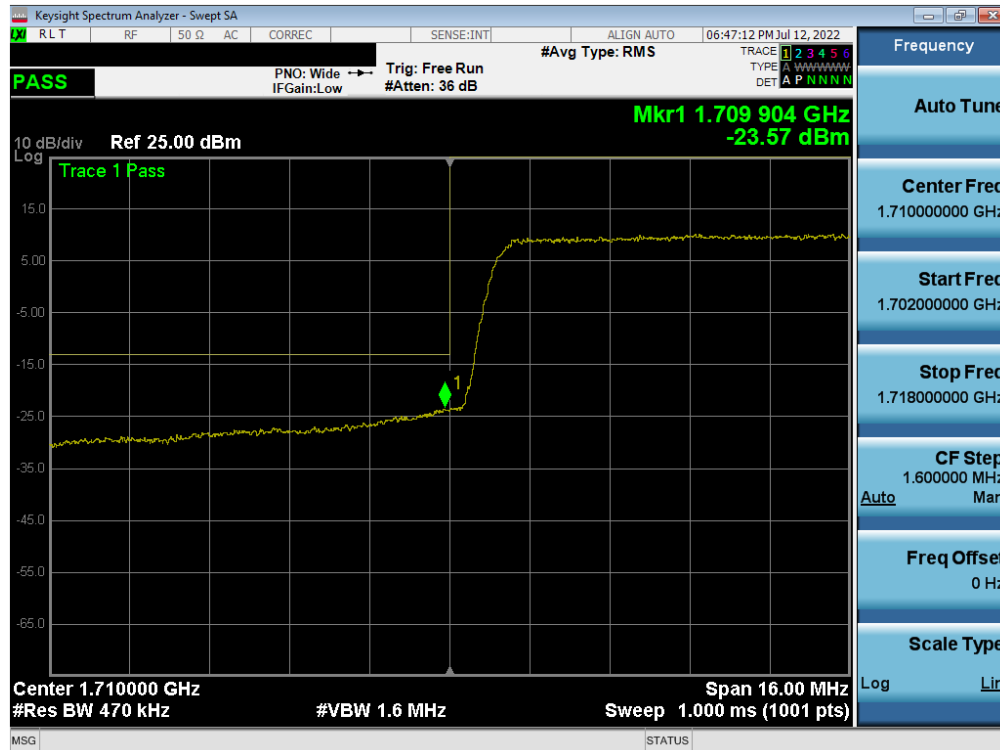
Plot 7-254. Lower Band Edge Plot (LTE Band 4 - 20MHz QPSK – Full RB)
