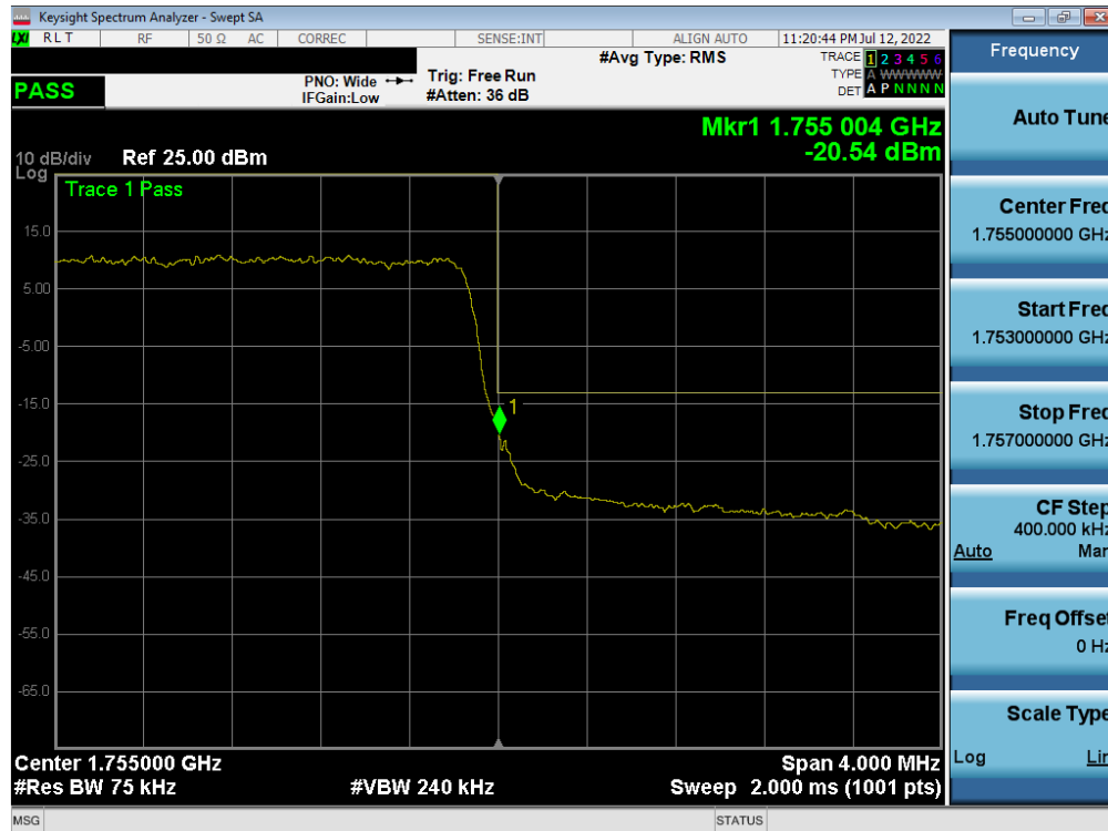
Plot 7-240. Upper Band Edge Plot (LTE Band 4 - 3MHz QPSK – Full RB)
