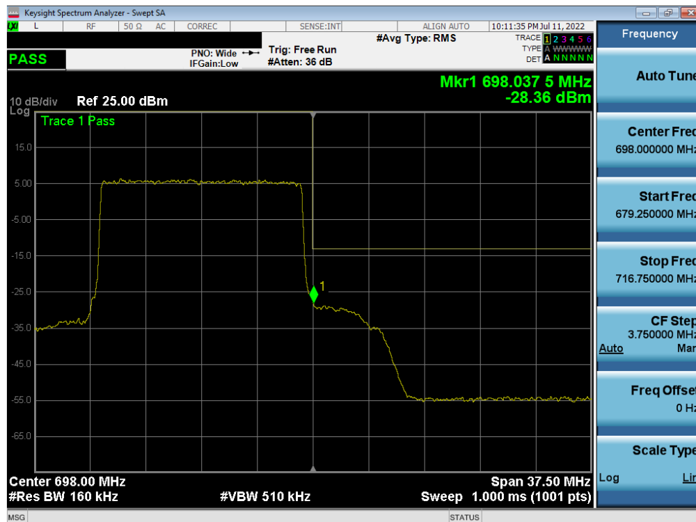
Plot 7-263. Upper Band Edge Plot (LTE Band 71 - 15MHz QPSK - Full RB)
