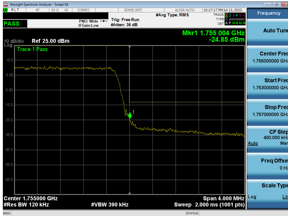
Plot 7-244. Upper Band Edge Plot (LTE Band 4 - 5MHz QPSK – Full RB)
