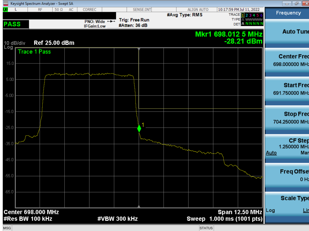
Plot 7-259. Upper Band Edge Plot (LTE Band 71 - 5MHz QPSK – Full RB)
