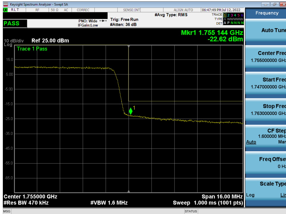
Plot 7-256. Upper Band Edge Plot (LTE Band 4 - 20MHz QPSK - Full RB)
