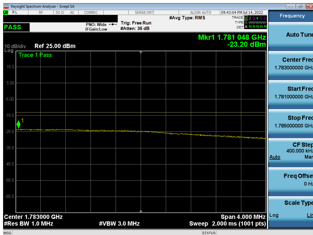
Plot 7-229. Upper Extended Band Edge Plot (LTE Band 66 - 15MHz QPSK – Full RB)
