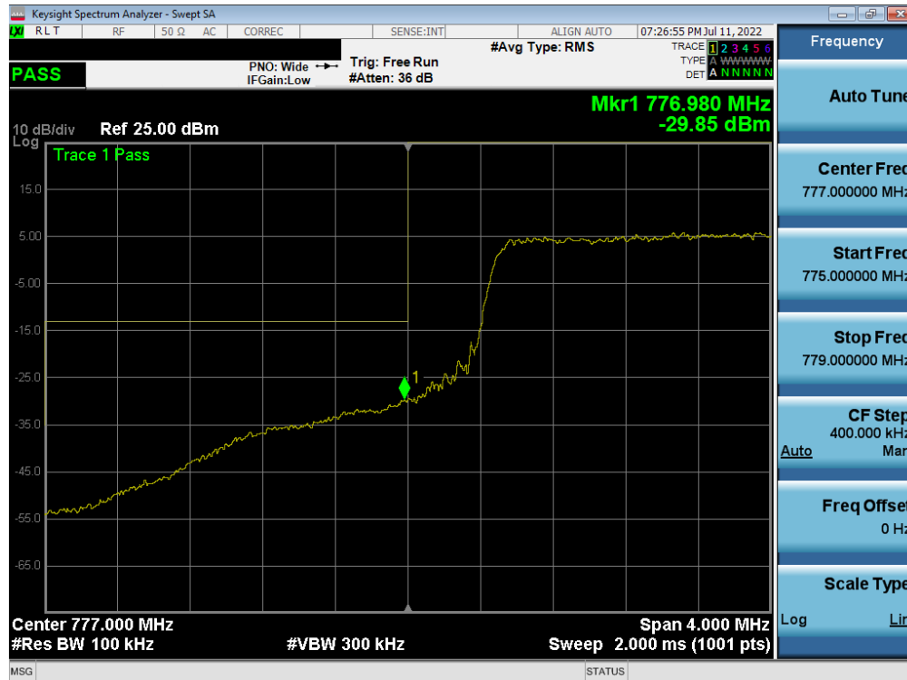
Plot 7-282. Lower Band Edge Plot (LTE Band 13 - 10MHz QPSK – Full RB)
