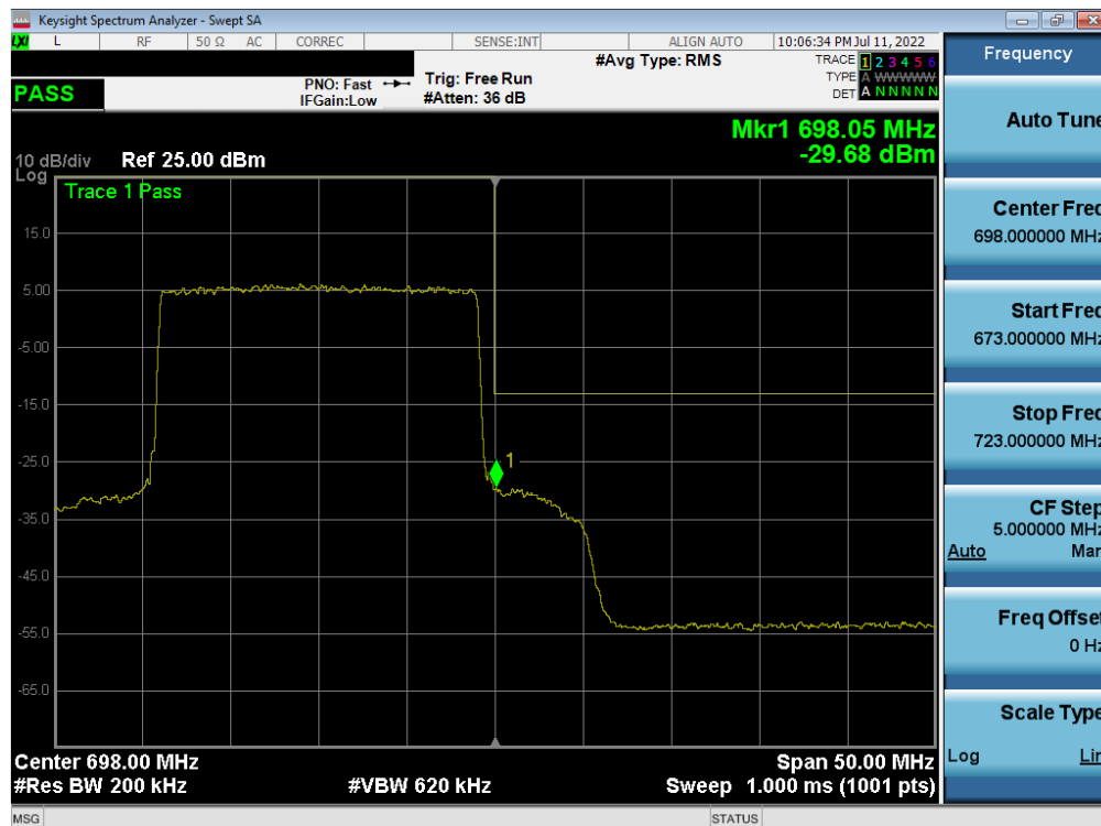
Plot 7-265. Upper Band Edge Plot (LTE Band 71 - 20MHz QPSK - Full RB)
