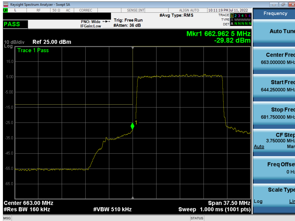
Plot 7-262. Lower Band Edge Plot (LTE Band 71 - 15MHz QPSK - Full RB)
