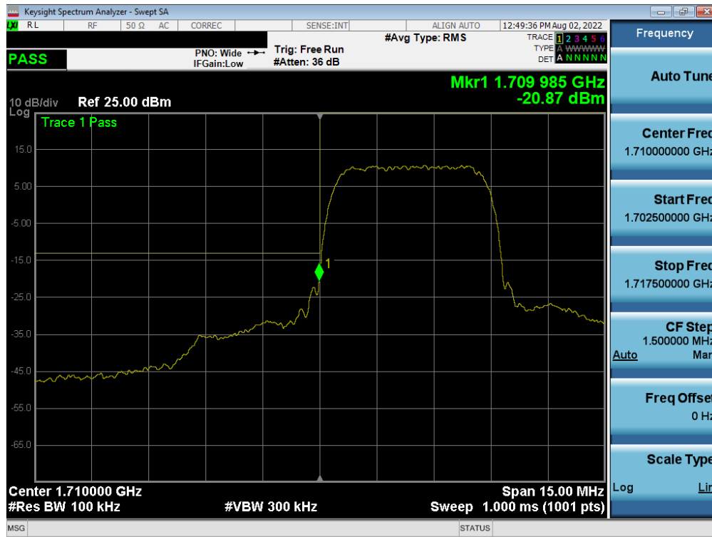
Plot 7-328. Lower Band Edge Plot (WCDMA AWS – Ch. 1312)
