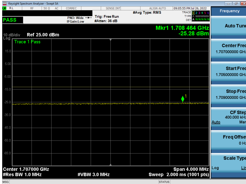
Plot 7-325. Lower Extended Band Edge Plot (ULCA LTE Band 66 – (20+20)MHz QPSK – Low Channel)
