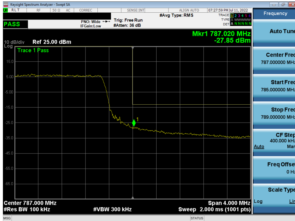
Plot 7-284. Upper Band Edge Plot (LTE Band 13 - 10MHz QPSK - Full RB)
