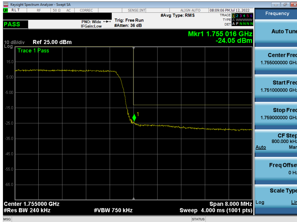
Plot 7-248. Upper Band Edge Plot (LTE Band 4 - 10MHz QPSK – Full RB)
