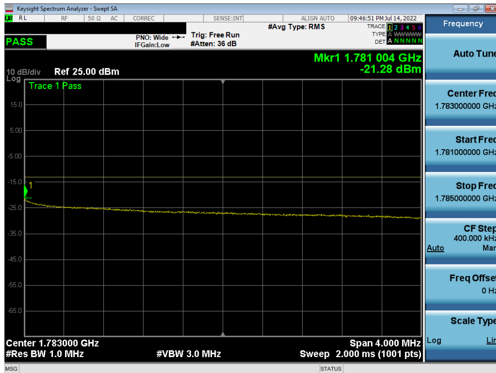
Plot 7-225. Upper Extended Band Edge Plot (LTE Band 66 - 10MHz QPSK – Full RB)
