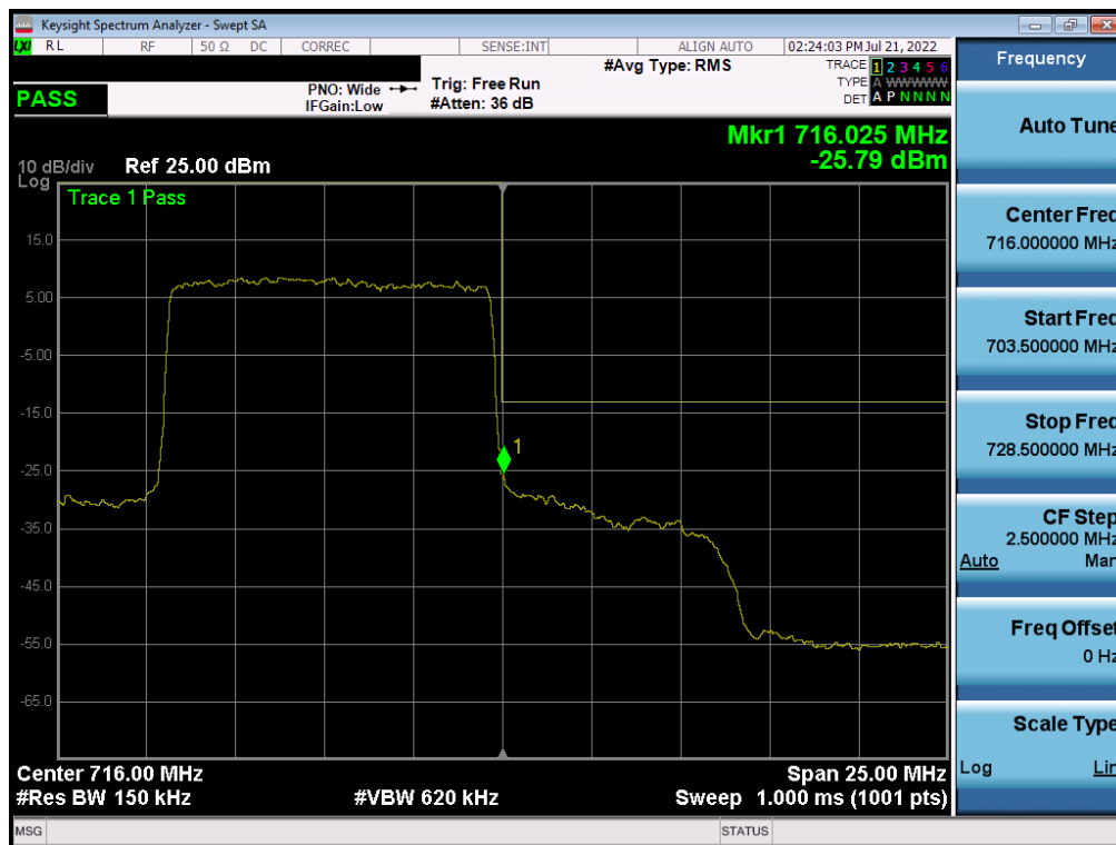
Plot 7-321. Upper Band Edge Plot (NR Band n12 – 10.0MHz DFTs-OFDM QPSK - Full RB)
