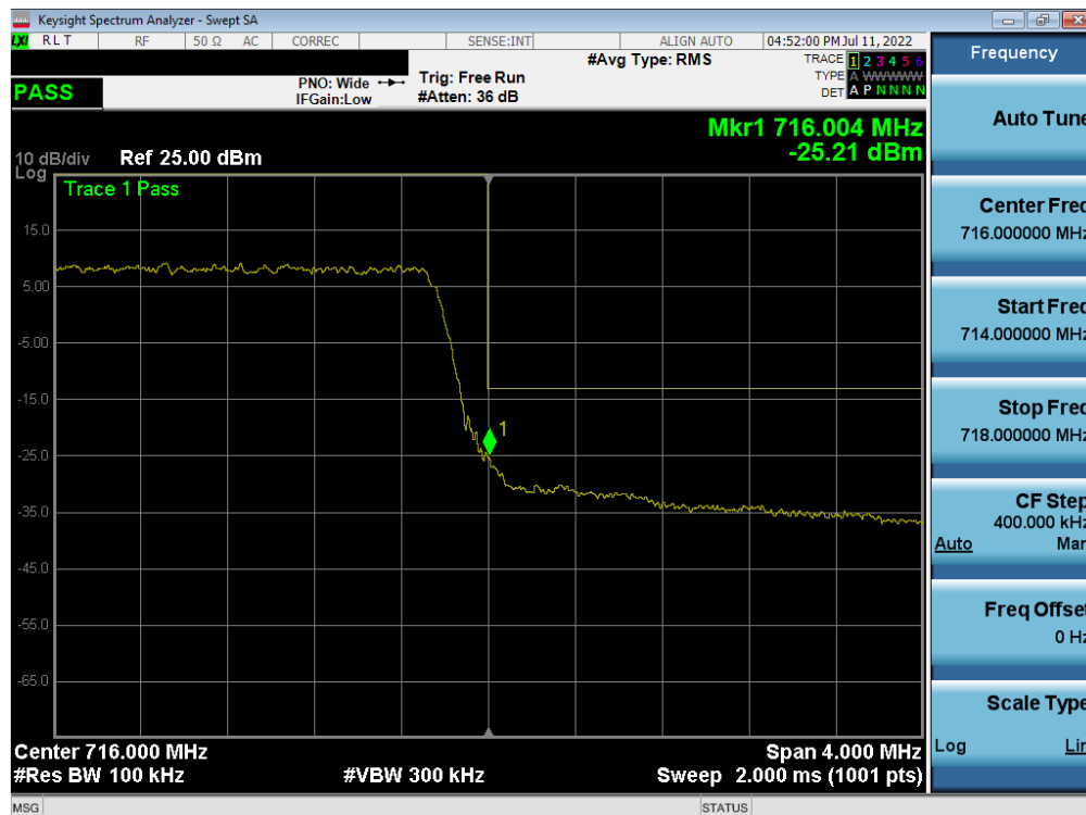
Plot 7-271. Upper Band Edge Plot (LTE Band 12 - 5MHz QPSK – Full RB)
