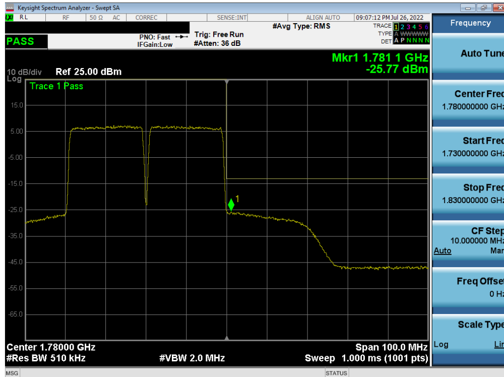
Plot 7-326. Upper Band Edge Plot (ULCA LTE Band 66 – (20+20)MHz QPSK – High Channel)
