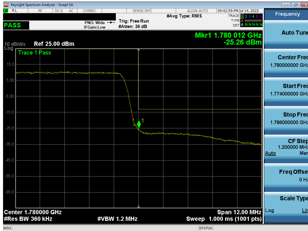
Plot 7-228. Upper Band Edge Plot (LTE Band 66 - 15MHz QPSK – Full RB)
