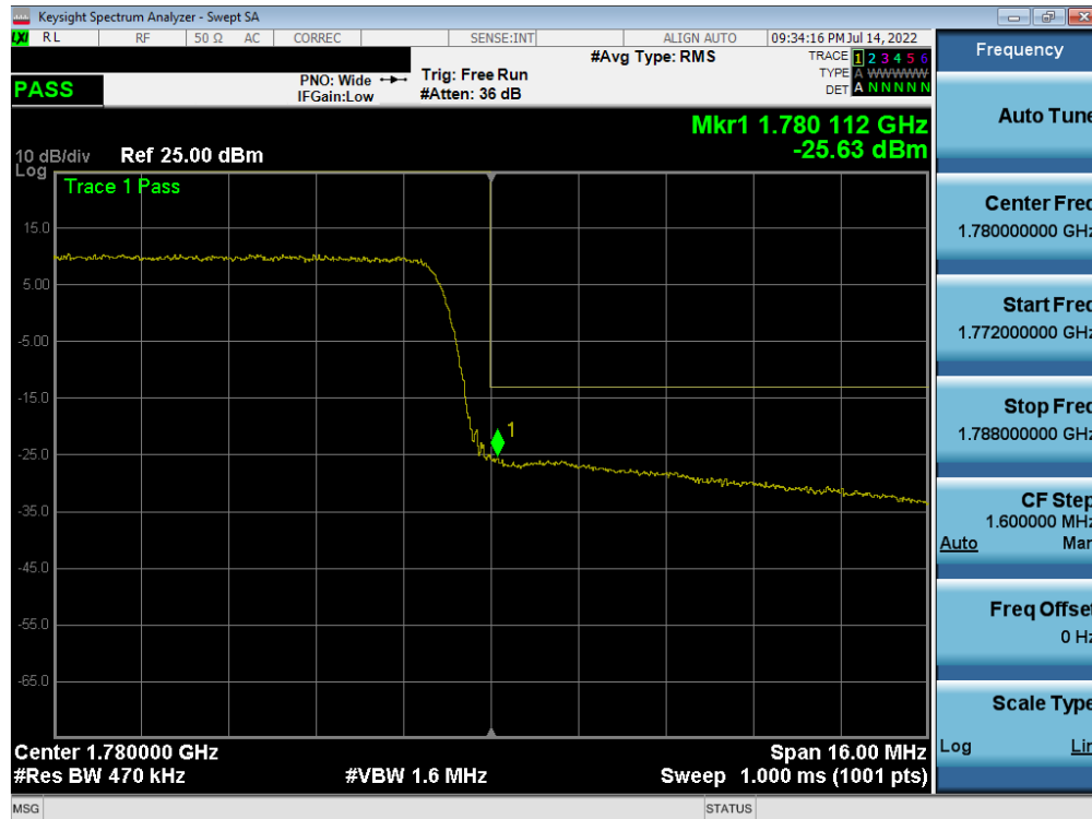
Plot 7-232. Upper Band Edge Plot (LTE Band 66 - 20MHz QPSK – Full RB)
