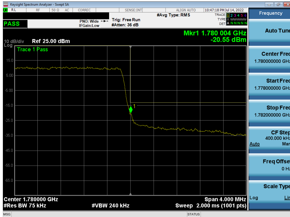
Plot 7-216. Upper Band Edge Plot (LTE Band 66 - 3MHz QPSK – Full RB)
