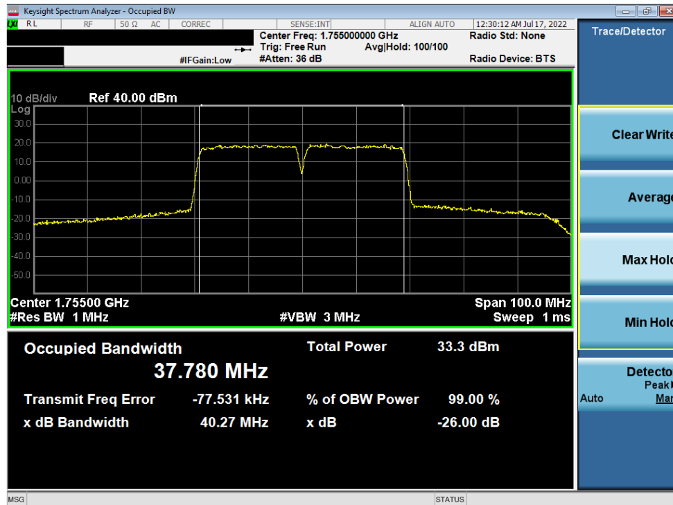
Plot 7-131. Occupied Bandwidth Plot (ULCA Band 66 – (20+20)MHz 16-QAM - Full RB)
