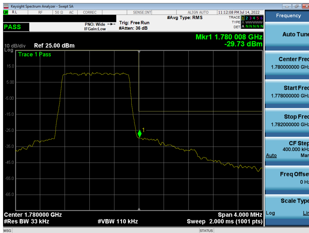
Plot 7-212. Upper Band Edge Plot (LTE Band 66 – 1.4MHz QPSK – Full RB)
