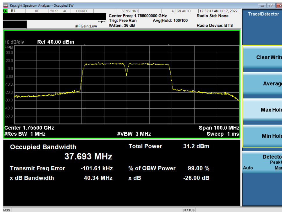
Plot 7-133. Occupied Bandwidth Plot (ULCA Band 66 – (20+20)MHz 256-QAM - Full RB)
