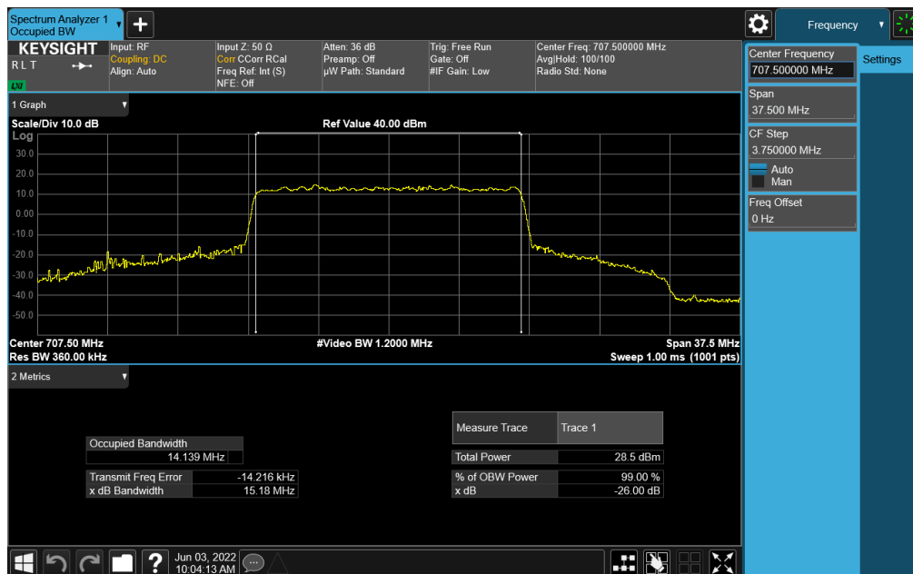
Plot 7-129. Occupied Bandwidth Plot (NR Band n12 - 15MHz CP-OFDM 256-QAM - Full RB)
