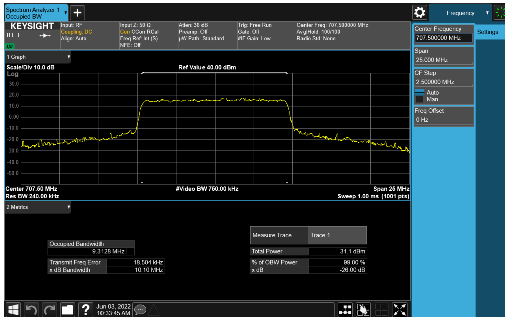
Plot 7-123. Occupied Bandwidth Plot (NR Band n12 - 10MHz CP-OFDM 64-QAM - Full RB)
