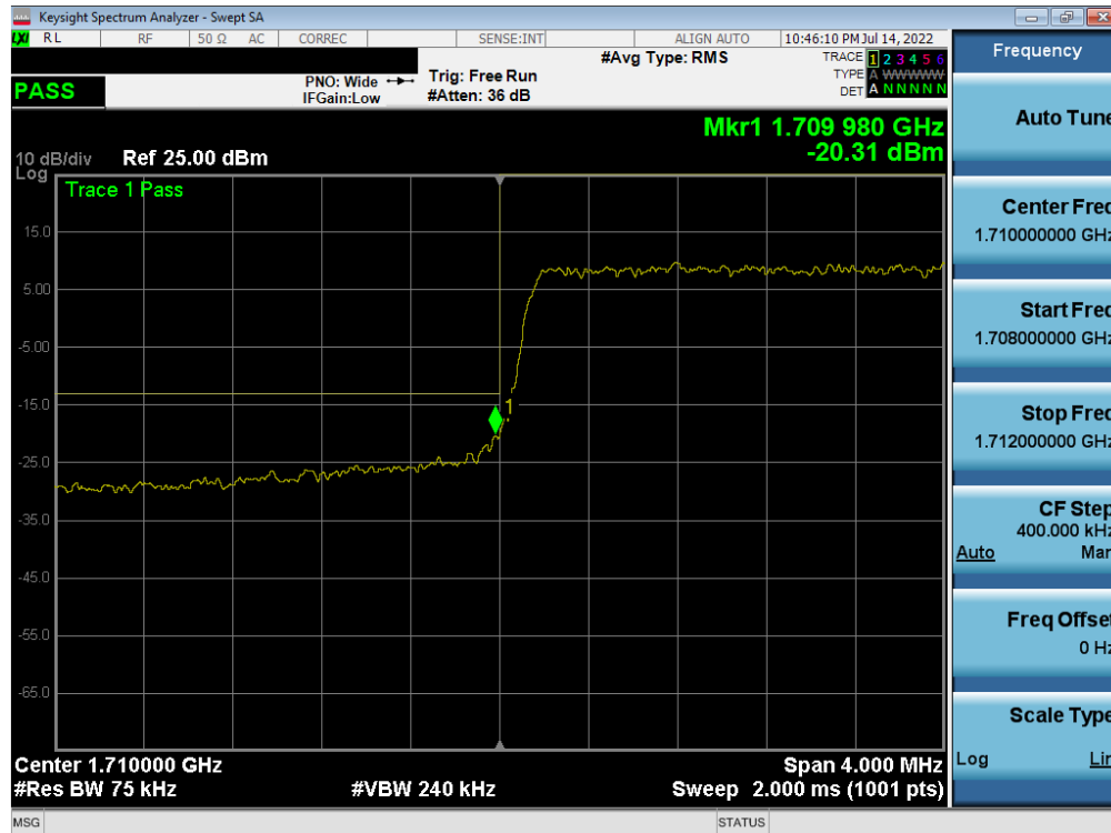
Plot 7-214. Lower Band Edge Plot (LTE Band 66 - 3MHz QPSK – Full RB)
