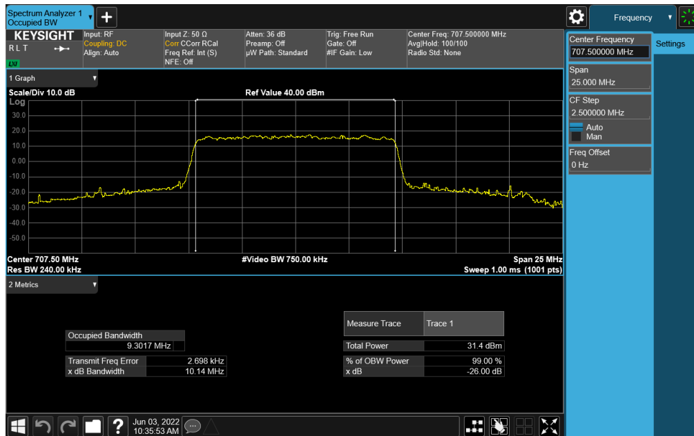
Plot 7-121. Occupied Bandwidth Plot (NR Band n12 - 10MHz CP-OFDM QPSK - Full RB)
