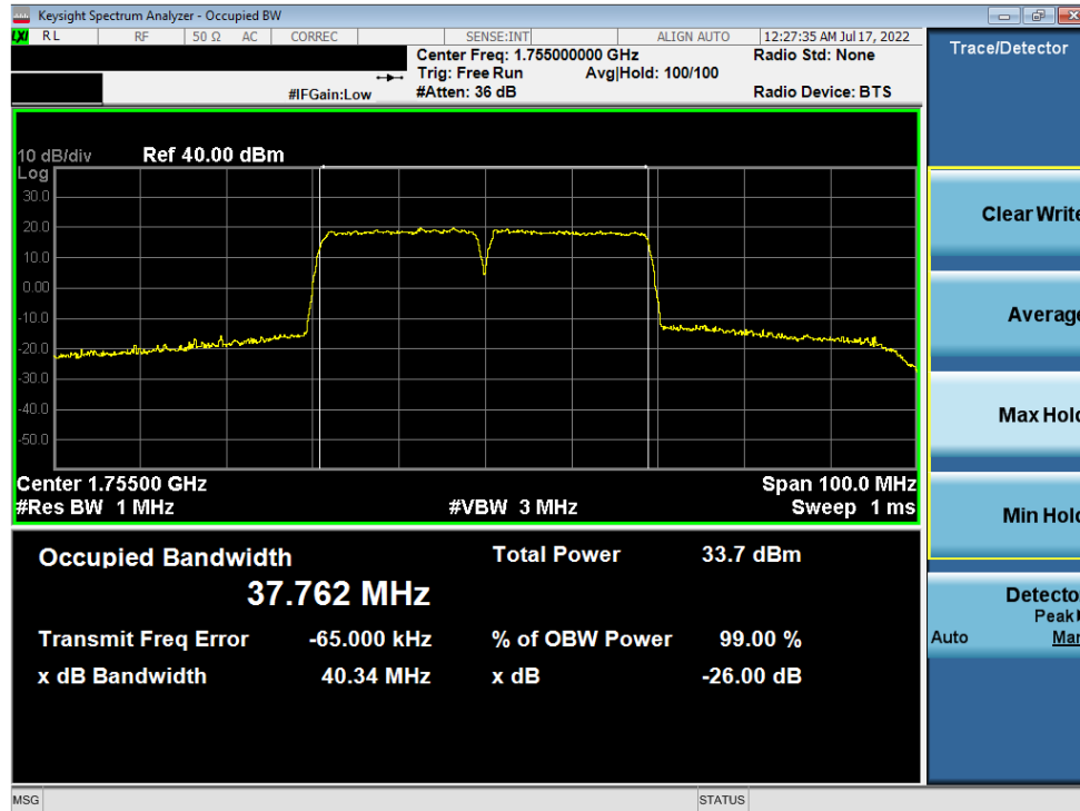
Plot 7-130. Occupied Bandwidth Plot (ULCA Band 66 – (20+20)MHz QPSK - Full RB)
