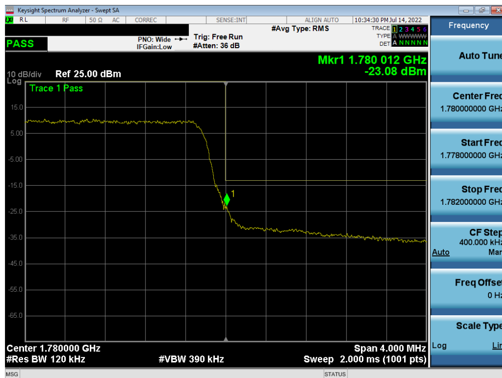
Plot 7-220. Upper Band Edge Plot (LTE Band 66 - 5MHz QPSK – Full RB)
