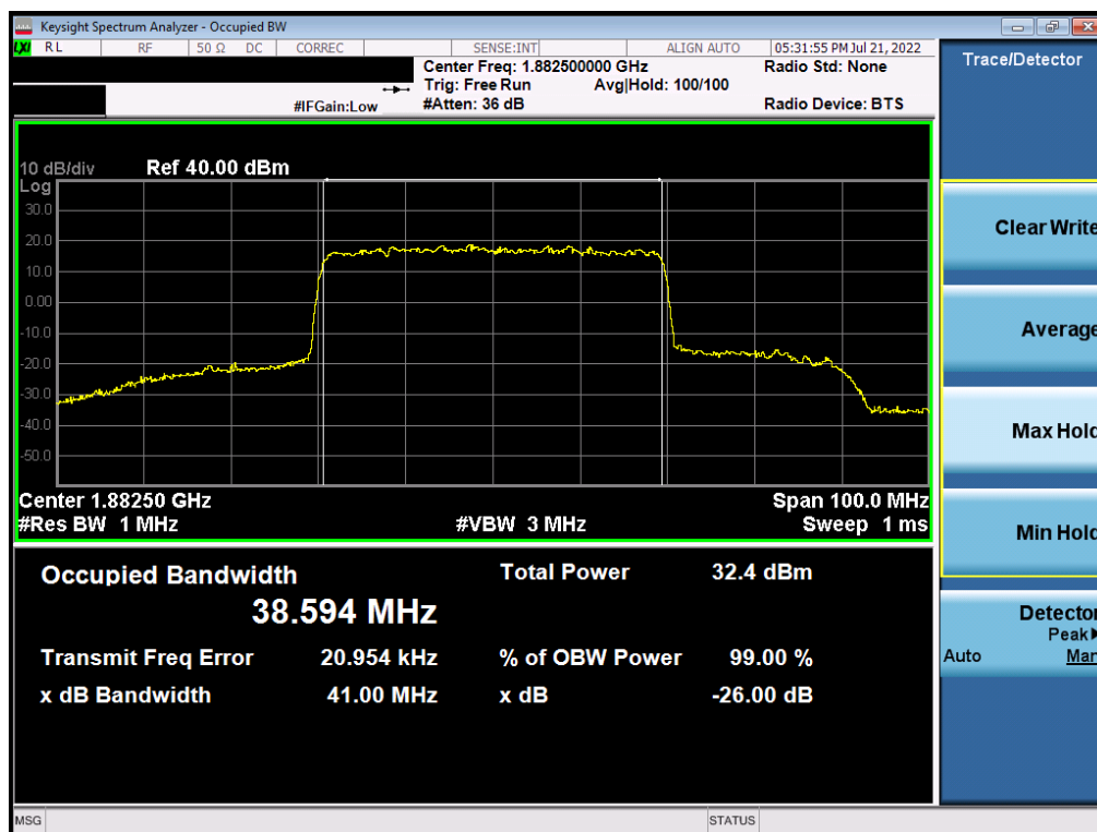
Plot 7-59. Occupied Bandwidth Plot (NR Band n25 - 40.0MHz CP-OFDM 256QAM - Full RB)
