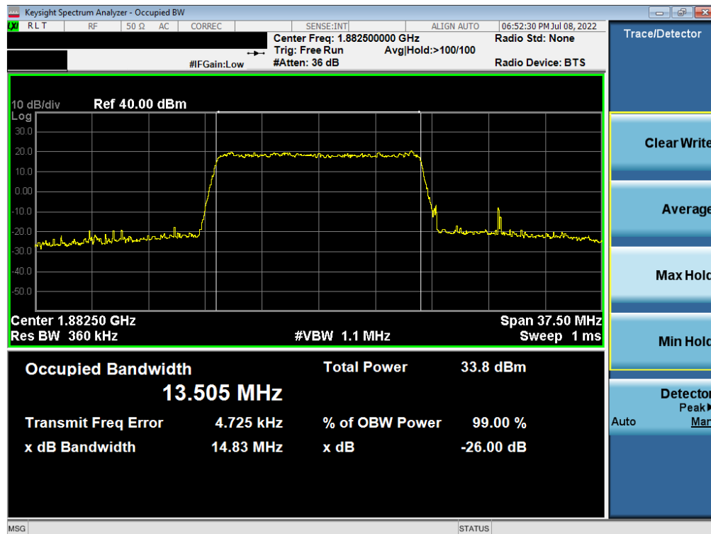
Plot 7-18. Occupied Bandwidth Plot (LTE Band 25/2 - 15MHz 16-QAM - Full RB Configuration)
