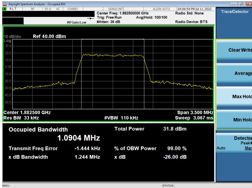
Plot 7-3. Occupied Bandwidth Plot (LTE Band 25/2 - 1.4MHz 64-QAM - Full RB Configuration)
