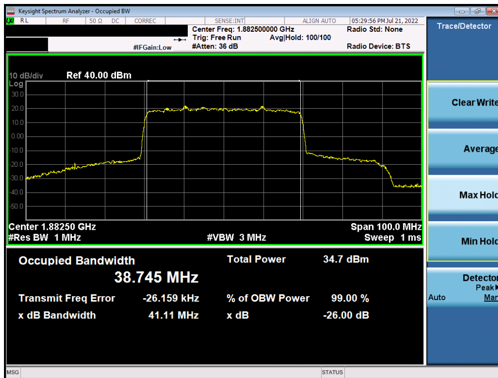
Plot 7-56. Occupied Bandwidth Plot (NR Band n25 - 40.0MHz CP-OFDM QPSK - Full RB)
