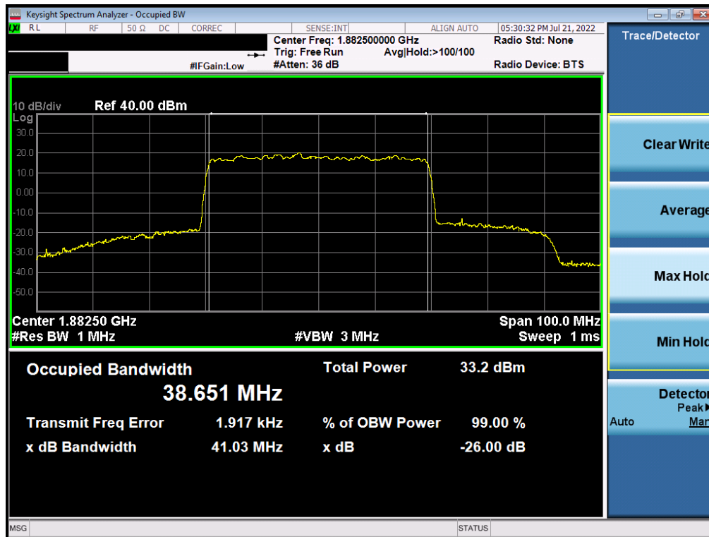
Plot 7-57. Occupied Bandwidth Plot (NR Band n25 - 40.0MHz CP-OFDM 16QAM - Full RB)
