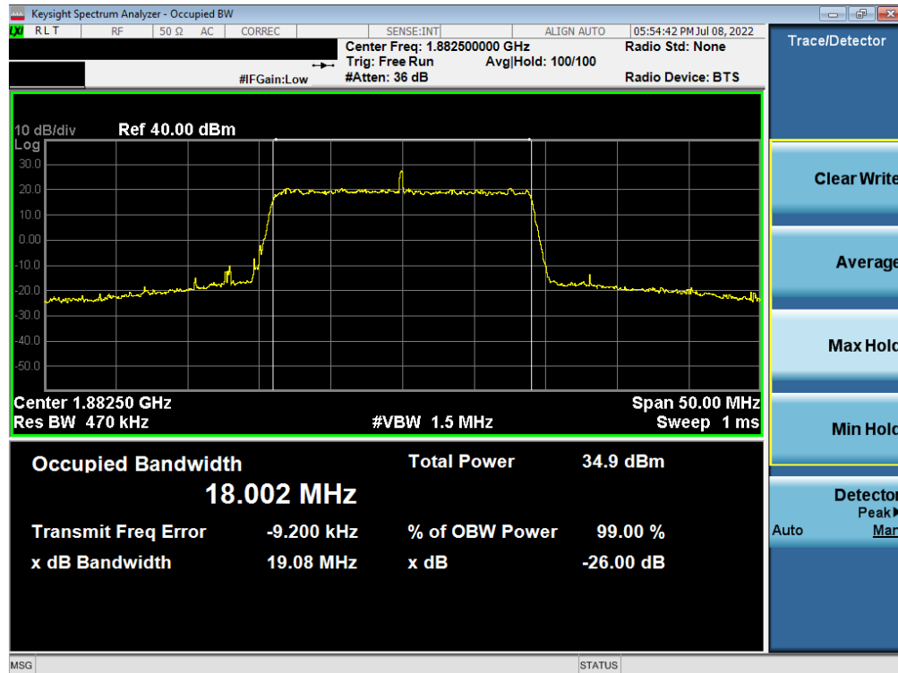
Plot 7-21. Occupied Bandwidth Plot (LTE Band 25/2 - 20MHz QPSK - Full RB Configuration)
