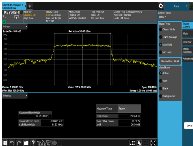
Plot 7-44. 26dB BW & 99% OBW Antenna WF7a (40MHz BW 11ax – RU484 – Ch.46)
