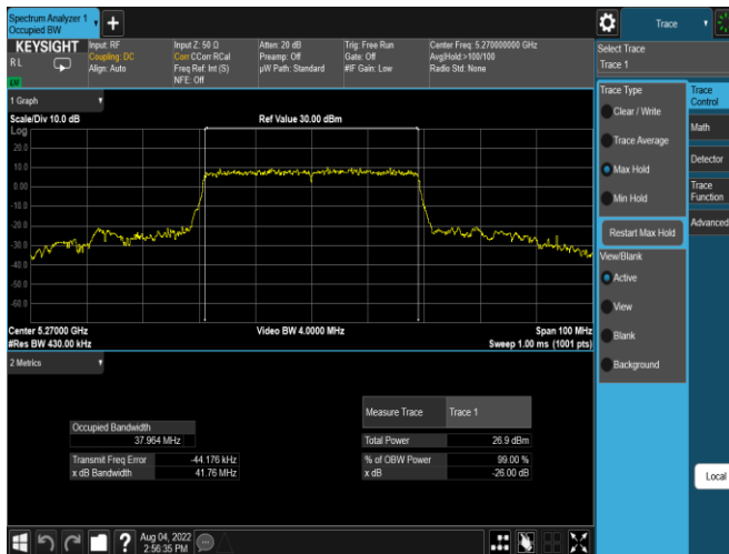
Plot 7-20. 26dB BW & 99% OBW Antenna WF8 (40MHz BW 11ax - RU484 - Ch.54)
