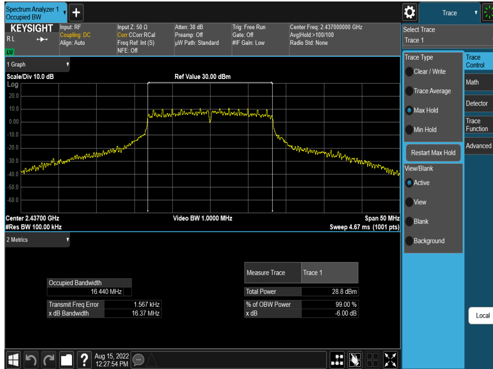
Plot 7-23. 6dB BW and 99% OBW Plot Antenna WF8 (802.11g – Ch. 6) – 36Mbps
