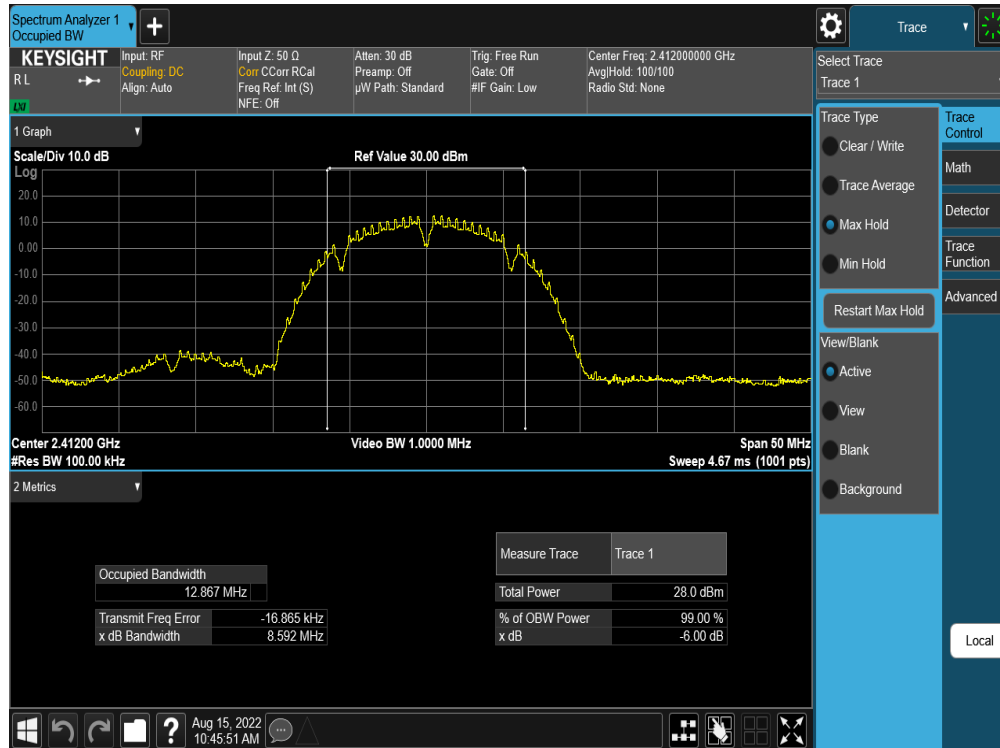
Plot 7-19. 6dB BW and 99% OBW Plot Antenna WF8 (802.11b – Ch. 1) – 11Mbps
