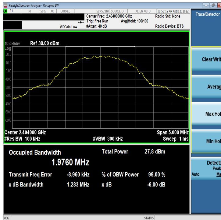
Plot 7-4. 6dB BW & 99% OBW Plot Antenna WF8 (Bluetooth (LE), 2Mbps, ePA – Ch. 1)
