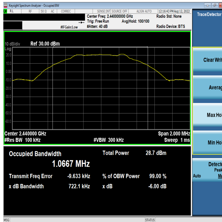
Plot 7-8. 6dB BW & 99% OBW Plot Antenna WF7b (Bluetooth (LE), 1Mbps, ePA – Ch. 19)
