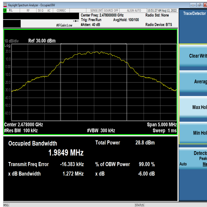
Plot 7-6. 6dB BW & 99% OBW Plot Antenna WF8 (Bluetooth (LE), 2Mbps, ePA – Ch. 38)
