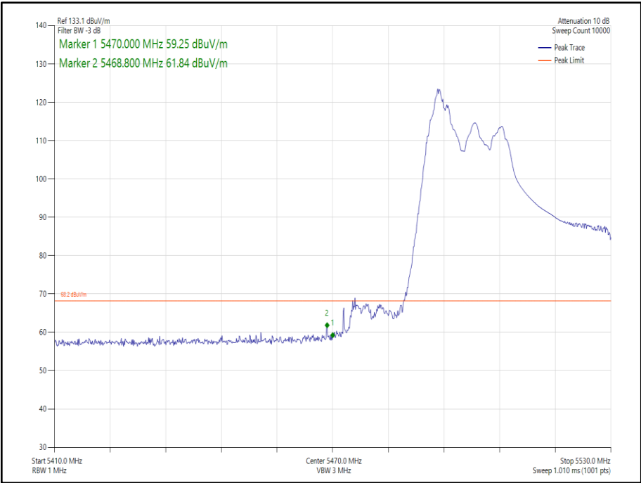
Figure 228 - 802.11ax HE40 CDD, Cores 0-1, RU37 - 5510 MHz Band Edge Frequency 5470 MHz
