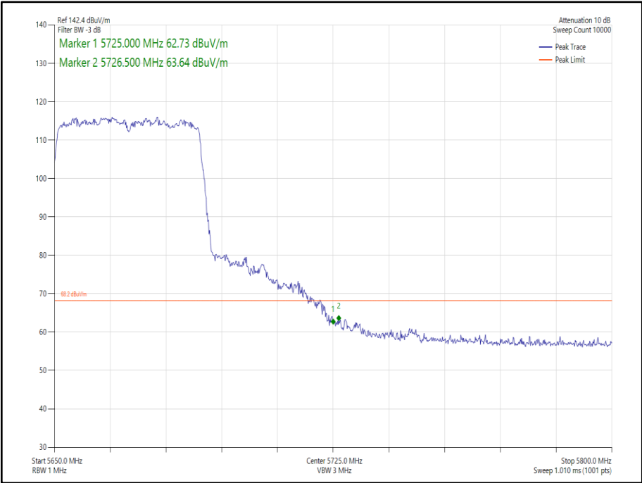
Figure 235 - 802.11ax HE40 SDM, Cores 0-1, SU - 5670 MHz Band Edge Frequency 5725 MHz
