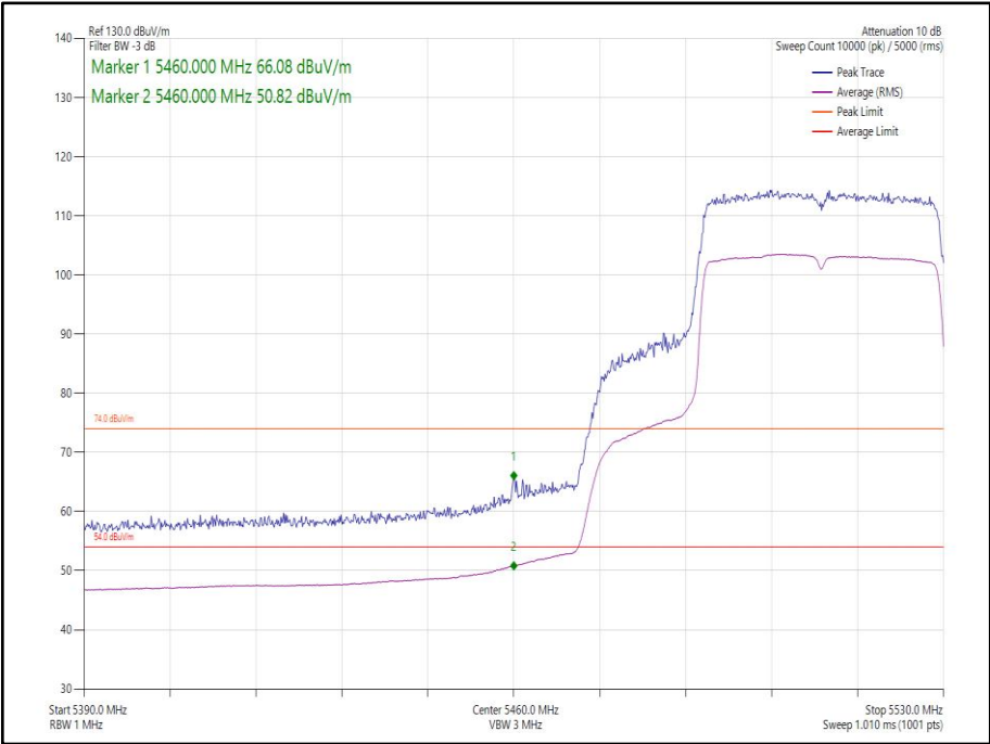
Figure 38 - 802.11ax HE40, Core 1, SU - 5510 MHz Band Edge Frequency 5460 MHz
