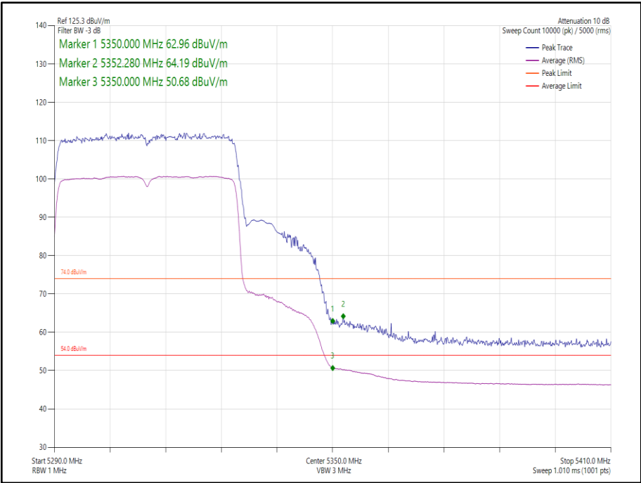
Figure 35 - 802.11ax HE40, Core 1, SU - 5310 MHz Band Edge Frequency 5350 MHz
