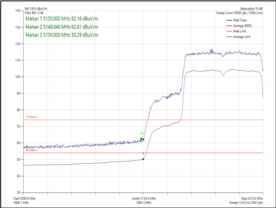
Figure 44 802.11ax HE40 SDM, Cores 0-1, SU - 5190 MHz Band Edge Frequency 5150 MHz
