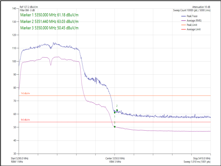
Figure 34 - 802.11n HT40, Core 1 - 5310 MHz Band Edge Frequency 5350 MHz
