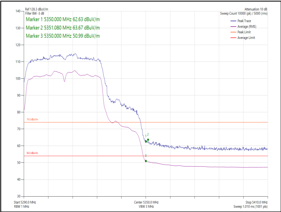
Figure 47 - 802.11n HT40 SDM, Cores 0-1 - 5310 MHz Band Edge Frequency 5350 MHz
