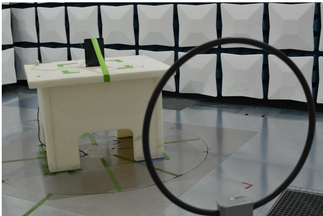
Figure 25: 9kHz-30MHz Test Setup (Front View)
