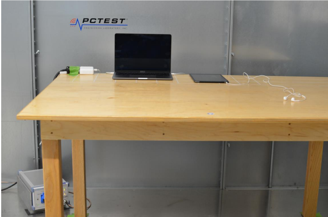
Figure 3: AC Line Conducted Emissions (Front View)
