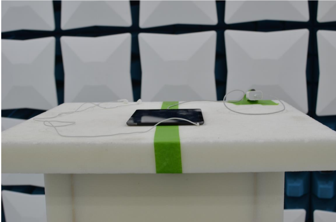
Figure 5: 1-18GHz Test Setup (Front View)
