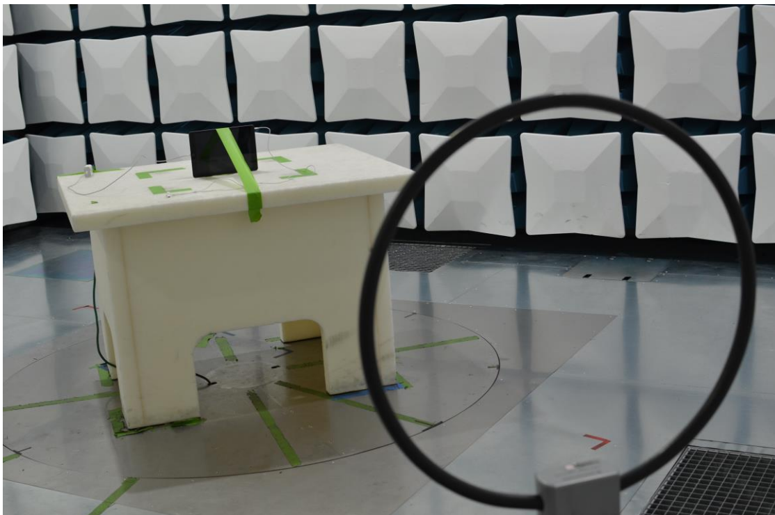
Figure 24: 9kHz-30MHz Test Setup (Front View)
