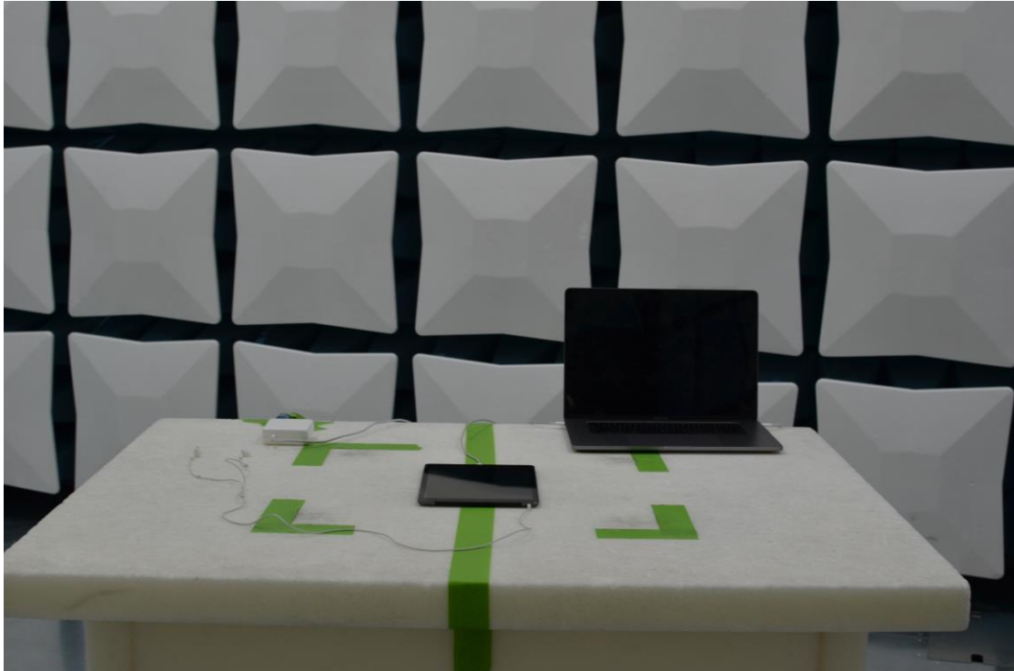
Figure 17: 30MHz-1GHz Test Setup (Front View)
