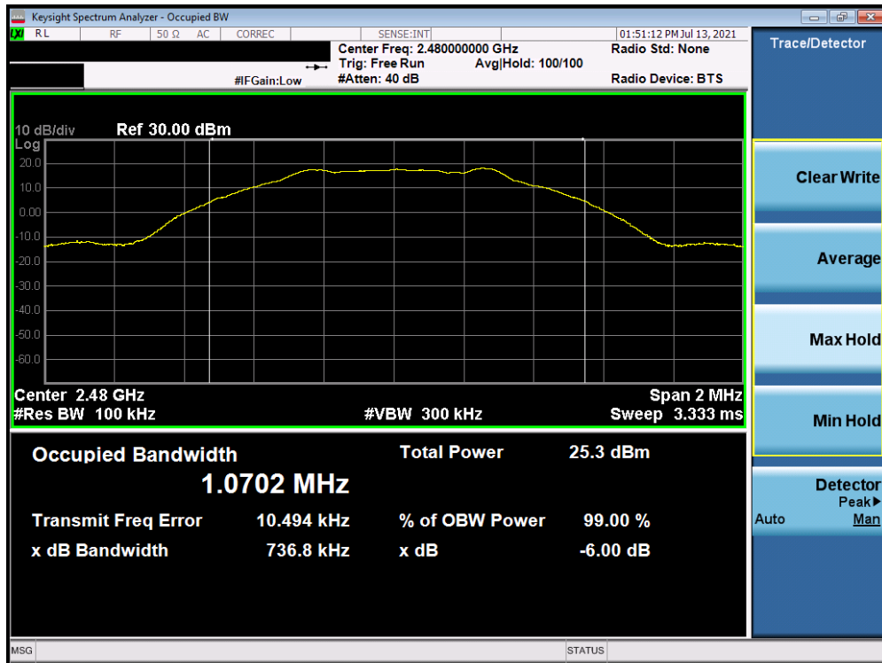
Plot 7-3. 6dB BW & 99% OBW Plot Antenna A (Bluetooth (LE), 1Mbps, ePA – Ch. 39)
