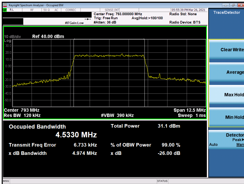
Plot 7-15. Occupied Bandwidth Plot (Band 14 - 5MHz 64-QAM - Full RB Configuration)
