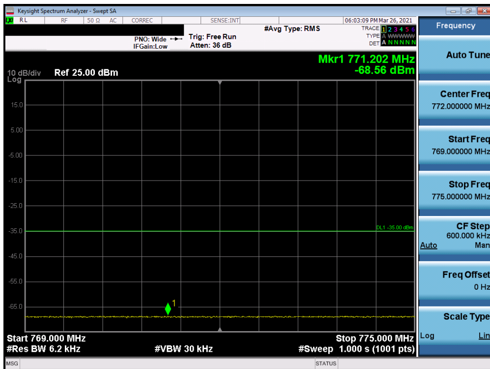
Plot 7-45. Lower Emission Mask Plot (LTE Band 14 - 5MHz QPSK)
