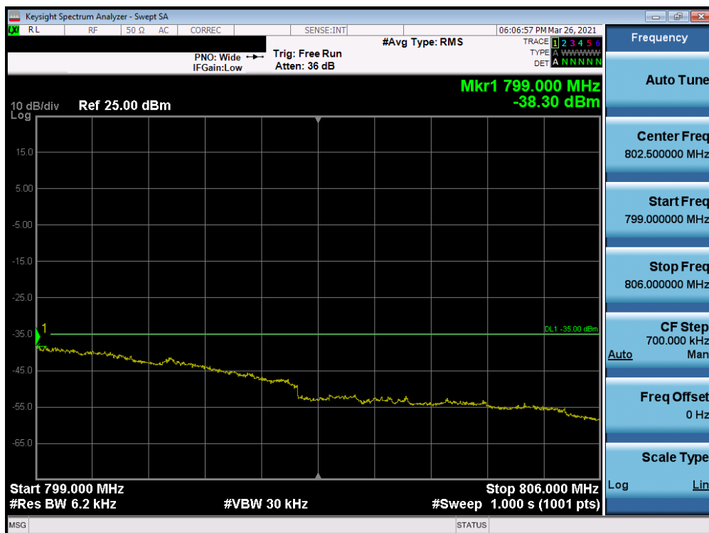
Plot 7-47. Upper Emission Mask Plot (LTE Band 14 - 5MHz QPSK)
