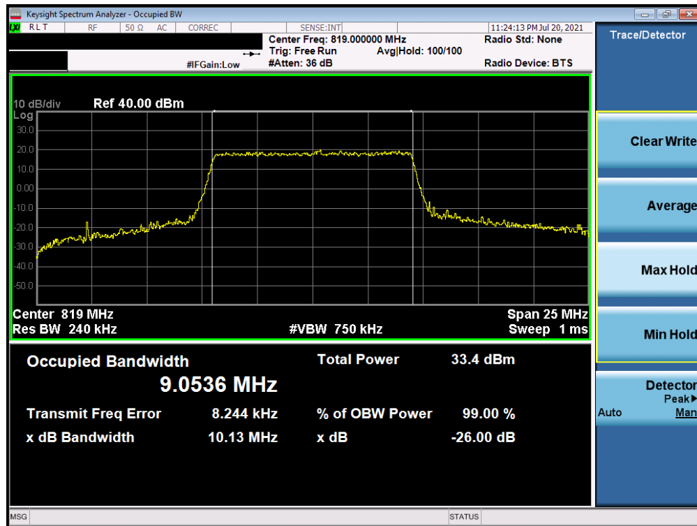
Plot 7-11. Occupied Bandwidth Plot (LTE Band 26 - 10MHz 16-QAM - Full RB Configuration)
