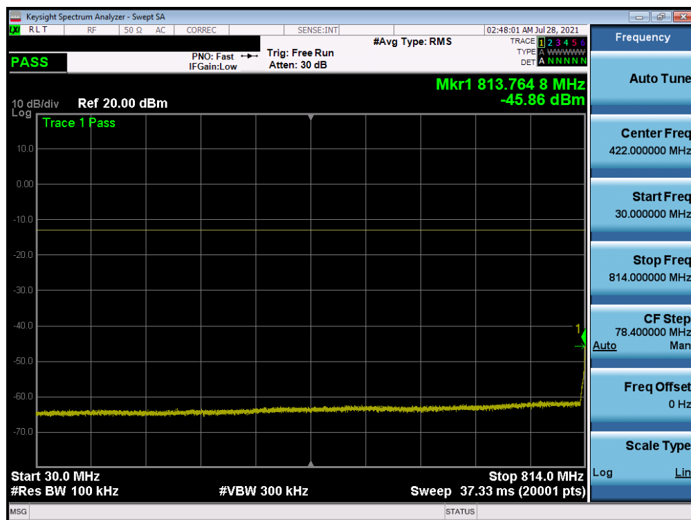
Plot 7-22. Conducted Spurious Plot (LTE Band 26 - 10MHz QPSK - RB Size 1, RB Offset 0 – Mid Channel)
