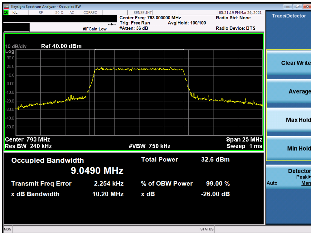
Plot 7-17. Occupied Bandwidth Plot (Band 14 - 10MHz 16-QAM - Full RB Configuration)
