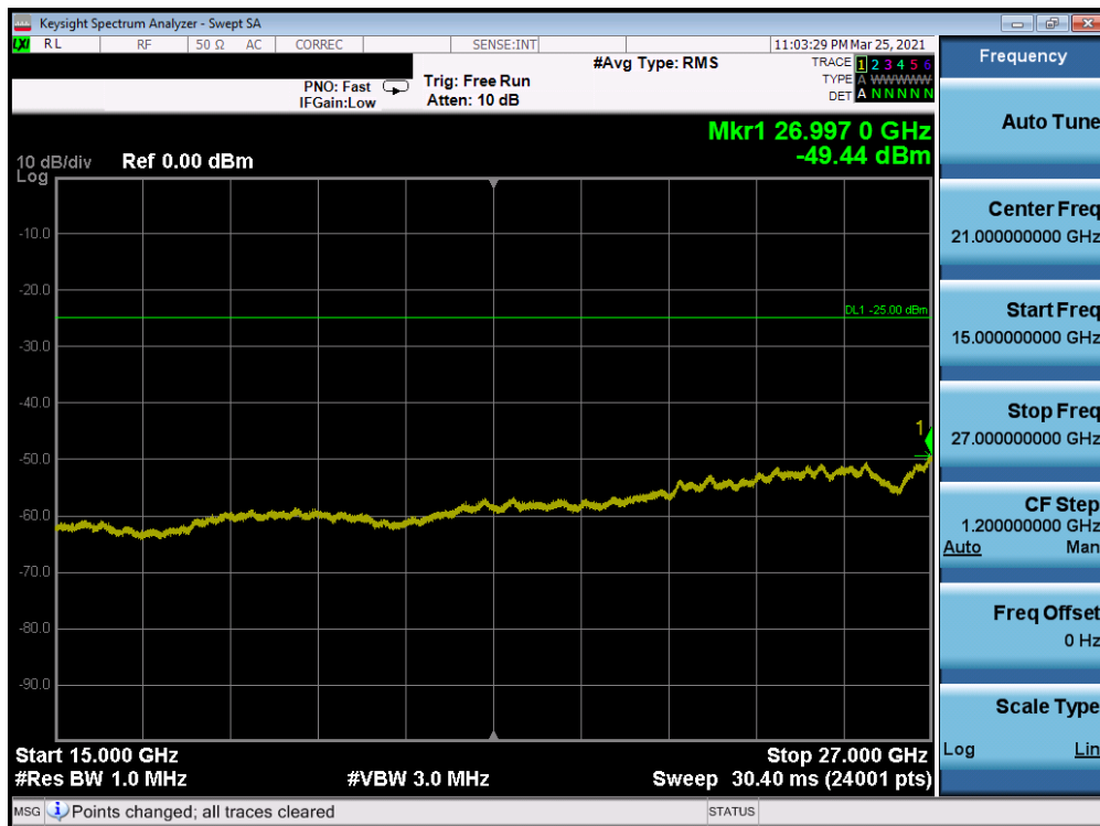
Plot 7-48. CSE (LTE Band 7 - 20MHz QPSK - RB Size 1, RB Offset 0 - Low Channel)
