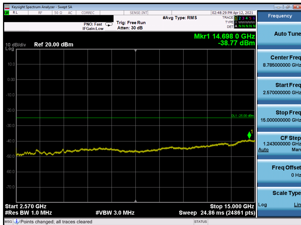
Plot 7-65. CSE (ULCA LTE Band 7 - (20 + 20)MHz QPSK - PCC 1/99 SCC 1/0, - Mid Channel)
