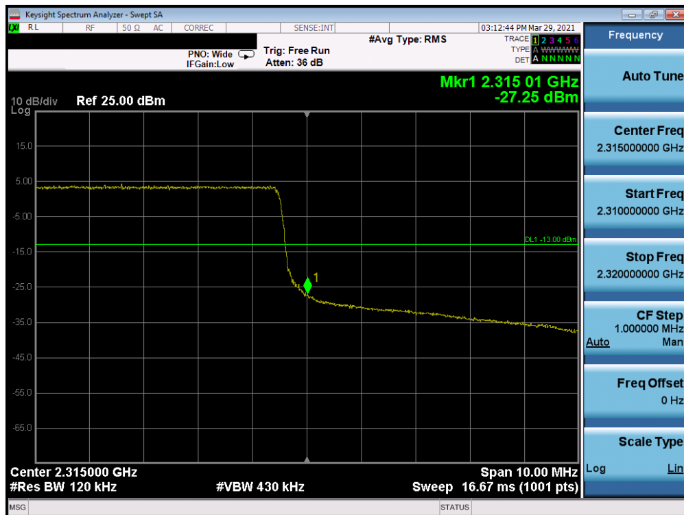
Plot 7-76. Upper Band Edge Plot (Band 30 - 10.0MHz QPSK - Full RB Configuration)
