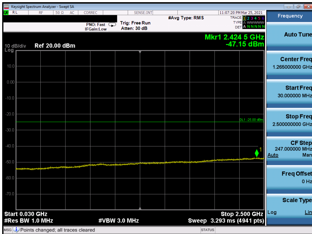
Plot 7-52. CSE (LTE Band 7 - 20MHz QPSK - RB Size 1, RB Offset 0 - High Channel)
