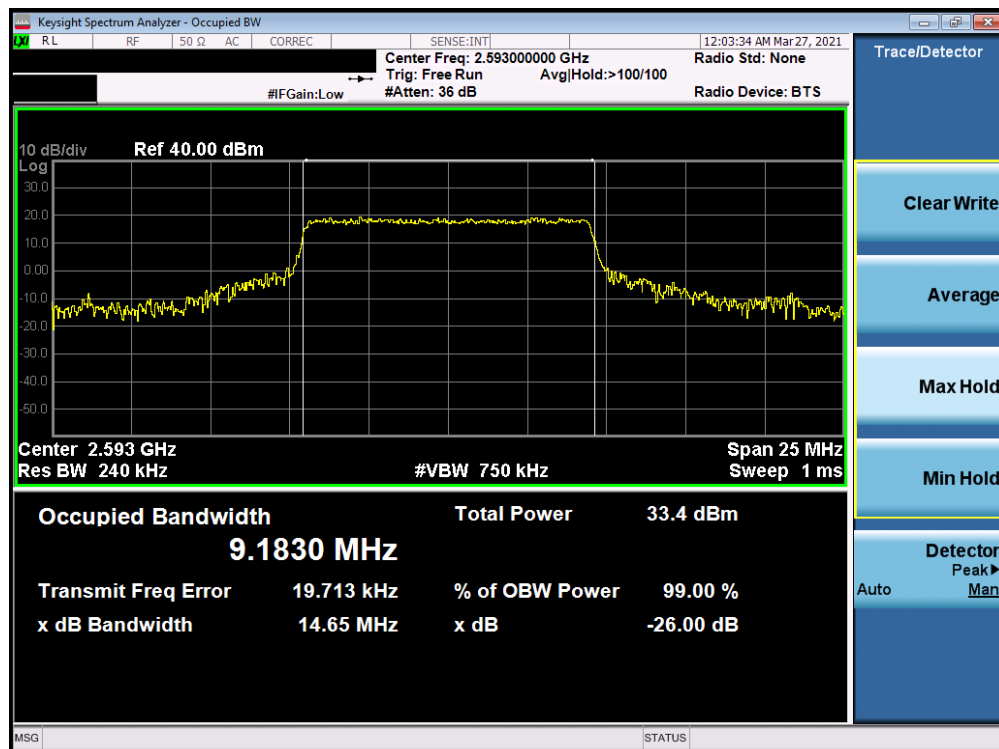
Plot 7-22. Occupied Bandwidth Plot (LTE Band 41 - 10MHz QPSK - Full RB Configuration)
