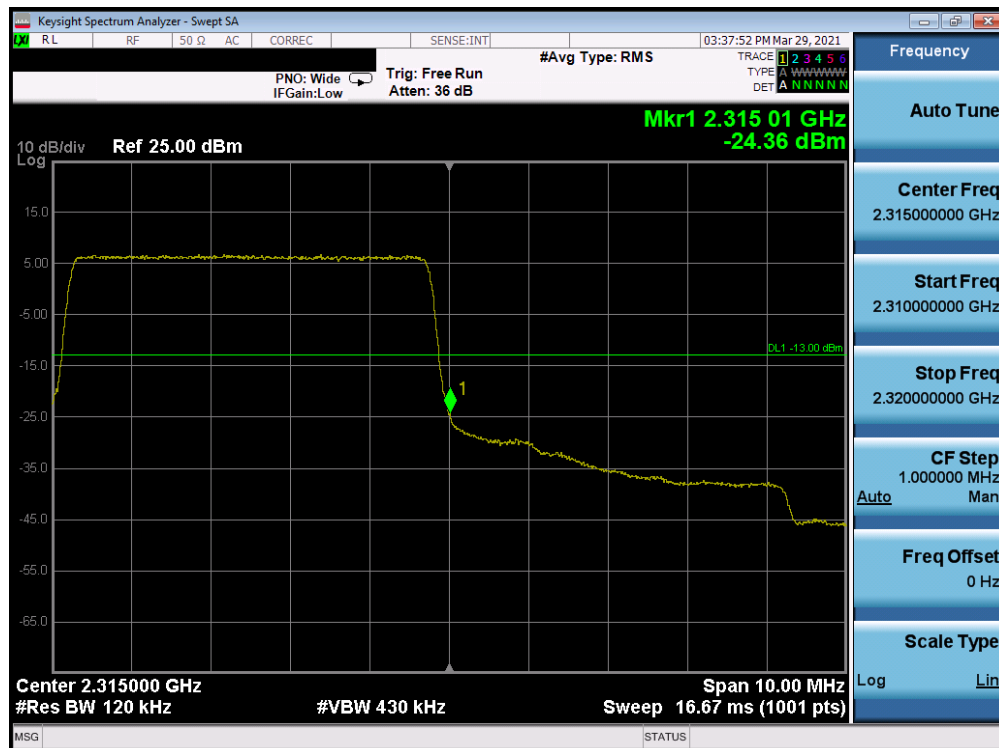
Plot 7-72. Upper Band Edge Plot (Band 30 - 5.0MHz QPSK - Full RB Configuration)
