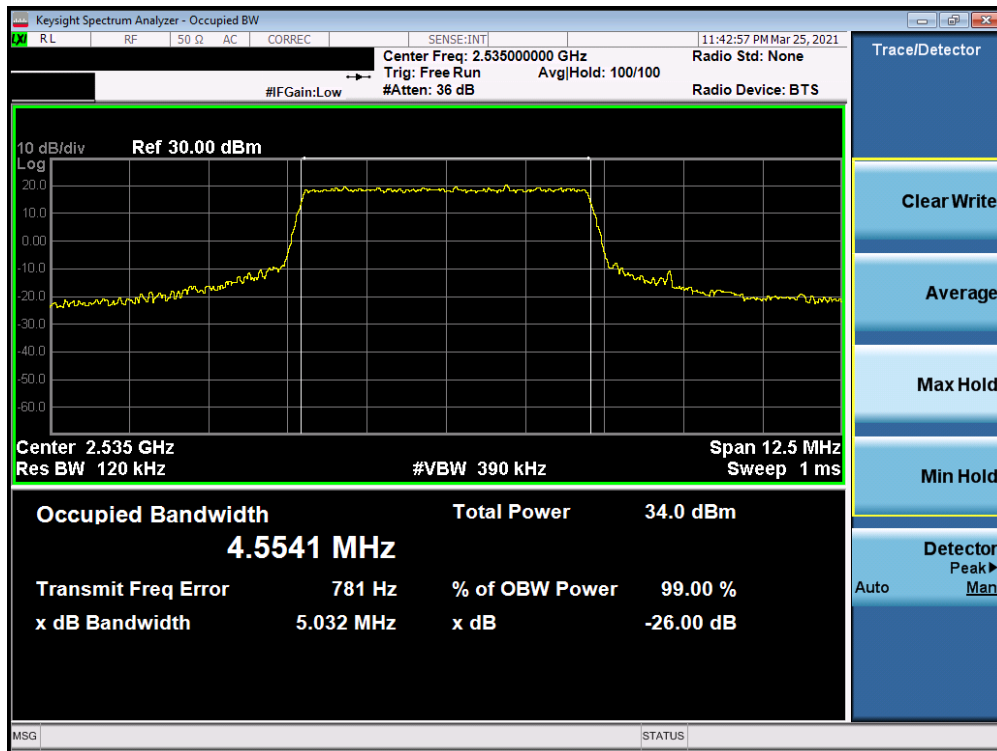
Plot 7-7. Occupied Bandwidth Plot (LTE Band 7 - 5MHz QPSK - Full RB Configuration)
