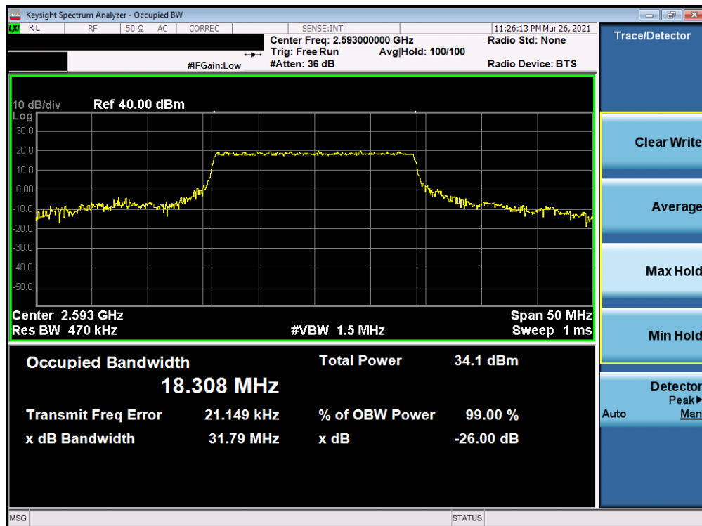
Plot 7-28. Occupied Bandwidth Plot (LTE Band 41 - 20MHz QPSK - Full RB Configuration)
