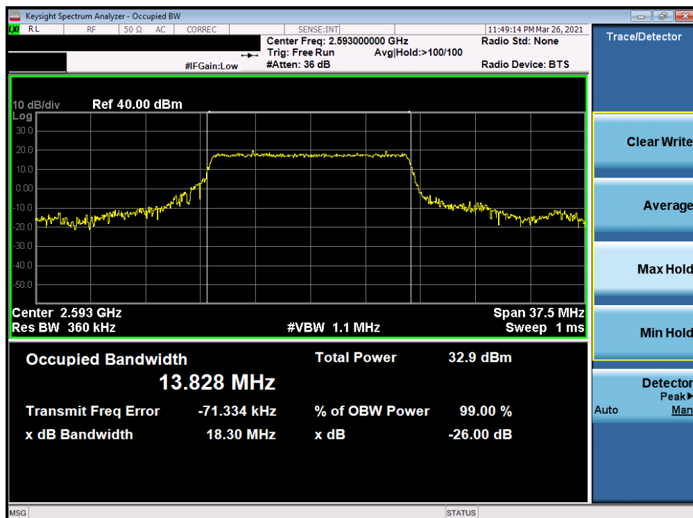
Plot 7-26. Occupied Bandwidth Plot (LTE Band 41 - 15MHz 16-QAM - Full RB Configuration)
