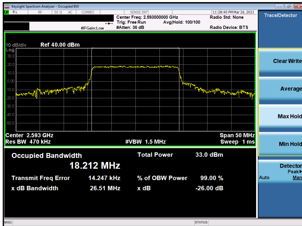
Plot 7-29. Occupied Bandwidth Plot (LTE Band 41 - 20MHz 16-QAM - Full RB Configuration)
