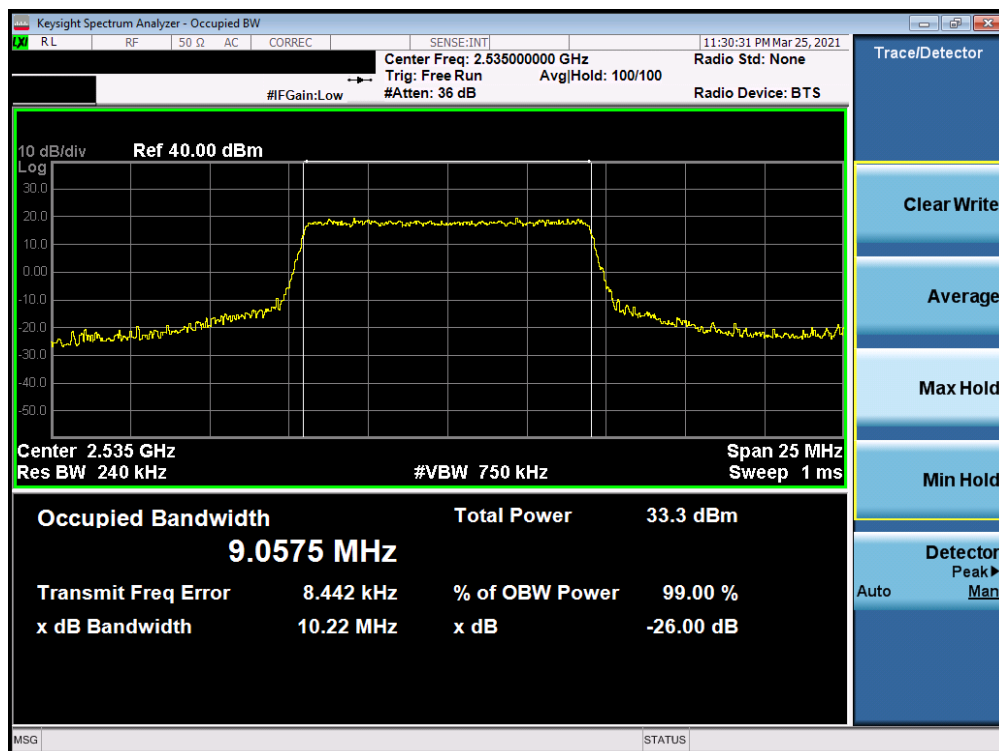
Plot 7-10. Occupied Bandwidth Plot (LTE Band 7 - 10MHz QPSK - Full RB Configuration)
