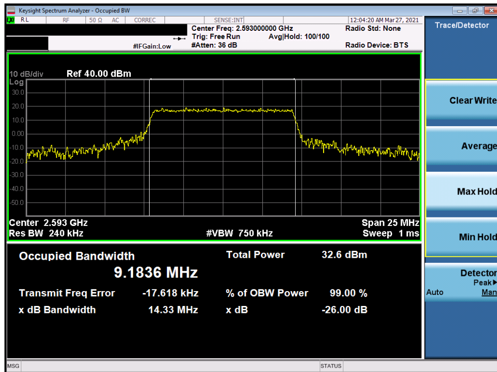
Plot 7-23. Occupied Bandwidth Plot (LTE Band 41 - 10MHz 16-QAM - Full RB Configuration)
