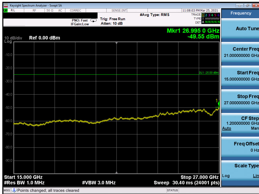
Plot 7-54. CSE (LTE Band 7 - 20MHz QPSK - RB Size 1, RB Offset 0 - High Channel)
