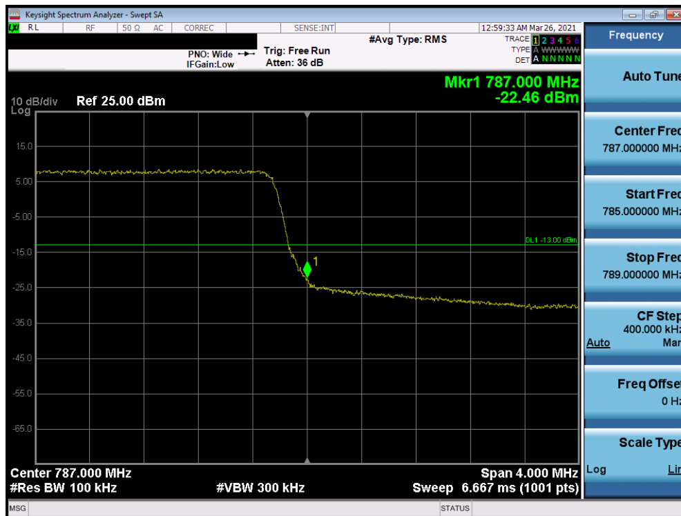
Plot 7-159. Upper Band Edge Plot (Band 13 - 5.0MHz QPSK - Full RB Configuration)
