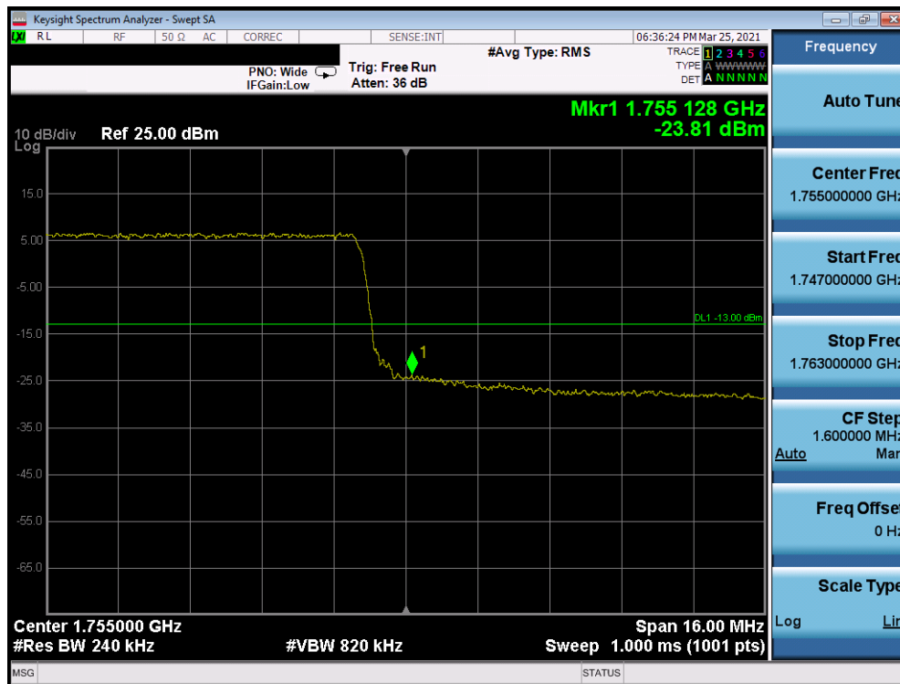
Plot 7-135. Upper Band Edge Plot (Band 4 - 20.0MHz QPSK - Full RB Configuration)
