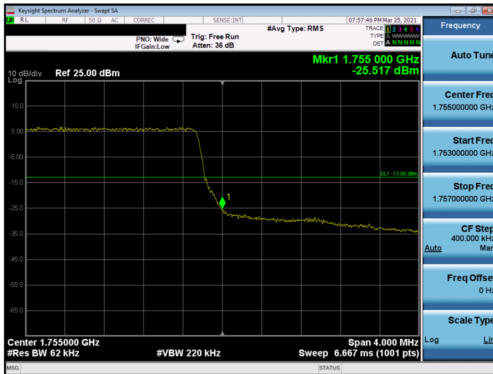
Plot 7-123. Upper Band Edge Plot (Band 4 - 5.0MHz QPSK - Full RB Configuration)
