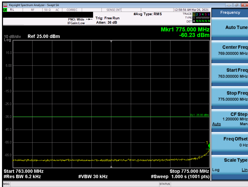
Plot 7-158. Lower Emission Mask Edge Plot (Band 13 - 5.0MHz QPSK - Full RB Configuration)
