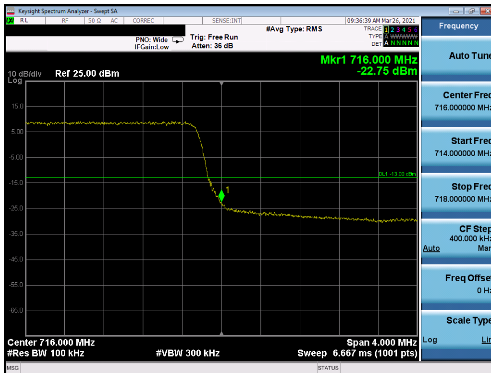
Plot 7-154. Upper Band Edge Plot (Band 17 - 5.0MHz QPSK - Full RB Configuration)
