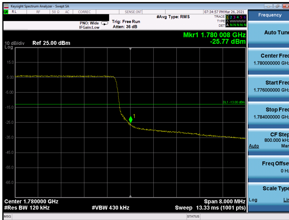
Plot 7-103. Upper Band Edge Plot (Band 66 - 10.0MHz QPSK - Full RB Configuration)
