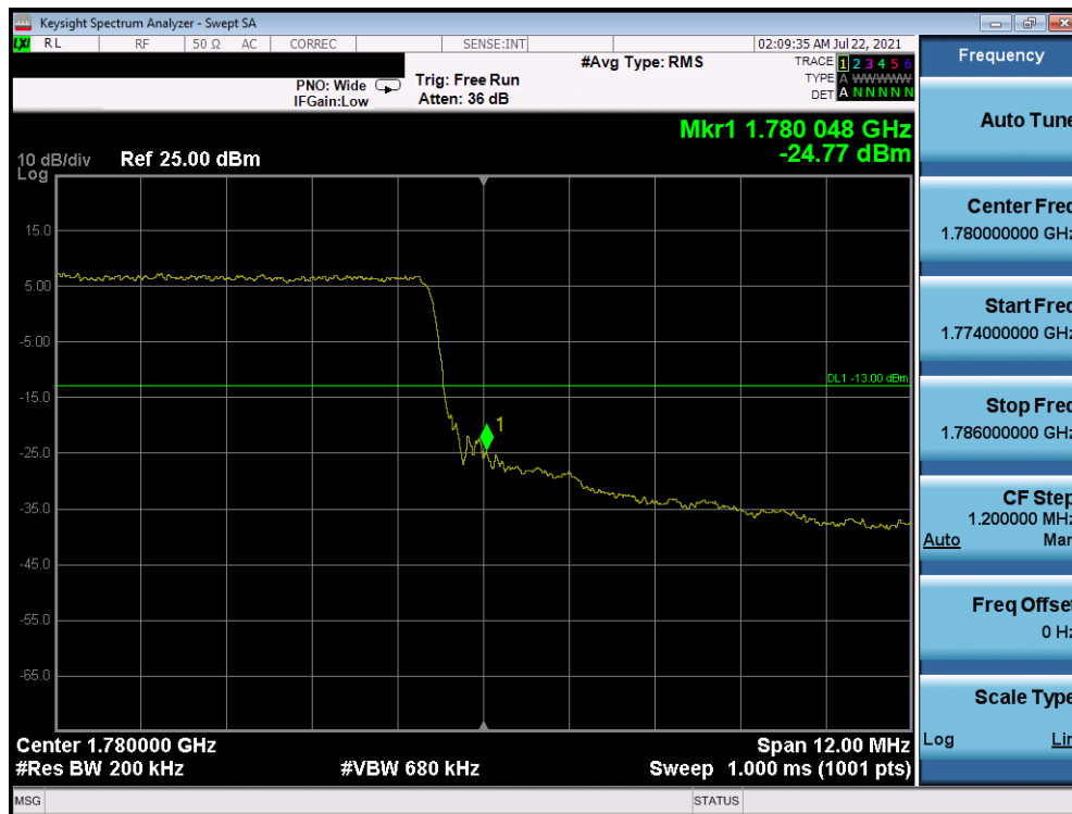
Plot 7-107. Upper Band Edge Plot (Band 66 - 15.0MHz QPSK - Full RB Configuration)
