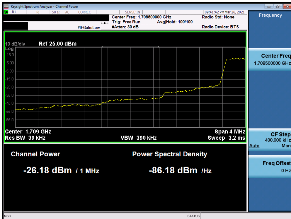
Plot 7-90. Lower Extended Band Edge Plot (Band 66 - 1.4MHz QPSK - Full RB Configuration)
