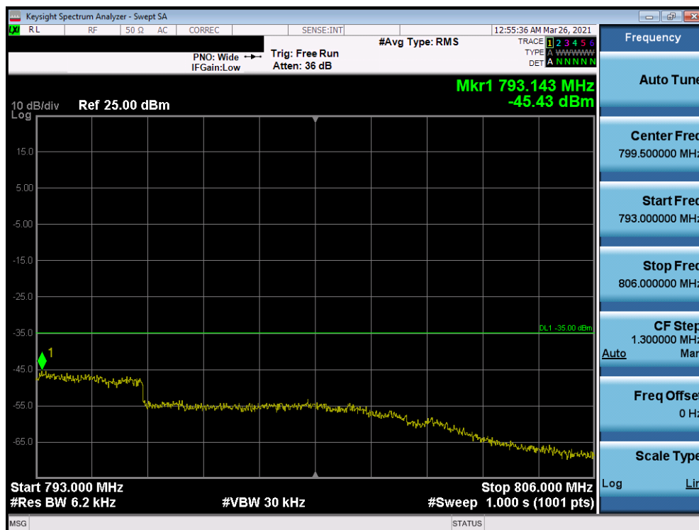
Plot 7-164. Higher Emission Mask Edge Plot (Band 13 - 10.0MHz QPSK - Full RB Configuration)
