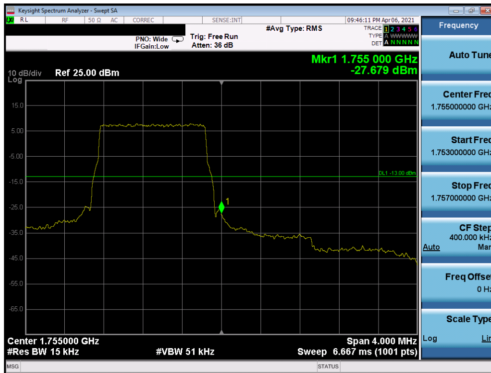
Plot 7-115. Upper Band Edge Plot (Band 4 - 1.4MHz QPSK - Full RB Configuration)
