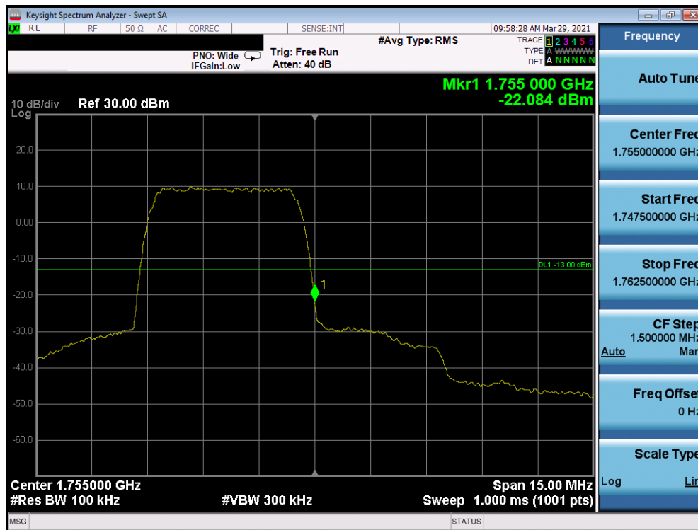
Plot 7-167. Band Edge Plot (AWS WCDMA Mode - High Channel)
