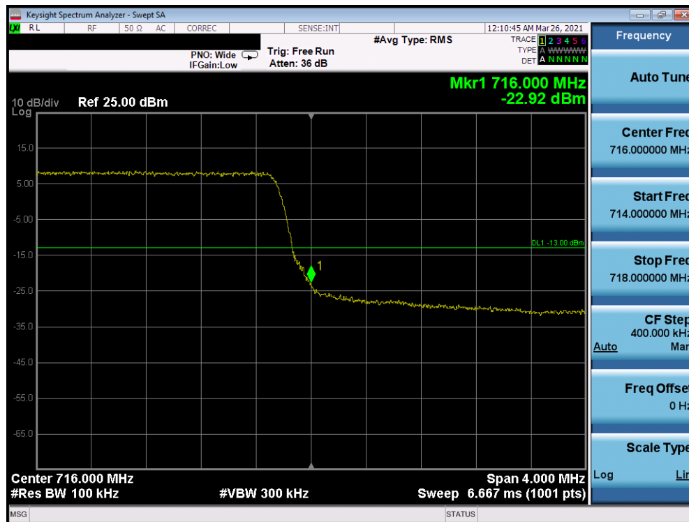
Plot 7-150. Upper Band Edge Plot (Band 12 - 5.0MHz QPSK - Full RB Configuration)
