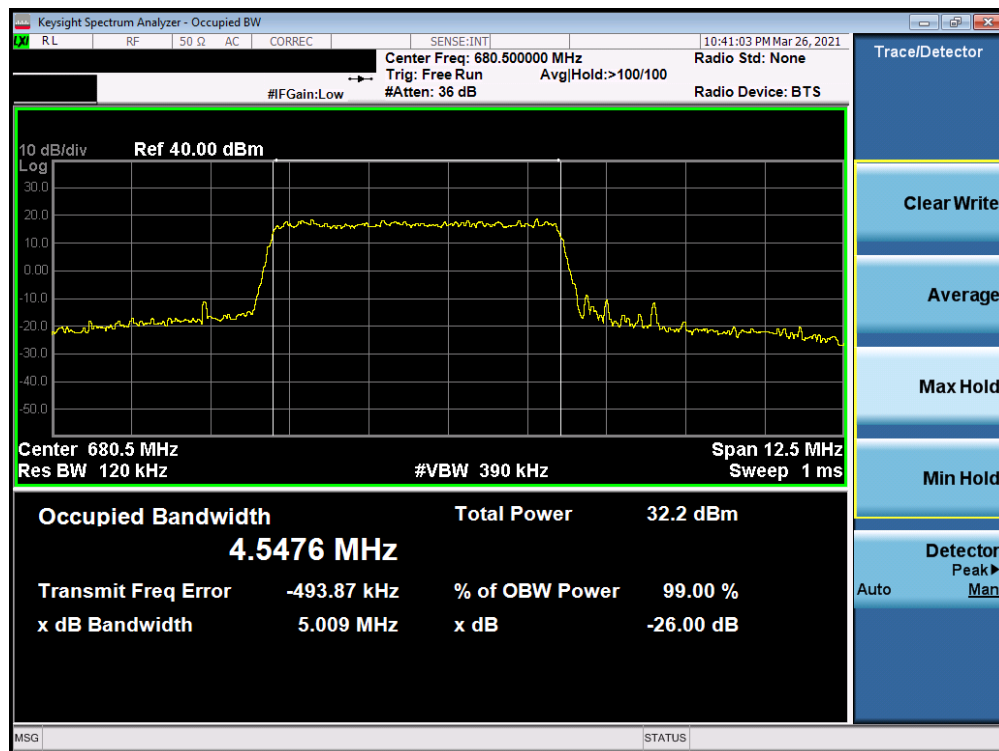
Plot 7-20. Occupied Bandwidth Plot (LTE Band 71 - 5MHz 16-QAM - Full RB Configuration)
