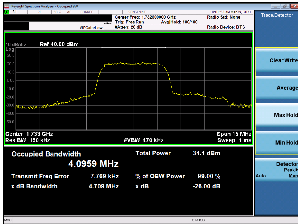
Plot 7-49. Occupied Bandwidth Plot (WCDMA, Ch. 1413)
