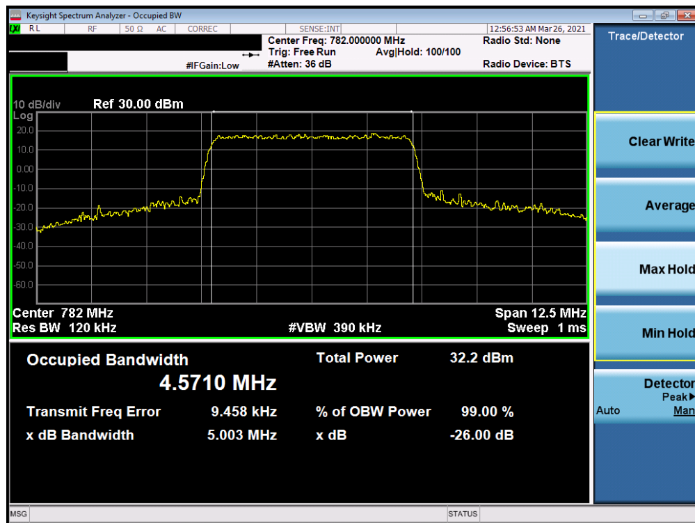
Plot 7-44. Occupied Bandwidth Plot (LTE Band 13 - 5MHz 16-QAM - Full RB Configuration)
