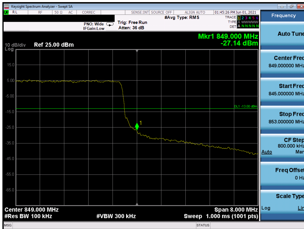
Plot 7-39. Upper Band Edge Plot (LTE Band 26 - 10MHz QPSK - Full RB Configuration)
