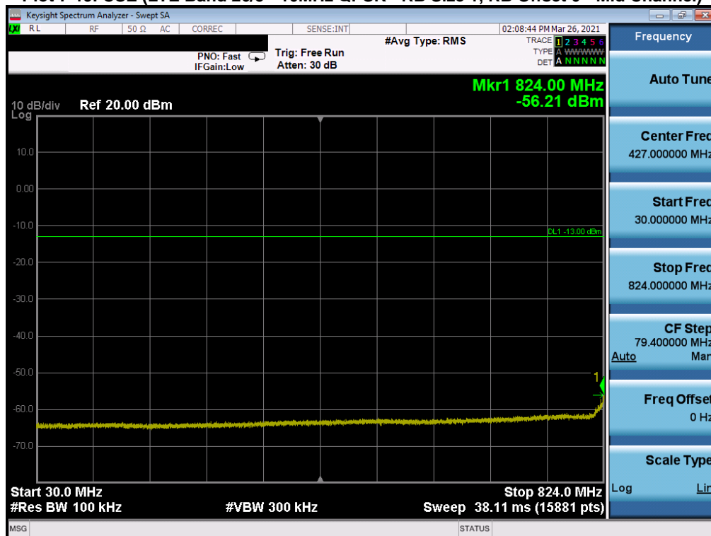
Plot 7-20. CSE (LTE Band 26/5 - 10MHz QPSK - RB Size 1, RB Offset 0 - High Channel)
