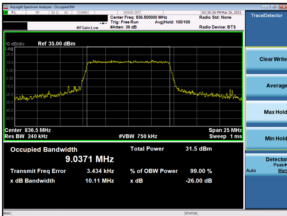
Plot 7-12. Occupied Bandwidth Plot (LTE Band 26/5 - 10MHz 64-QAM - Full RB Configuration)
