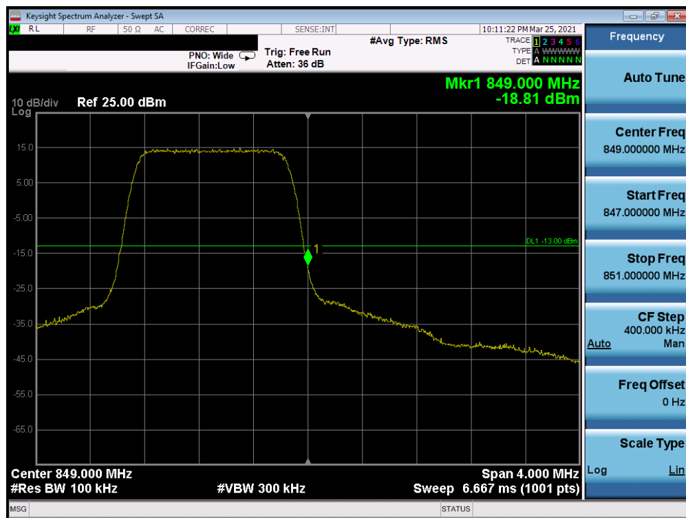
Plot 7-41. Upper Band Edge Plot (LTE Band 5 – 1.4MHz QPSK – Full RB Configuration)
