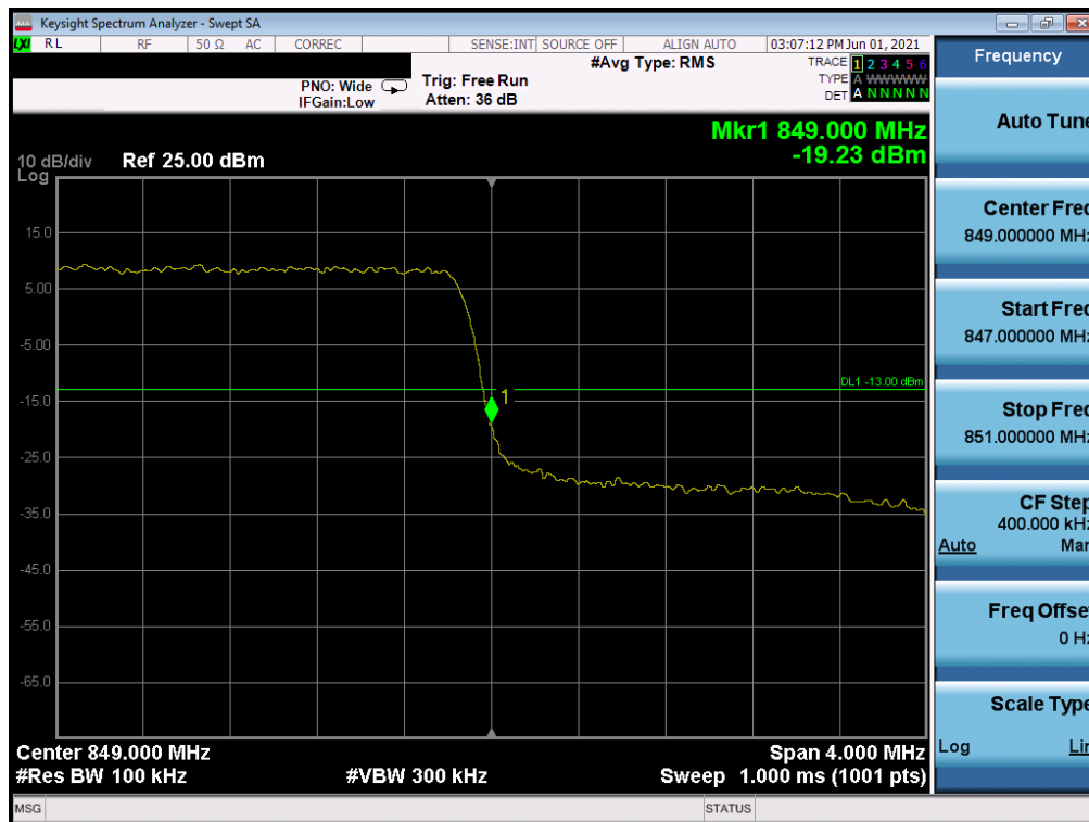
Plot 7-43. Upper Band Edge Plot (LTE Band 5 - 3MHz QPSK – Full RB Configuration)
