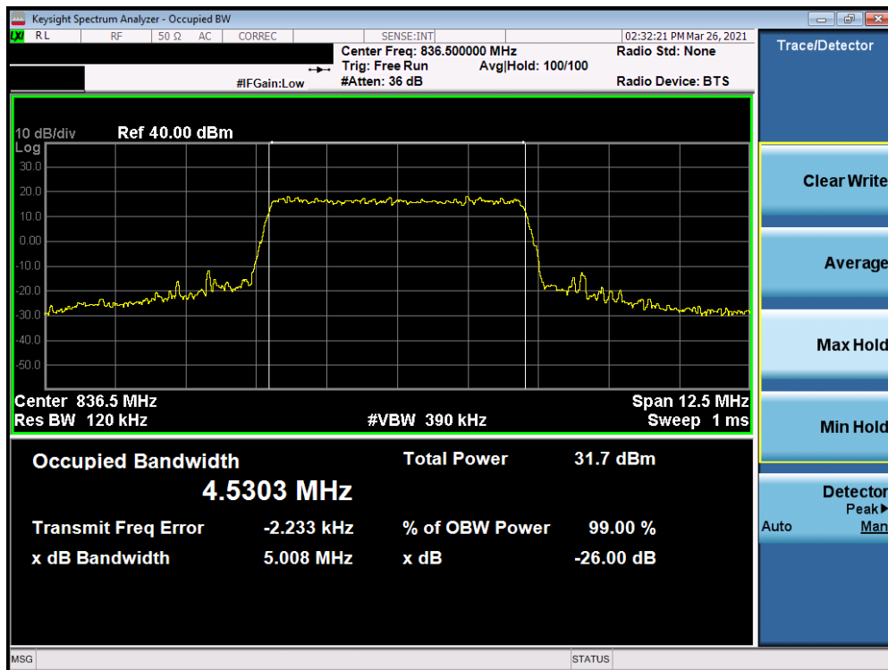
Plot 7-9. Occupied Bandwidth Plot (LTE Band 26/5 - 5MHz 64-QAM - Full RB Configuration)
