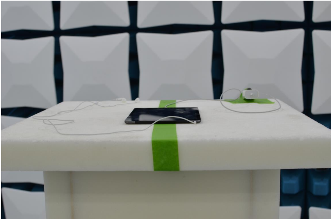
Figure 1: 1-18GHz Test Setup (Front View)
