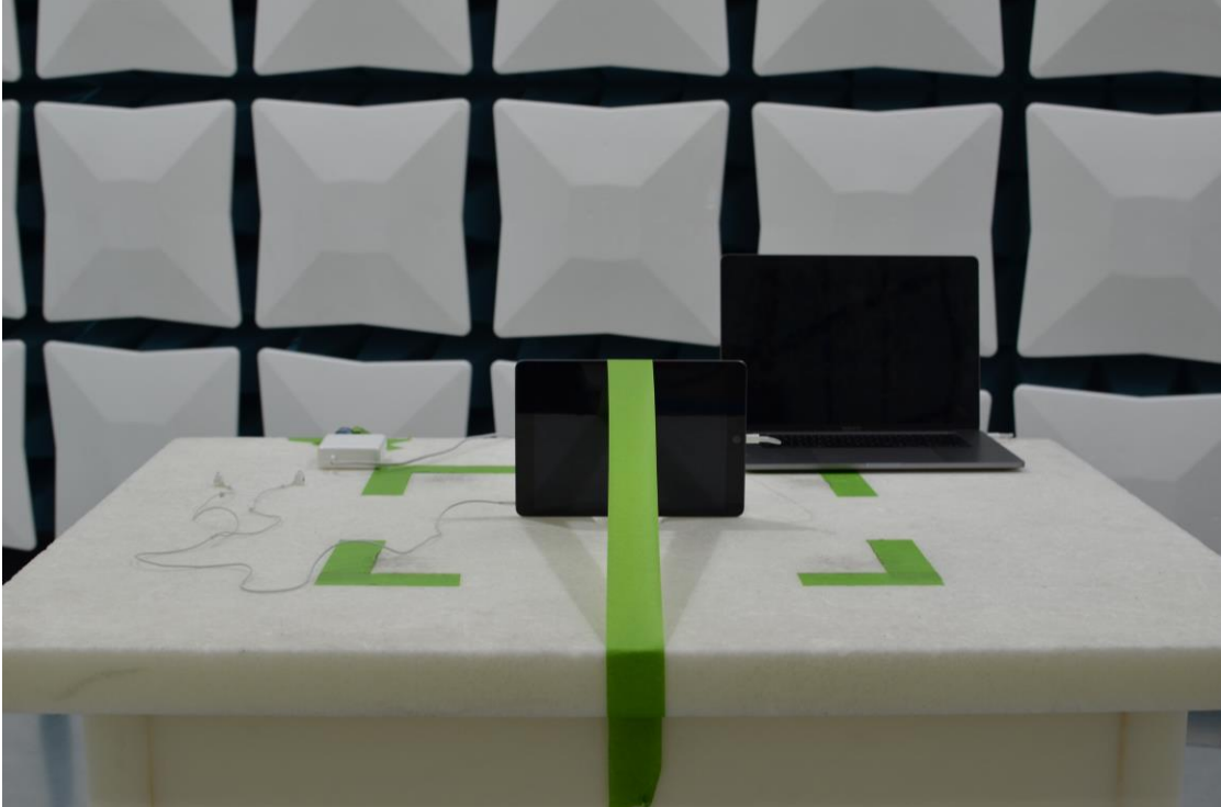
Figure 15: 30MHz-1GHz Test Setup (Front View)
