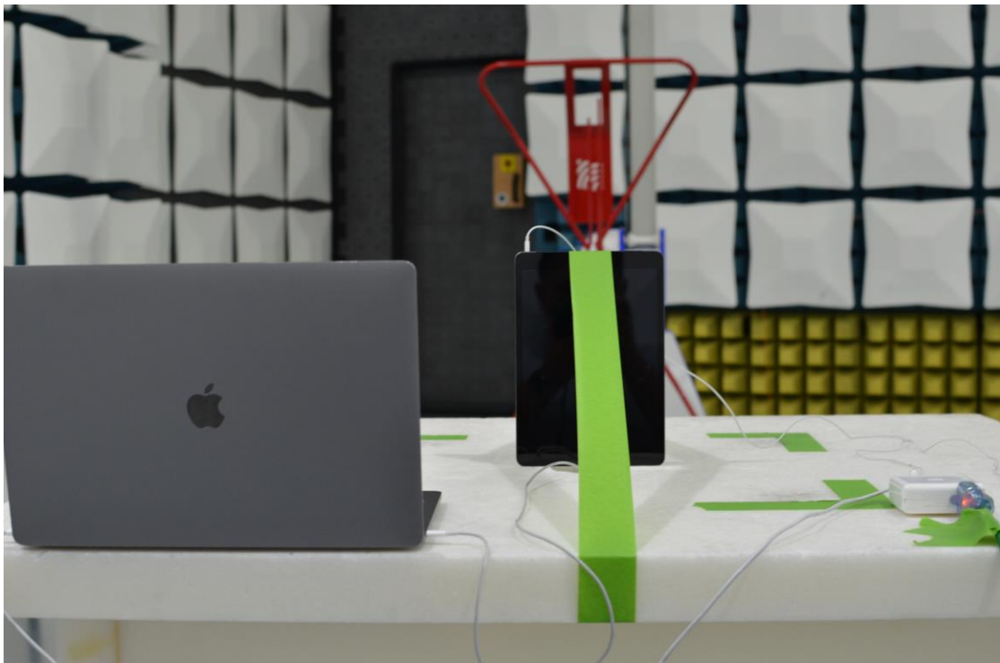
Figure 18: 30MHz-1GHz Test Setup (Rear View)
