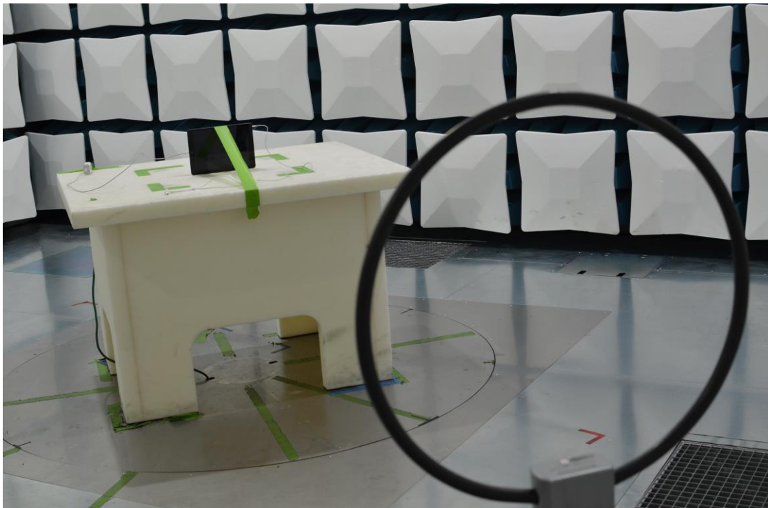
Figure 20: 9kHz-30MHz Test Setup (Front View)
