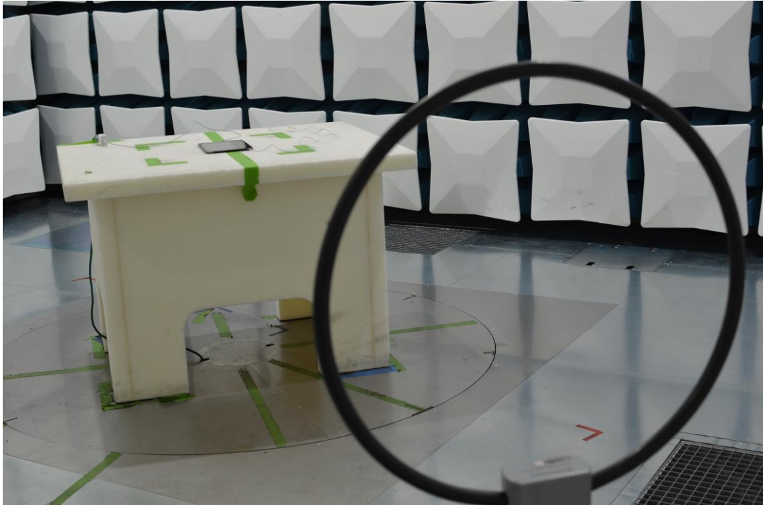
Figure 19: 9kHz-30MHz Test Setup (Front View)
