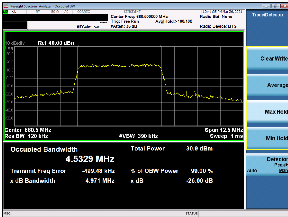
Plot 7-21. Occupied Bandwidth Plot (LTE Band 71 - 5MHz 64-QAM - Full RB Configuration)
