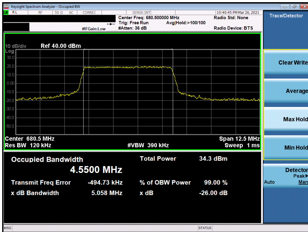
Plot 7-19. Occupied Bandwidth Plot (LTE Band 71 - 5MHz QPSK - Full RB Configuration)
