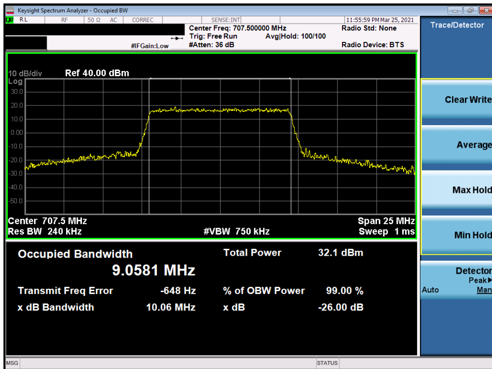
Plot 7-41. Occupied Bandwidth Plot (LTE Band 12/17 - 10MHz 16-QAM - Full RB Configuration)
