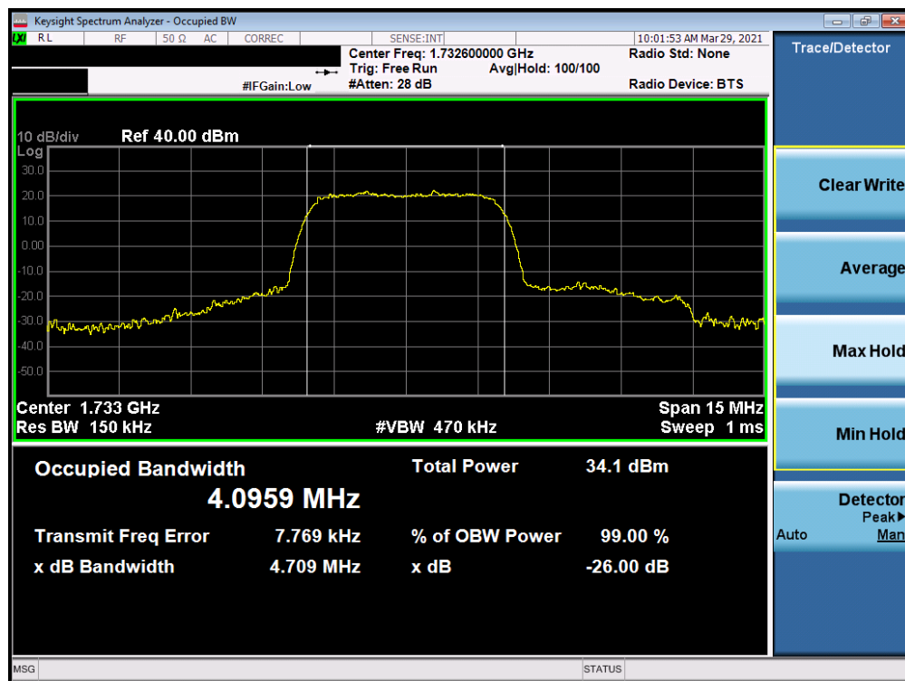
Plot 7-49. Occupied Bandwidth Plot (WCDMA, Ch. 1413)
