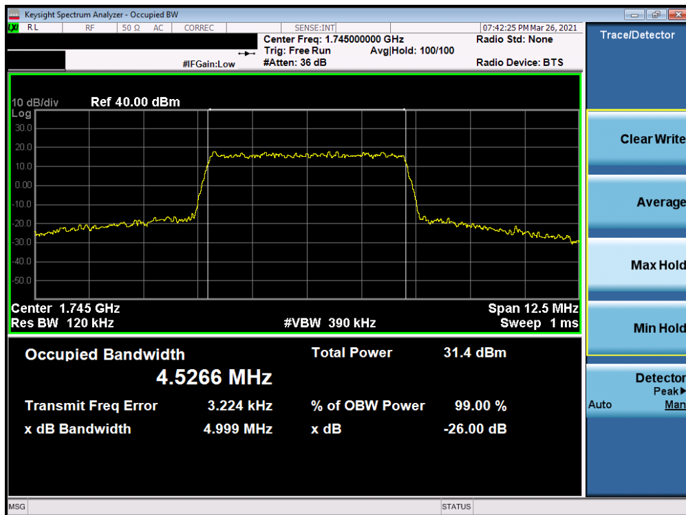
Plot 7-9. Occupied Bandwidth Plot (LTE Band 66/4 - 5MHz 64-QAM - Full RB Configuration)
