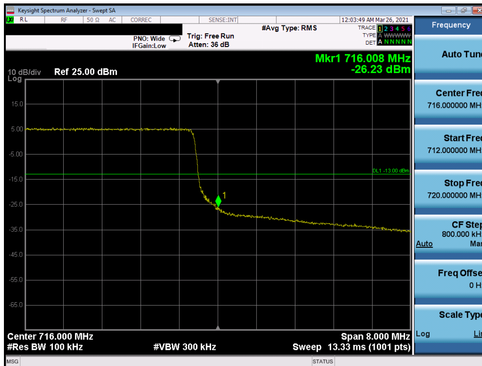
Plot 7-152. Upper Band Edge Plot (Band 12 - 10.0MHz QPSK - Full RB Configuration)
