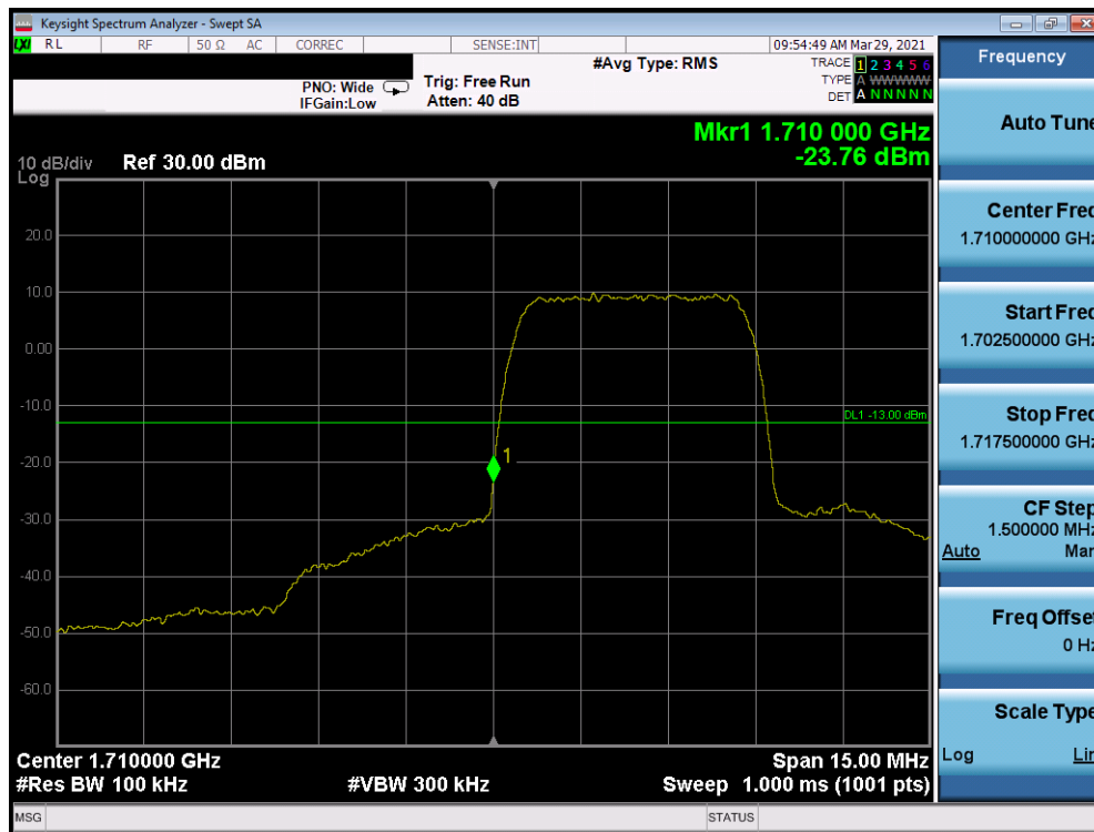
Plot 7-165. Band Edge Plot (AWS WCDMA Mode - Low Channel)
