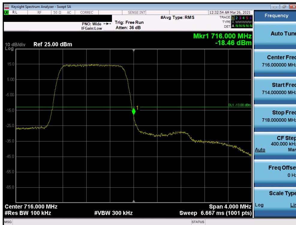
Plot 7-146. Upper Band Edge Plot (Band 12 - 1.4MHz QPSK - Full RB Configuration)
