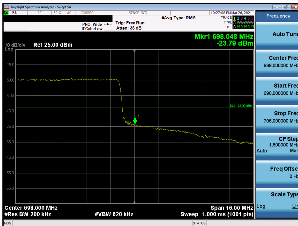
Plot 7-144. Upper Band Edge Plot (Band 71 - 20.0MHz QPSK - Full RB Configuration)
