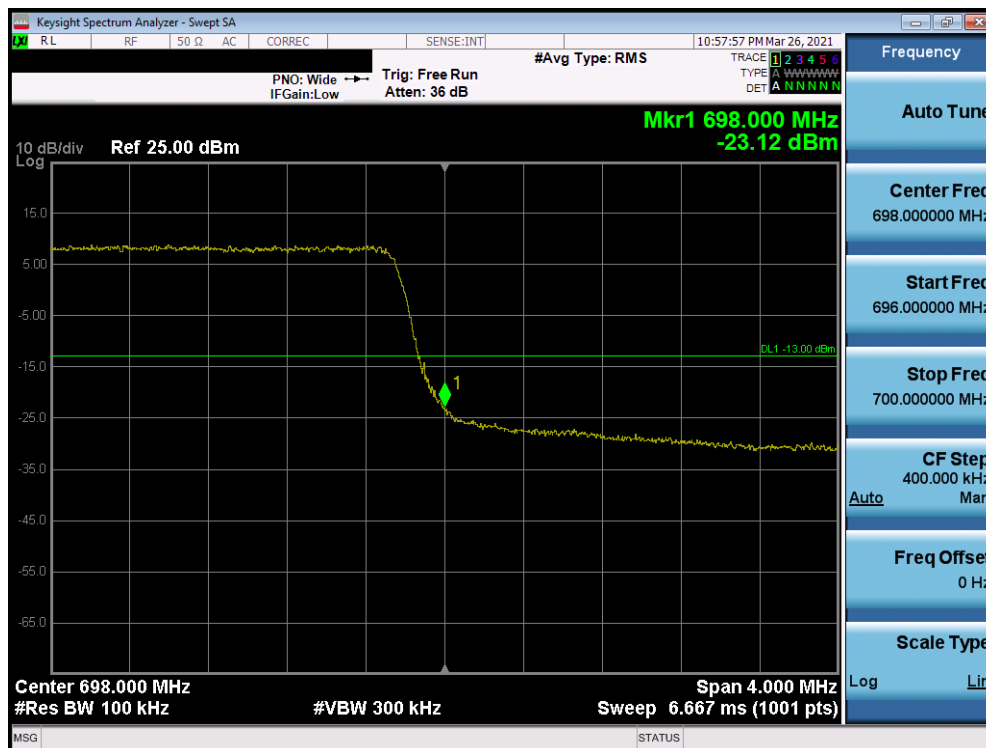
Plot 7-138. Upper Band Edge Plot (Band 71 - 5.0MHz QPSK - Full RB Configuration)
