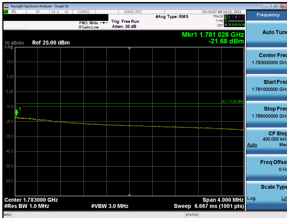
Plot 7-108. Upper Extended Band Edge Plot (Band 66 - 15.0MHz QPSK - Full RB Configuration)
