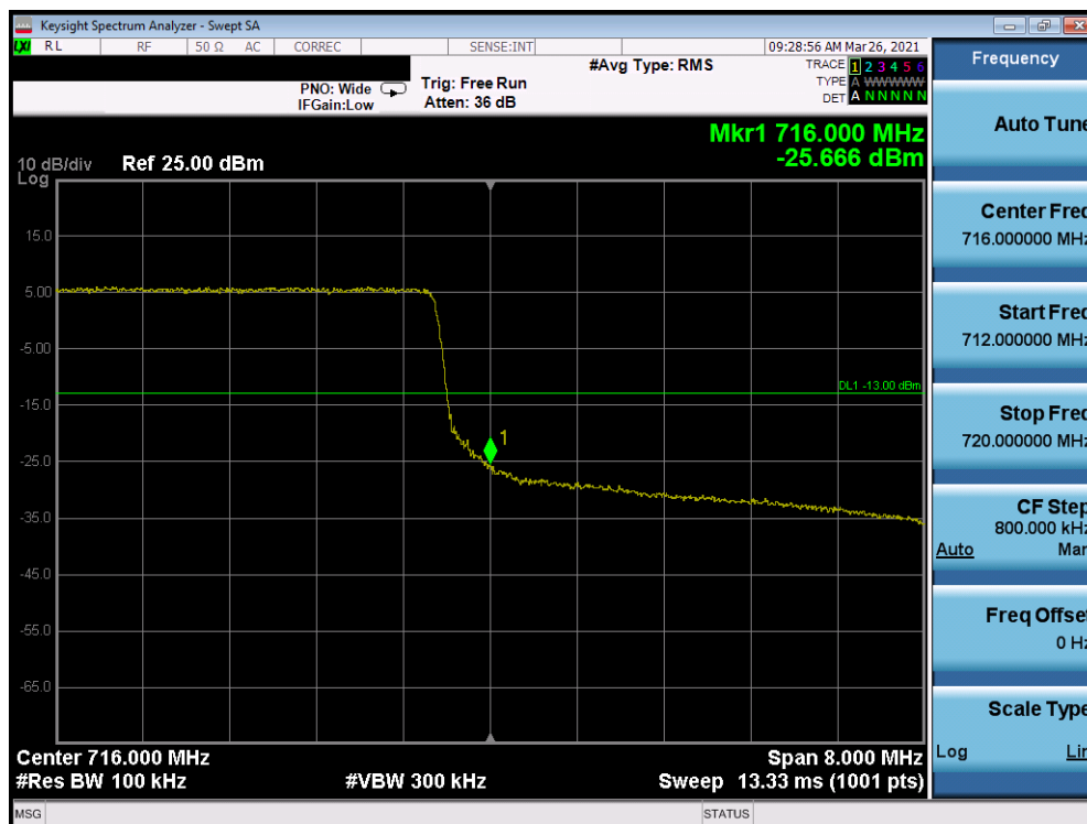
Plot 7-156. Upper Band Edge Plot (Band 17 - 10.0MHz QPSK - Full RB Configuration)
