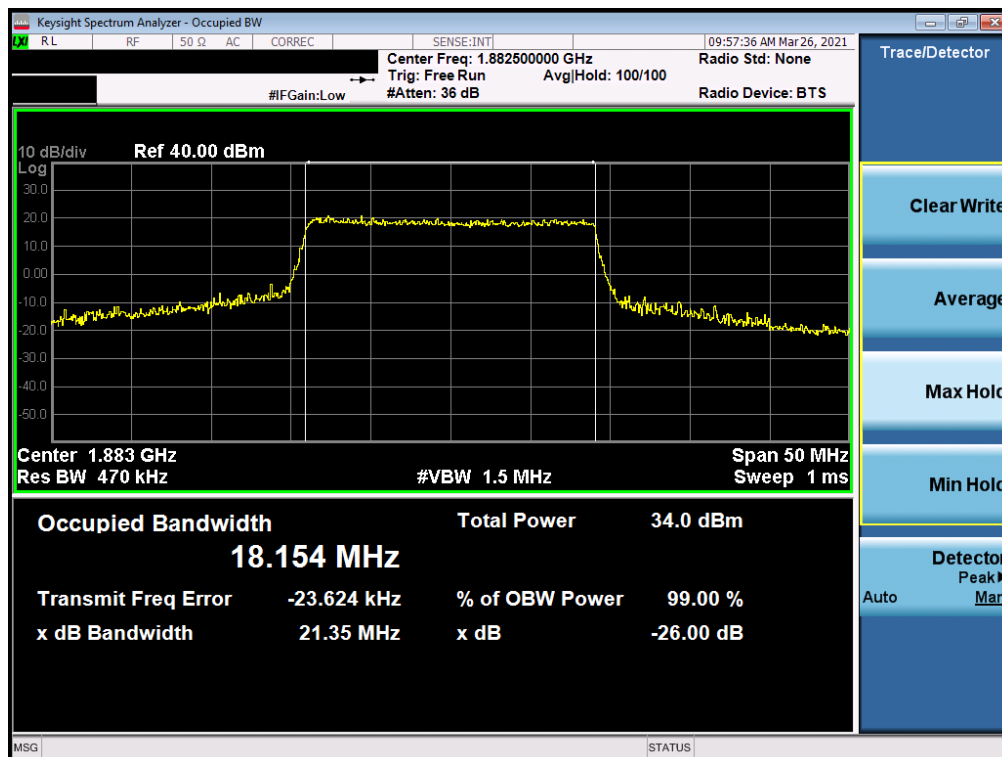
Plot 7-16. Occupied Bandwidth Plot (LTE Band 25/2 - 20MHz QPSK - Full RB Configuration)
