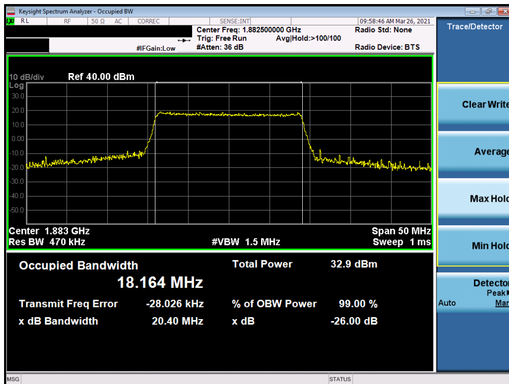
Plot 7-18. Occupied Bandwidth Plot (LTE Band 25/2 - 20MHz 64-QAM - Full RB Configuration)
