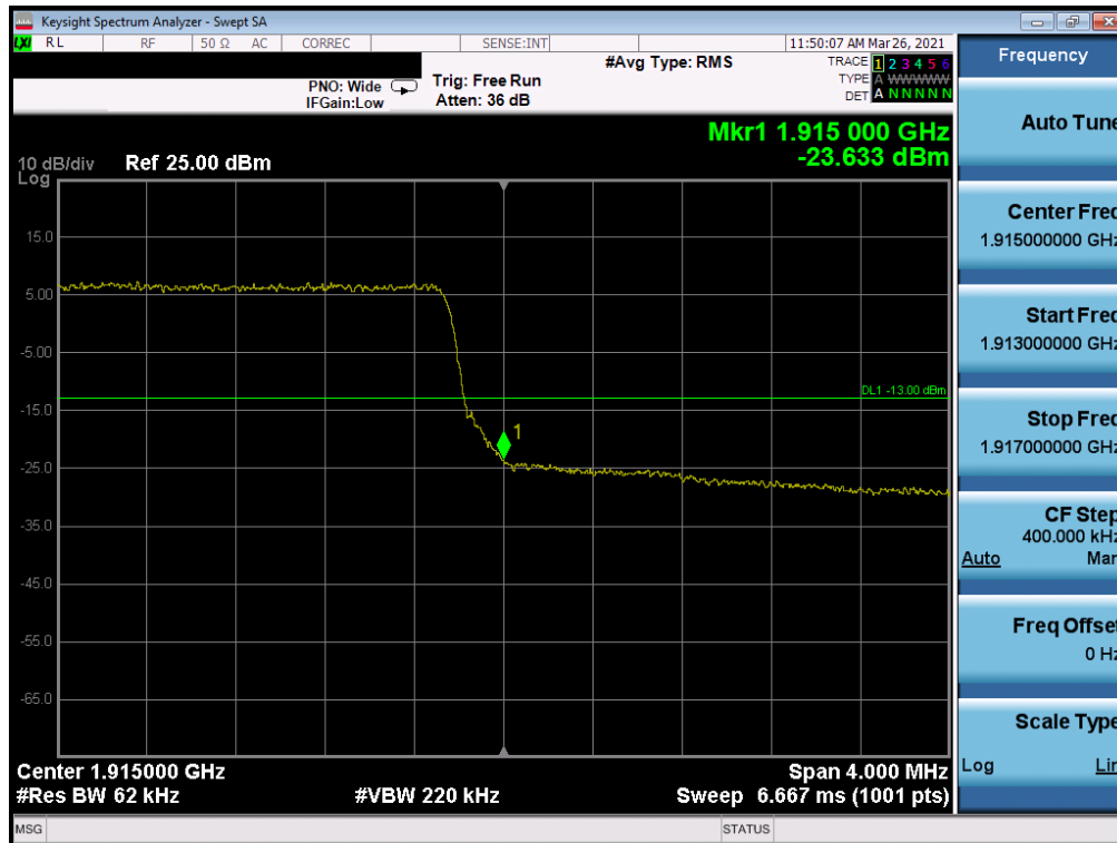
Plot 7-48. Upper Band Edge Plot (LTE Band 25 - 5MHz QPSK – Full RB Configuration)
