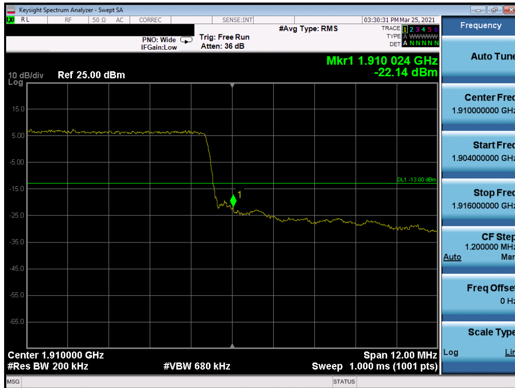
Plot 7-80. Upper Band Edge Plot (LTE Band 2 - 15MHz QPSK – Full RB Configuration)
