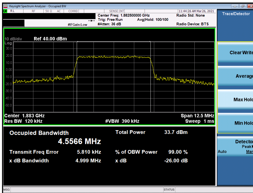
Plot 7-8. Occupied Bandwidth Plot (LTE Band 25/2 - 5MHz 16-QAM - Full RB Configuration)
