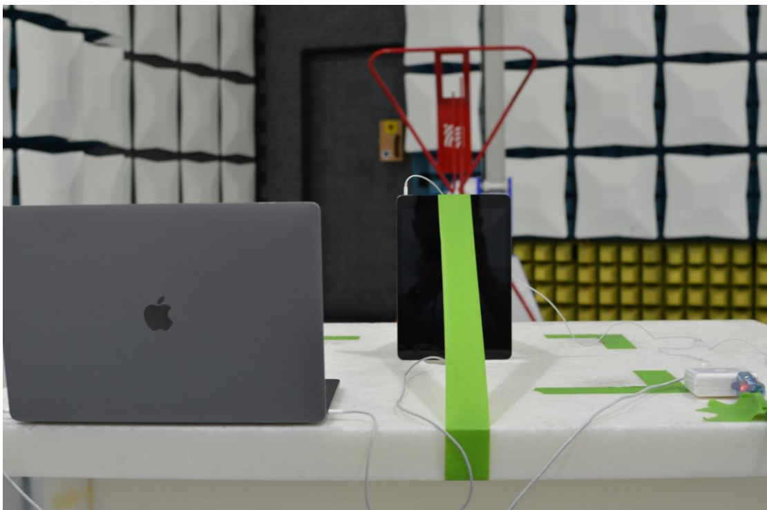
Figure 22: 30MHz-1GHz Test Setup (Rear View)
