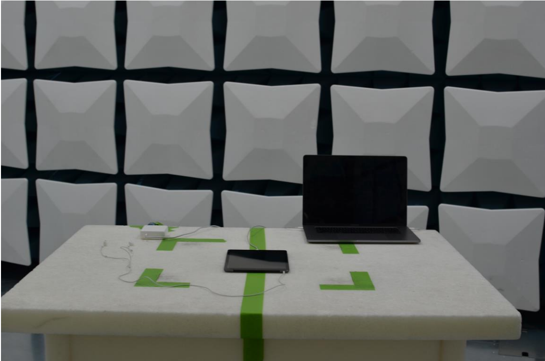
Figure 17: 30MHz-1GHz Test Setup (Front View)
