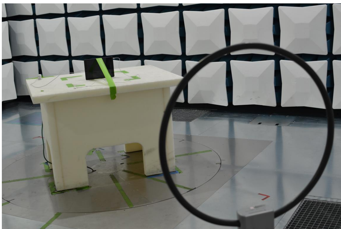
Figure 24: 9kHz-30MHz Test Setup (Front View)
