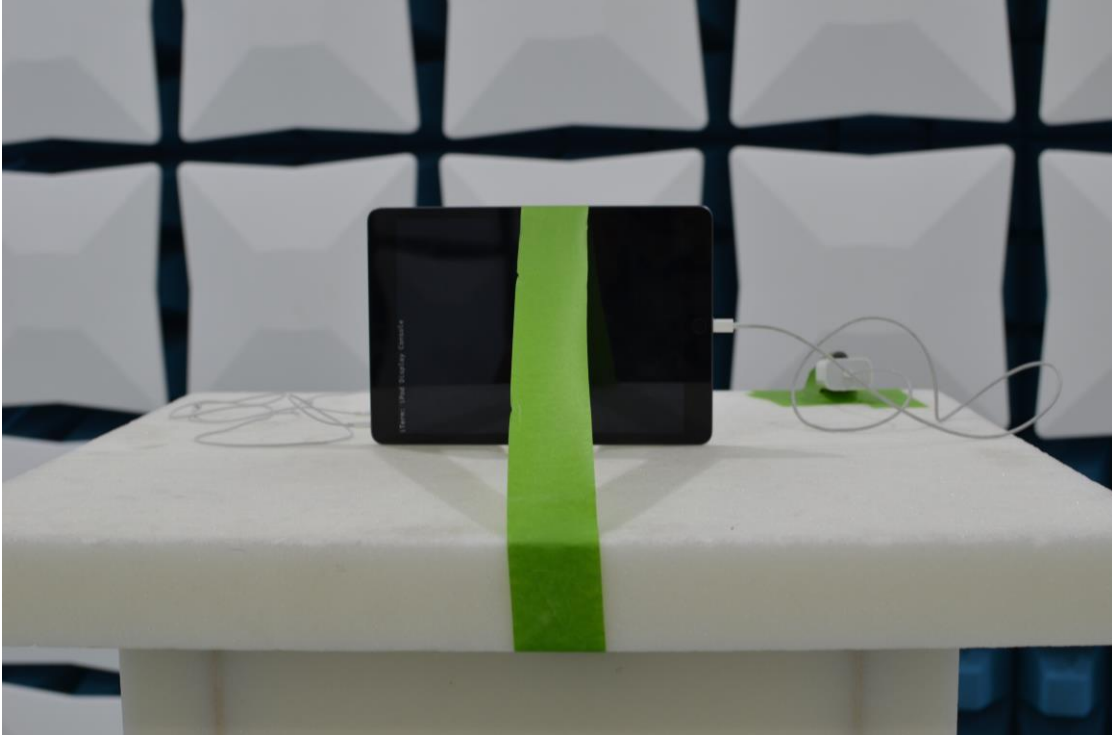
Figure 7: 1-18GHz Test Setup (Front View)
