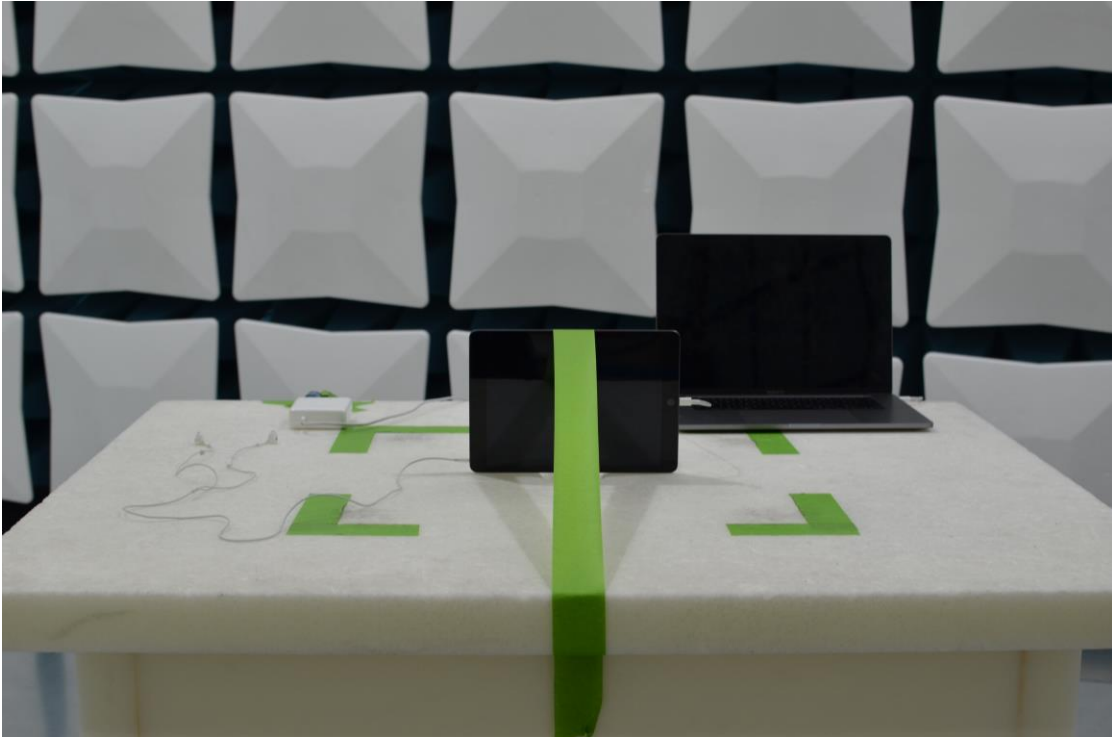
Figure 19: 30MHz-1GHz Test Setup (Front View)
