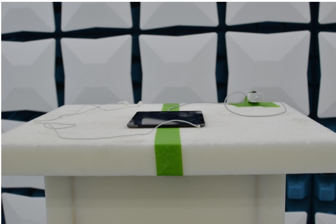
Figure 5: 1-18GHz Test Setup (Front View)
