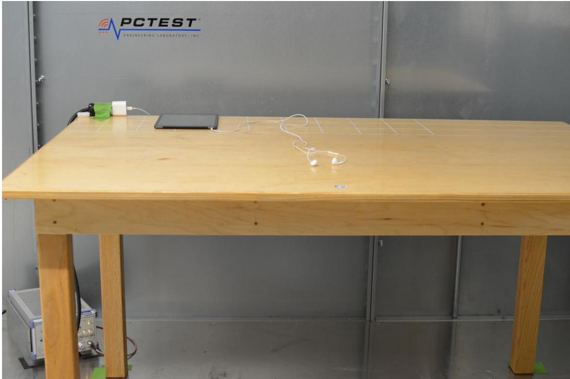
Figure 1: AC Line Conducted Emissions (Front View)
