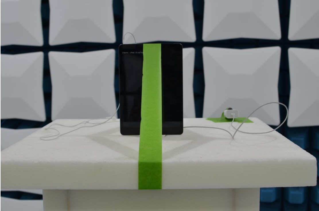
Figure 9: 1-18GHz Test Setup (Front View)
