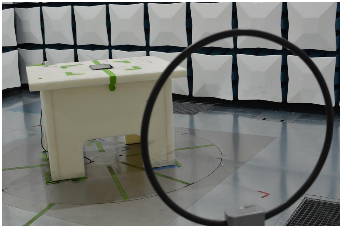
Figure 23: 9kHz-30MHz Test Setup (Front View)
