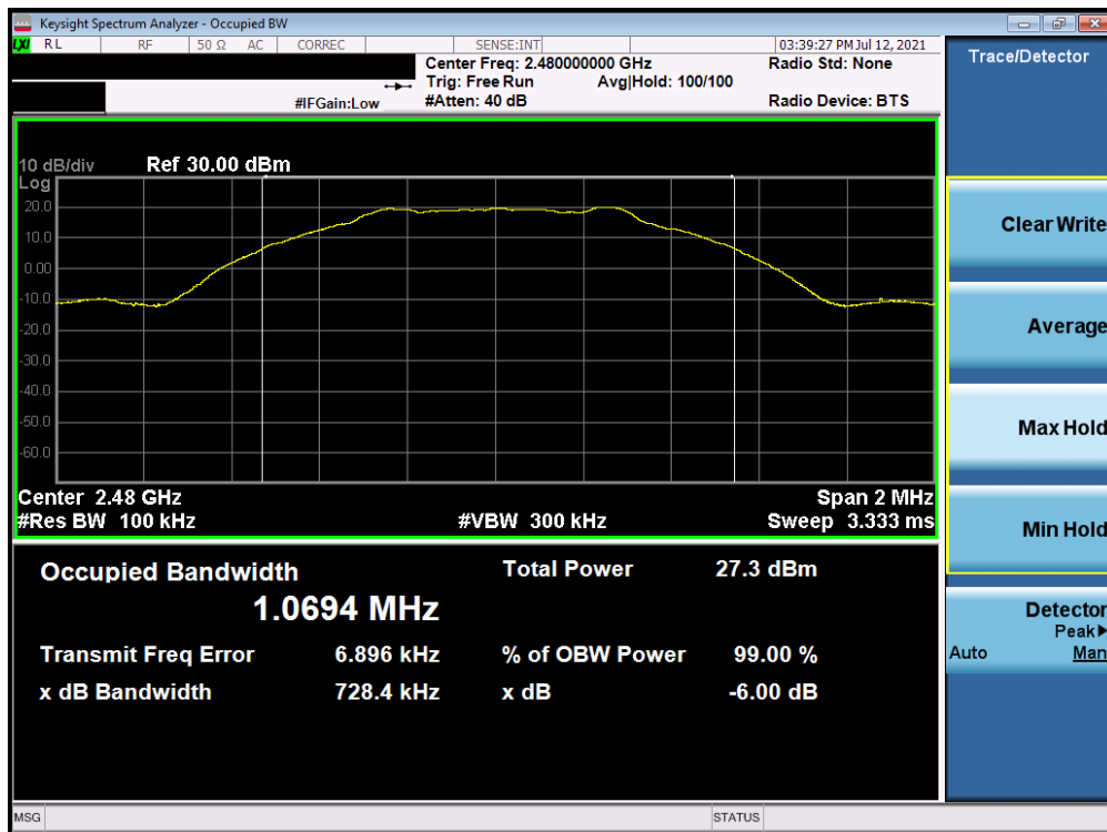
Plot 7-3. 6dB Bandwidth Plot Antenna A (Bluetooth (LE), 1Mbps, ePA – Ch. 39)
