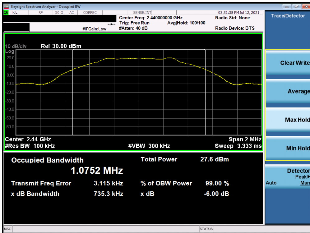
Plot 7-2. 6dB Bandwidth Plot Antenna A (Bluetooth (LE), 1Mbps, ePA – Ch. 19)
