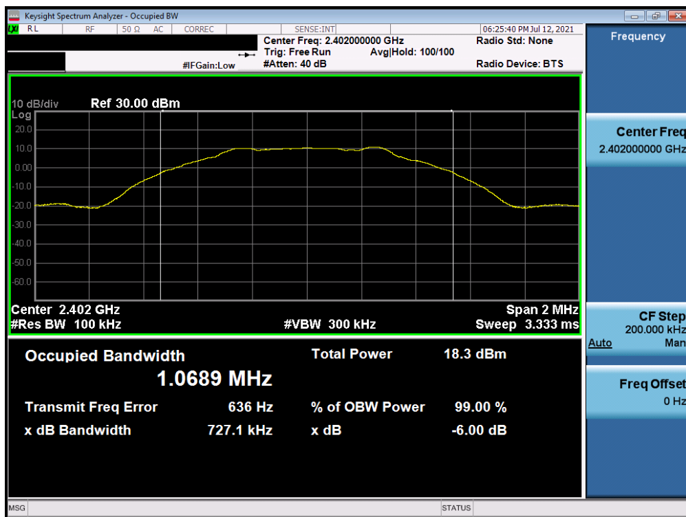
Plot 7-4. 6dB Bandwidth Plot Antenna A (Bluetooth (LE), 1Mbps, iPA – Ch. 0)
