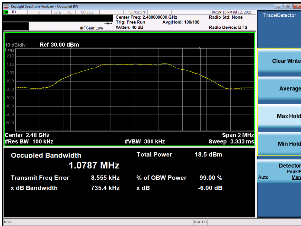
Plot 7-6. 6dB Bandwidth Plot Antenna A (Bluetooth (LE), 1Mbps, iPA – Ch. 39)
