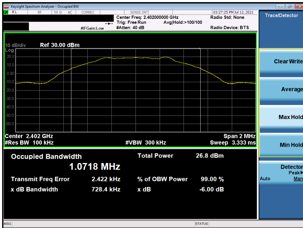
Plot 7-1. 6dB Bandwidth Plot Antenna A (Bluetooth (LE), 1Mbps, ePA – Ch. 0)
