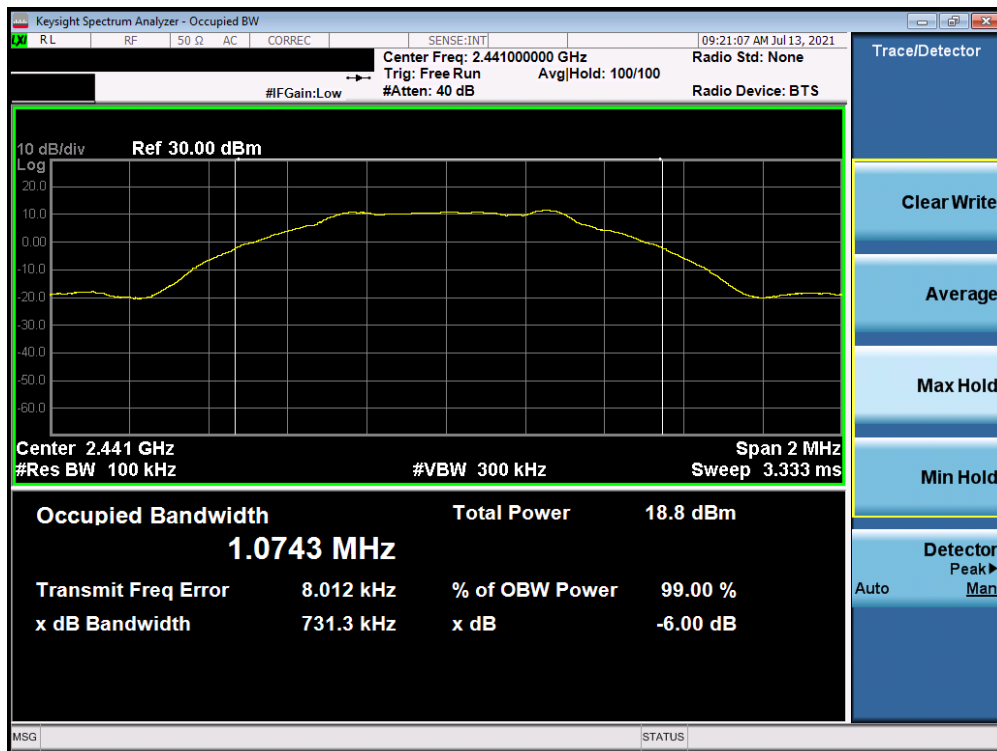
Plot 7-5. 6dB Bandwidth Plot Antenna A (Bluetooth (LE), 1Mbps, iPA – Ch. 19)
