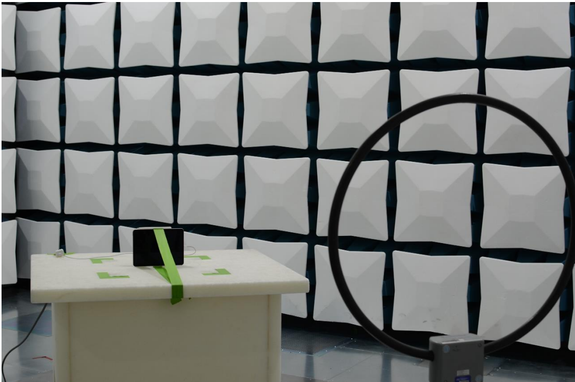
Figure 20: 9kHz-30MHz Test Setup (Front View)
