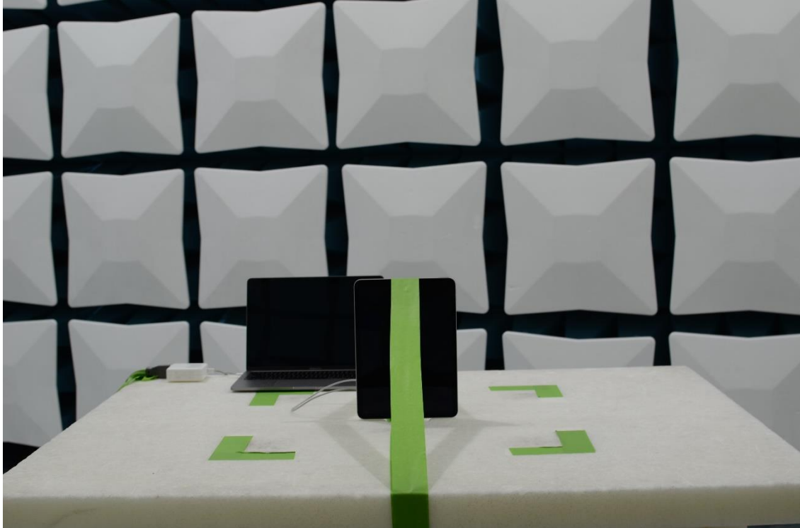
Figure 17: 30MHz-1GHz Test Setup (Front View)
