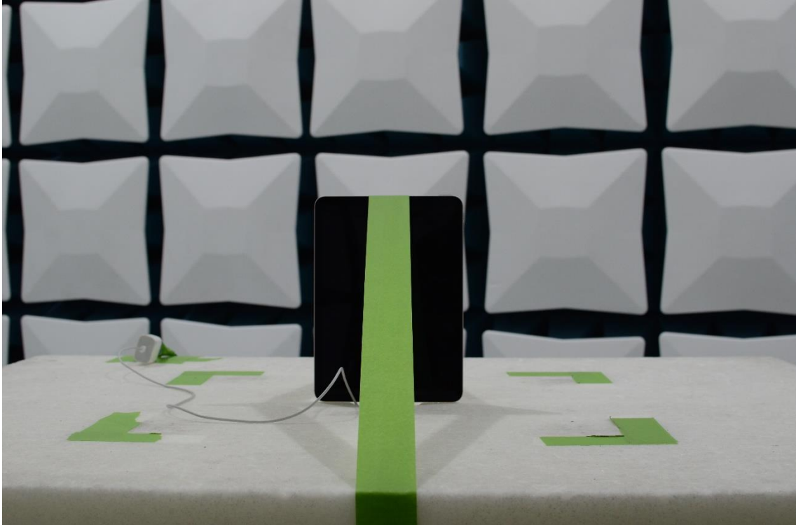
Figure 11: 30MHz-1GHz Test Setup (Front View)
