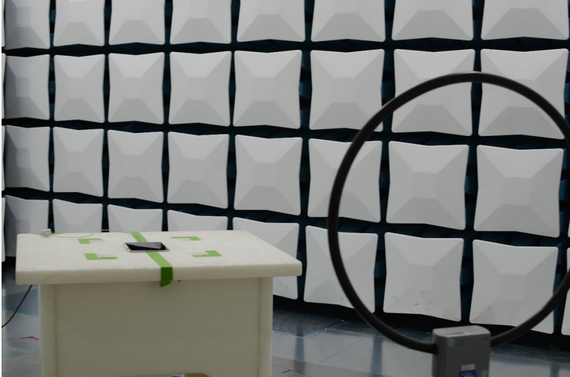
Figure 19: 9kHz-30MHz Test Setup (Front View)
