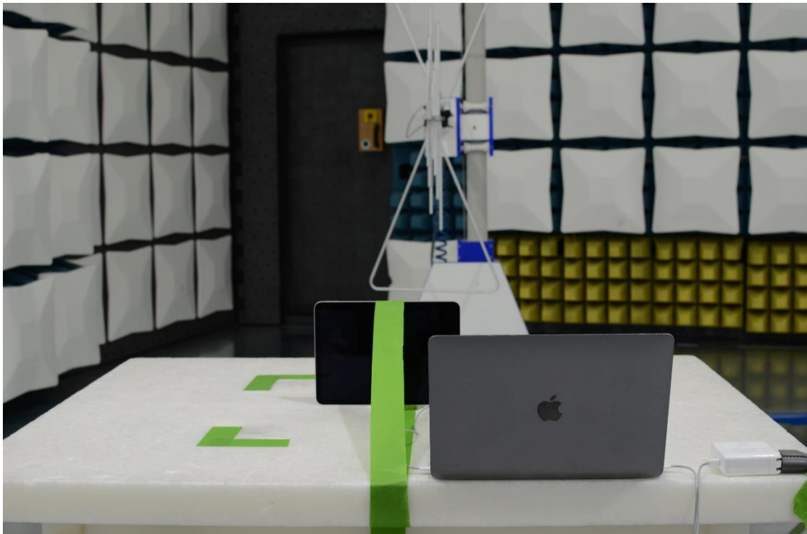
Figure 16: 30MHz-1GHz Test Setup (Rear View)
