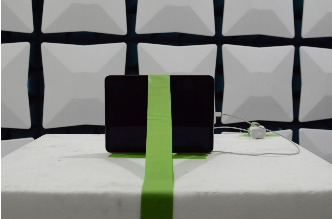
Figure 3: 1-18GHz Test Setup (Front View)
