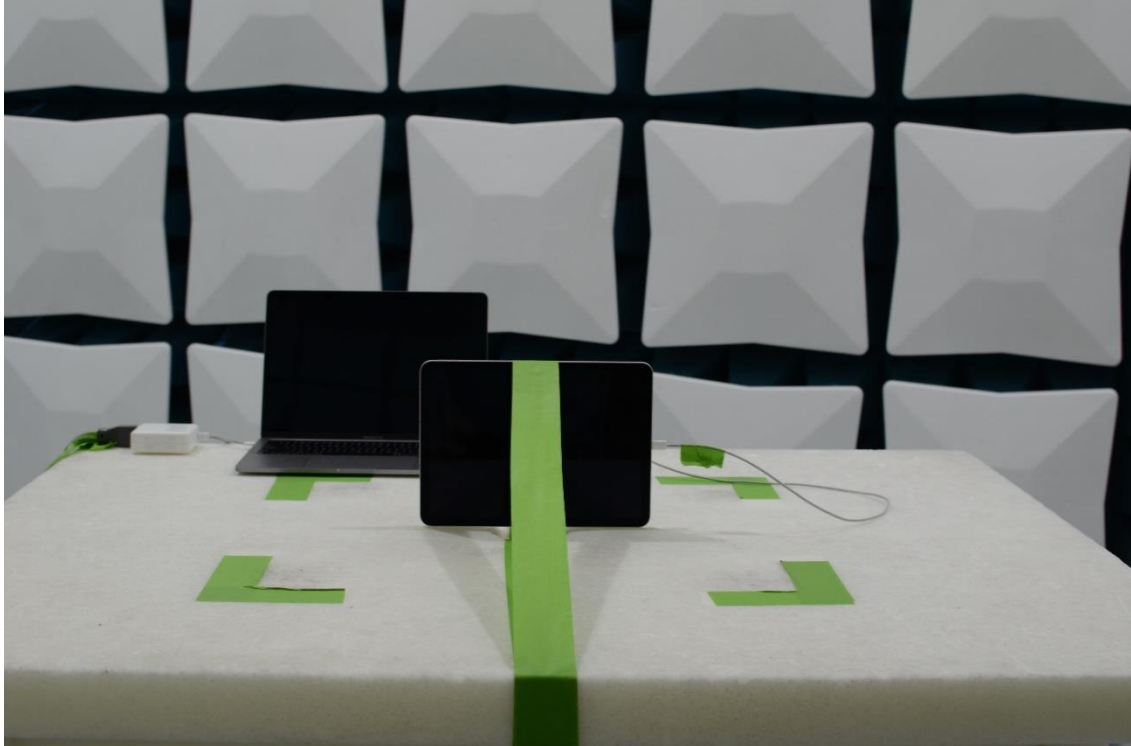
Figure 15: 30MHz-1GHz Test Setup (Front View)
