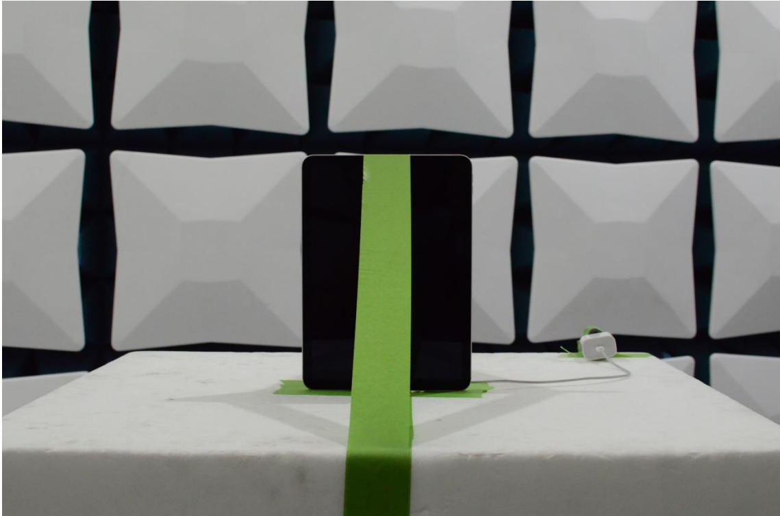
Figure 5: 1-18GHz Test Setup (Front View)
