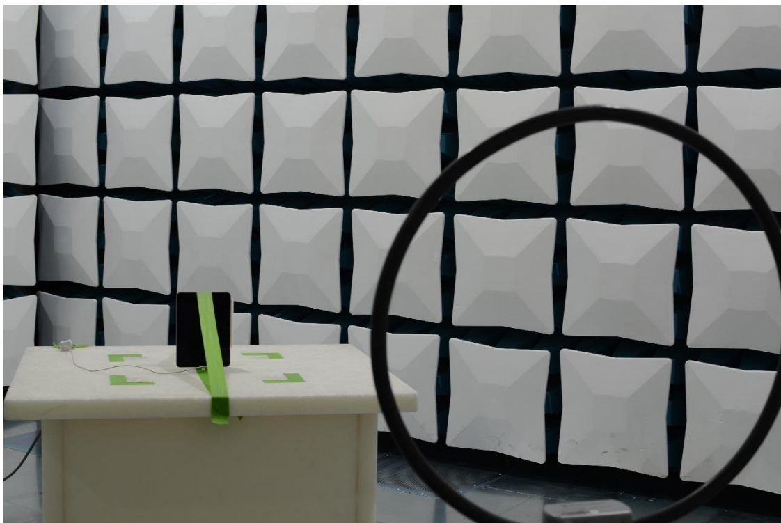
Figure 21: 9kHz-30MHz Test Setup (Front View)
