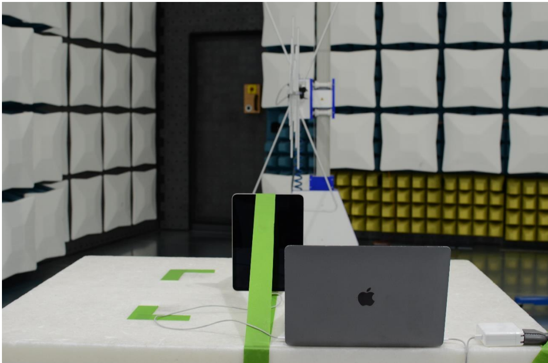
Figure 18: 30MHz-1GHz Test Setup (Rear View)
