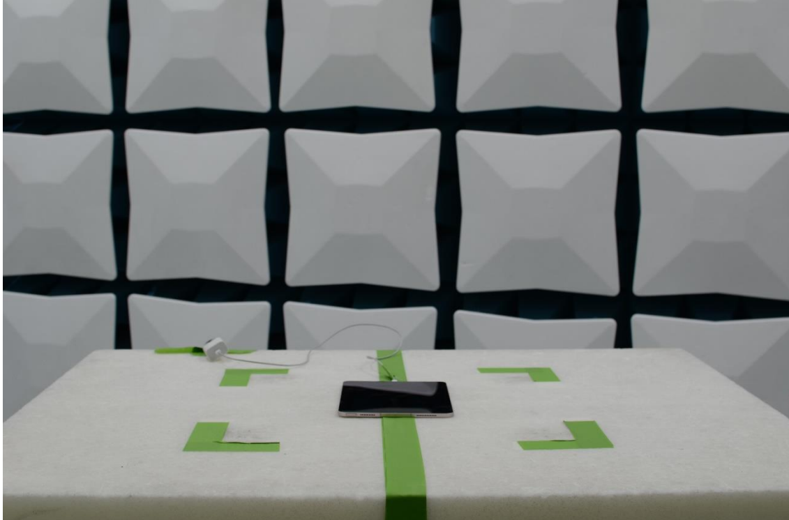
Figure 7: 30MHz-1GHz Test Setup (Front View)
