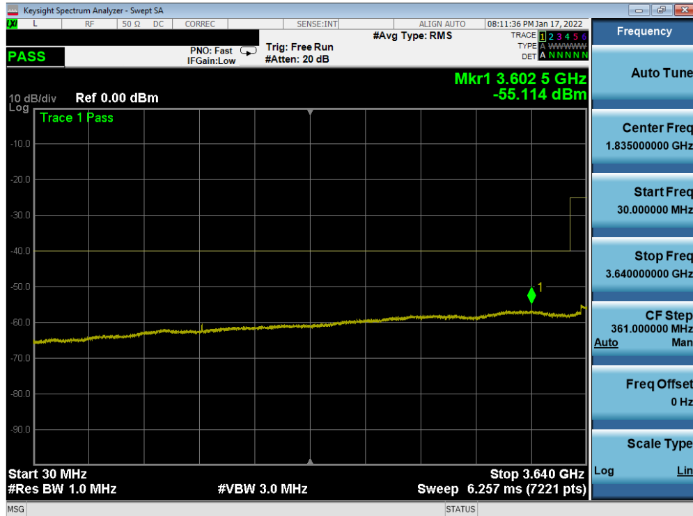
Plot 7-41. Conducted Spurious Plot (LTE Band 48 - 20MHz QPSK - High Channel)
