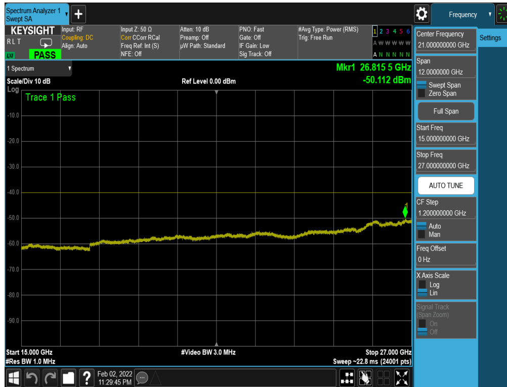
Plot 7-39. Conducted Spurious Plot (LTE Band 48 - 20MHz QPSK - Mid Channel)
