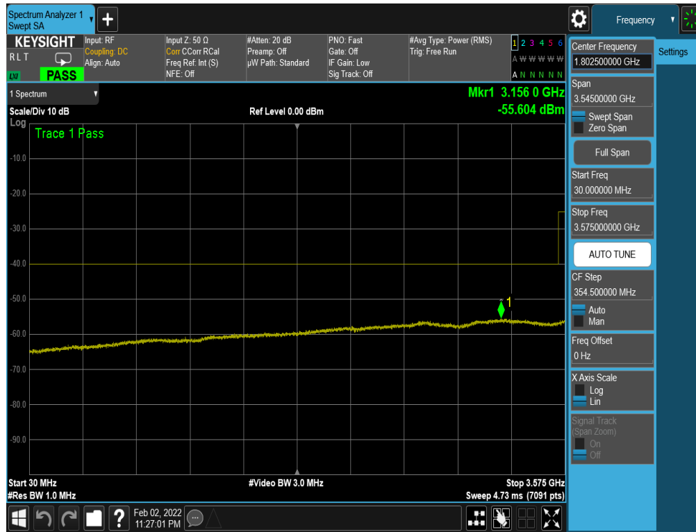
Plot 7-37. Conducted Spurious Plot (LTE Band 48 - 20MHz QPSK - Mid Channel)
