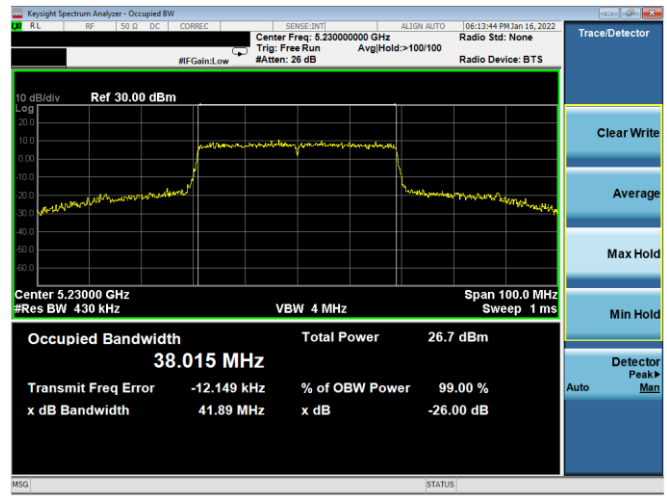
Plot 7-76. 26dB BW & 99% OBW Antenna 1B (40MHz BW 802.11ax(SU) – Ch. 46, MCS3)
