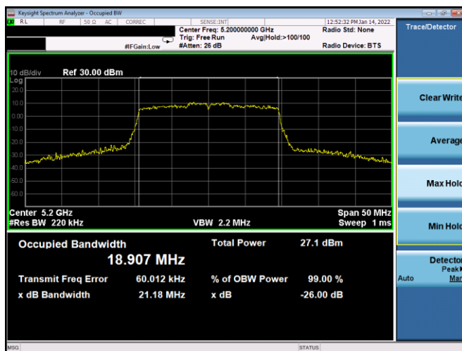
Plot 7-74. 26dB BW & 99% OBW Antenna 1B (20MHz BW 802.11ax(SU) – Ch. 40, MCS3)
