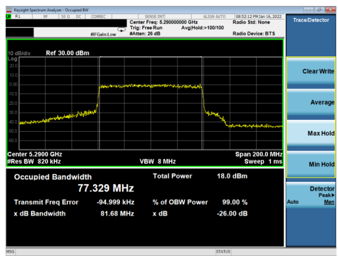
Plot 7-102. 26dB BW & 99% OBW Antenna 1B (80MHz BW 802.11ax(SU) – Ch. 58, MCS5)
