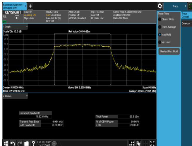
Plot 7-68. 26dB BW & 99% OBW Antenna 1B (20MHz BW 802.11ax(SU) – Ch. 116, MCS0)
