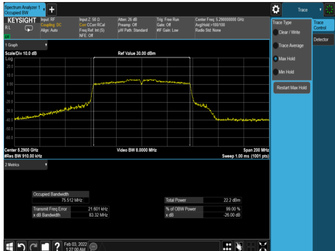
Plot 7-65. 26dB BW & 99% OBW Antenna 1B (80MHz BW 802.11ac – Ch. 58, MCS0)
