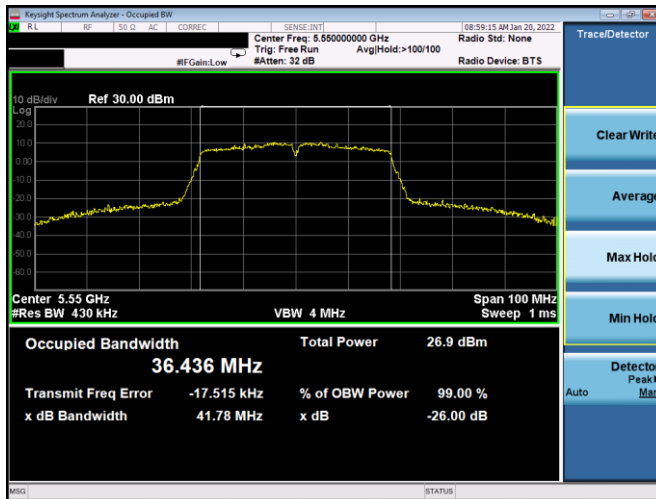
Plot 7-15. 26dB BW & 99% OBW Antenna 2B (40MHz BW 802.11n – Ch. 110, MCS0)
