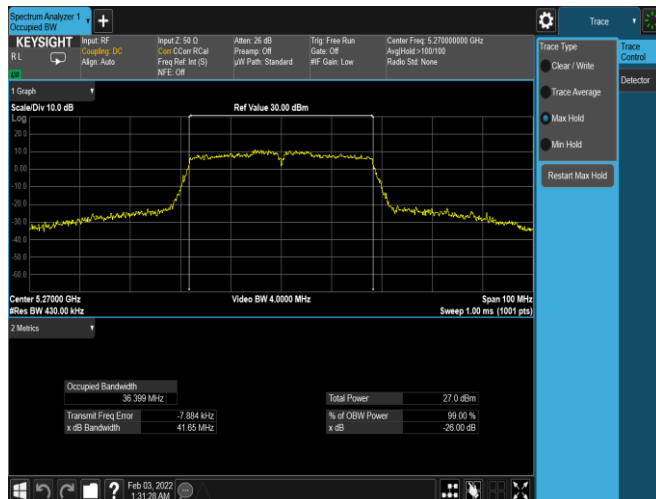
Plot 7-63. 26dB BW & 99% OBW Antenna 1B (40MHz BW 802.11n – Ch. 54, MCS0)
