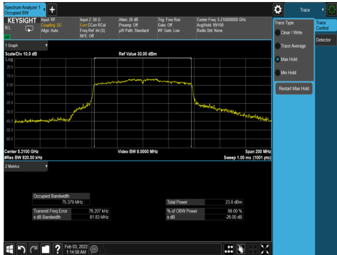
Plot 7-59. 26dB BW & 99% OBW Antenna 1B (80MHz BW 802.11ac – Ch. 42, MCS0)
