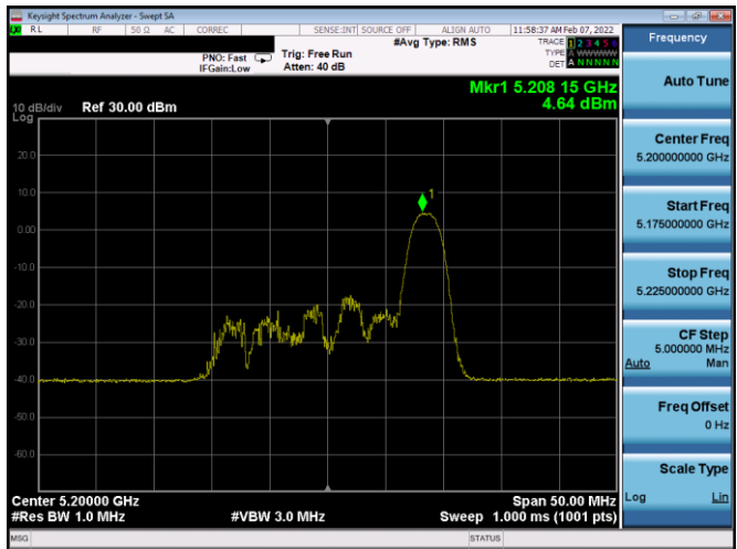
Plot 7-545. ISED PSD SDM Diversity Antenna 2b (20MHz BW 11ax Index 8 – RU26 – Ch.40)
