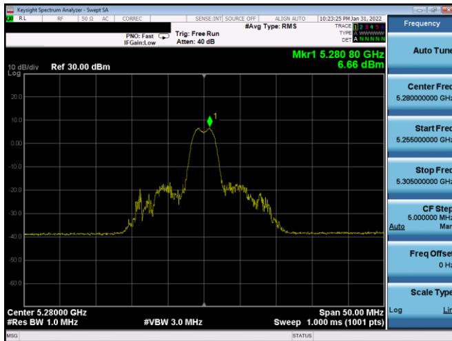
Plot 7-218. PSD Antenna 1b (20MHz BW 11ax Index 4 – RU26 – Ch.56)
