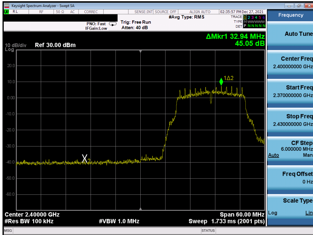
Plot 7-176. Band Edge Plot Antenna 3a (802.11g- Ch. 2) – 6Mbps
