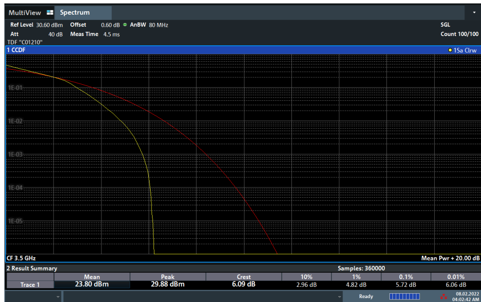
Plot 7-126. PAR Plot (NR Band n77 - 50MHz DFT-s-OFDM 16-QAM - Full RB)
