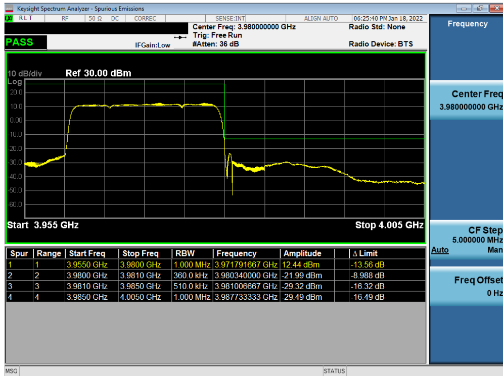
Plot 7-218. Upper ACP Plot (NR Band n77 C-Band - 20MHz DFT-s-OFDM \pi/2 BPSK – Full RB)
