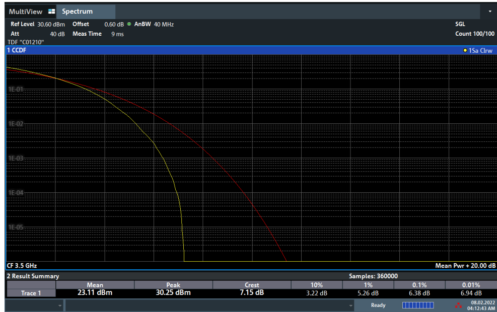
Plot 7-117. PAR Plot (NR Band n77 - 30MHz DFT-s-OFDM 64-QAM - Full RB)
