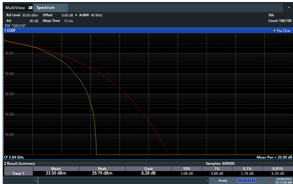
Plot 7-161. PAR Plot (NR Band n77 - 30MHz DFT-s-OFDM 16-QAM - Full RB)
