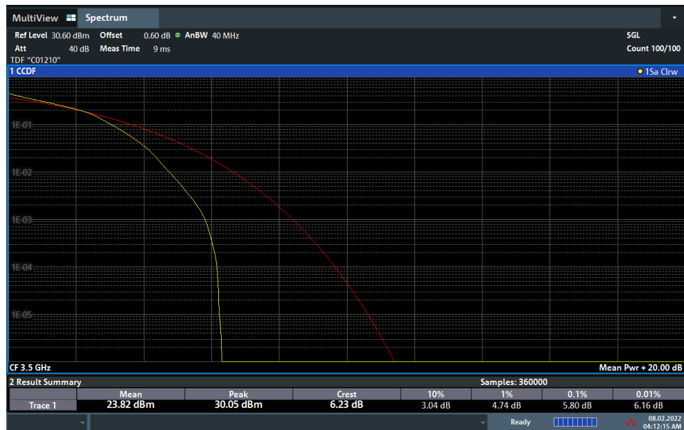
Plot 7-116. PAR Plot (NR Band n77 - 30MHz DFT-s-OFDM 16-QAM - Full RB)
