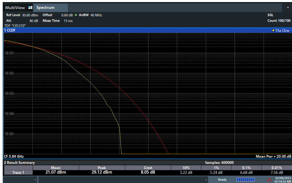
Plot 7-163. PAR Plot (NR Band n77 - 30MHz DFT-s-OFDM 256-QAM - Full RB)
