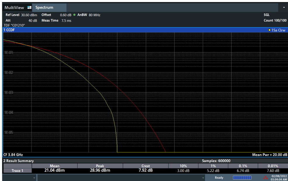
Plot 7-173. PAR Plot (NR Band n77 - 50MHz DFT-s-OFDM 256-QAM - Full RB)
