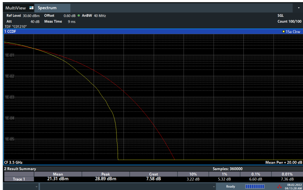
Plot 7-118. PAR Plot (NR Band n77 - 30MHz DFT-s-OFDM 256-QAM - Full RB)
