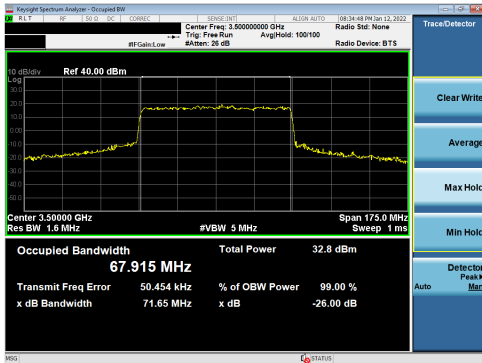
Plot 7-28. Occupied Bandwidth Plot (NR Band n77 DoD Band - 70MHz CP-OFDM 16-QAM - Full RB)
