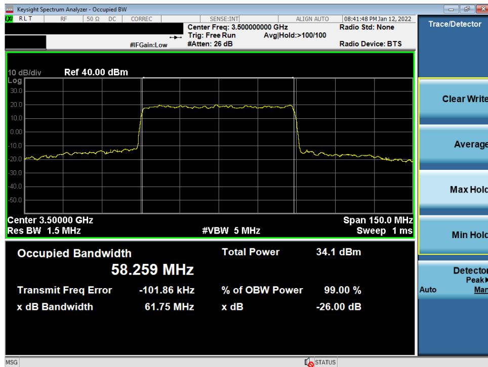
Plot 7-22. Occupied Bandwidth Plot (NR Band n77 DoD Band - 60MHz DFT-s-OFDM QPSK - Full RB)
