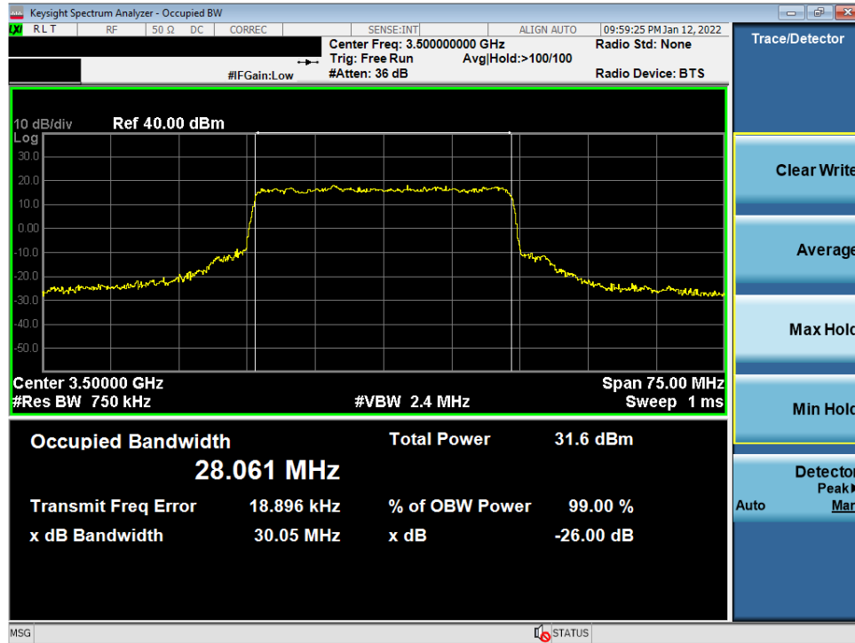
Plot 7-9. Occupied Bandwidth Plot (NR Band n77 DoD Band - 30MHz CP-OFDM 64-QAM - Full RB)
