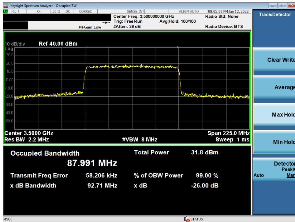
Plot 7-38. Occupied Bandwidth Plot (NR Band n77 DoD Band - 90MHz CP-OFDM 16-QAM - Full RB)
