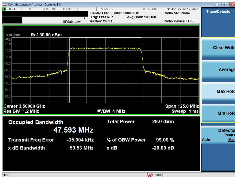
Plot 7-20. Occupied Bandwidth Plot (NR Band n77 DoD Band - 50MHz CP-OFDM 256-QAM - Full RB)
