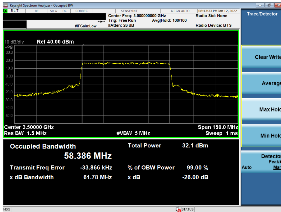
Plot 7-24. Occupied Bandwidth Plot (NR Band n77 DoD Band - 60MHz CP-OFDM 64-QAM - Full RB)
