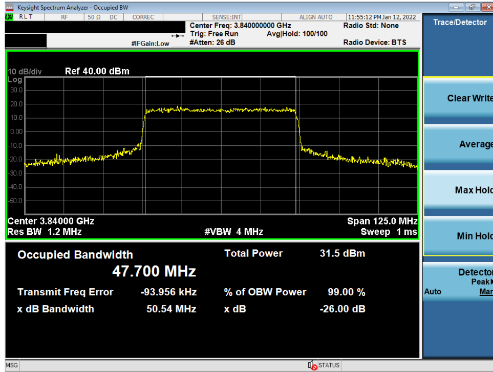
Plot 7-64. Occupied Bandwidth Plot (NR Band n77 C-Band - 50MHz CP-OFDM 64-QAM - Full RB)
