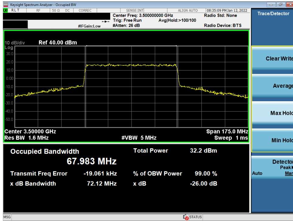
Plot 7-29. Occupied Bandwidth Plot (NR Band n77 DoD Band - 70MHz CP-OFDM 64-QAM - Full RB)
