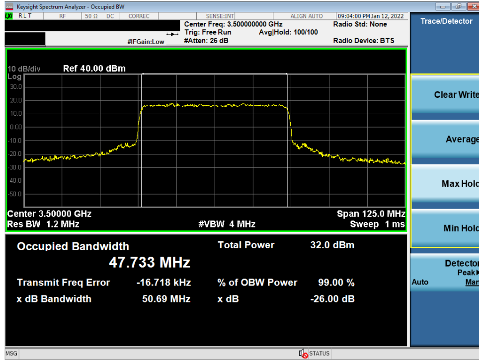
Plot 7-19. Occupied Bandwidth Plot (NR Band n77 DoD Band - 50MHz CP-OFDM 64-QAM - Full RB)
