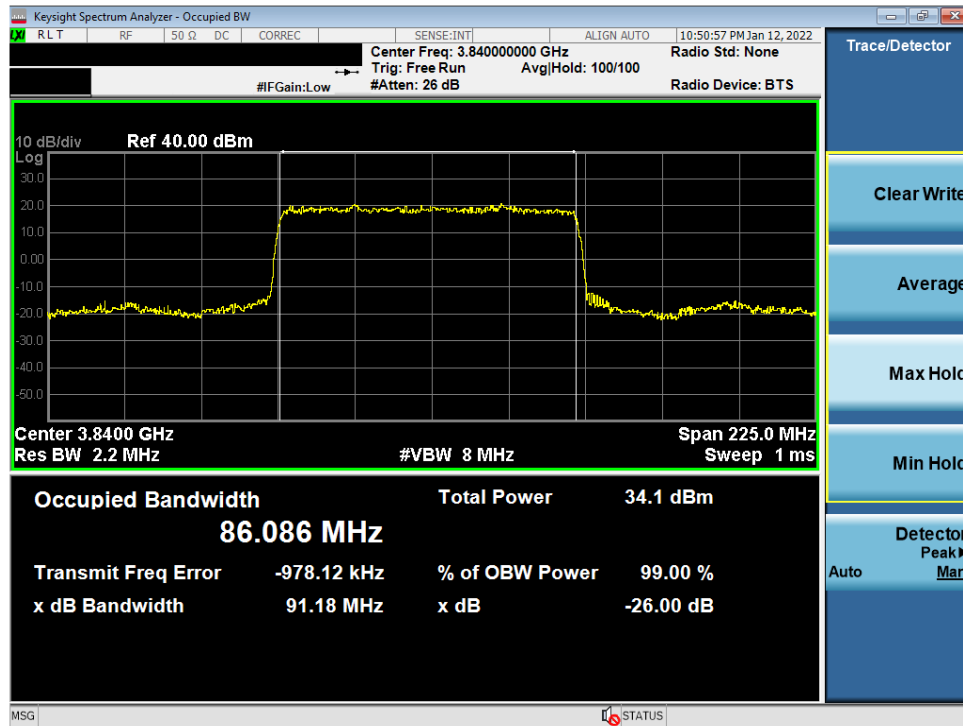
Plot 7-81. Occupied Bandwidth Plot (NR Band n77 C-Band - 90MHz DFT-s-OFDM \pi/2 BPSK - Full RB)
