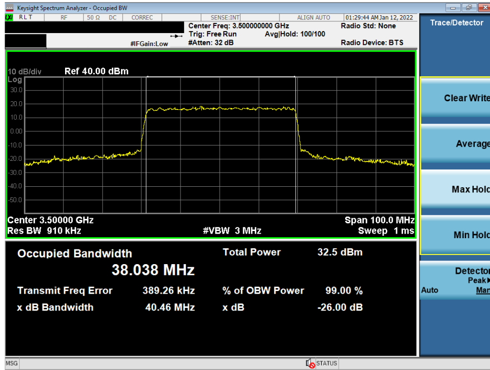
Plot 7-13. Occupied Bandwidth Plot (NR Band n77 DoD Band - 40MHz CP-OFDM 16-QAM - Full RB)
