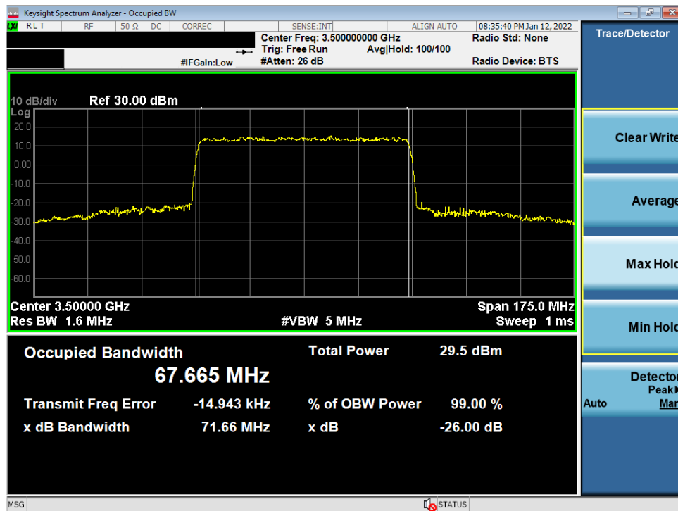
Plot 7-30. Occupied Bandwidth Plot (NR Band n77 DoD Band - 70MHz CP-OFDM 256-QAM - Full RB)
