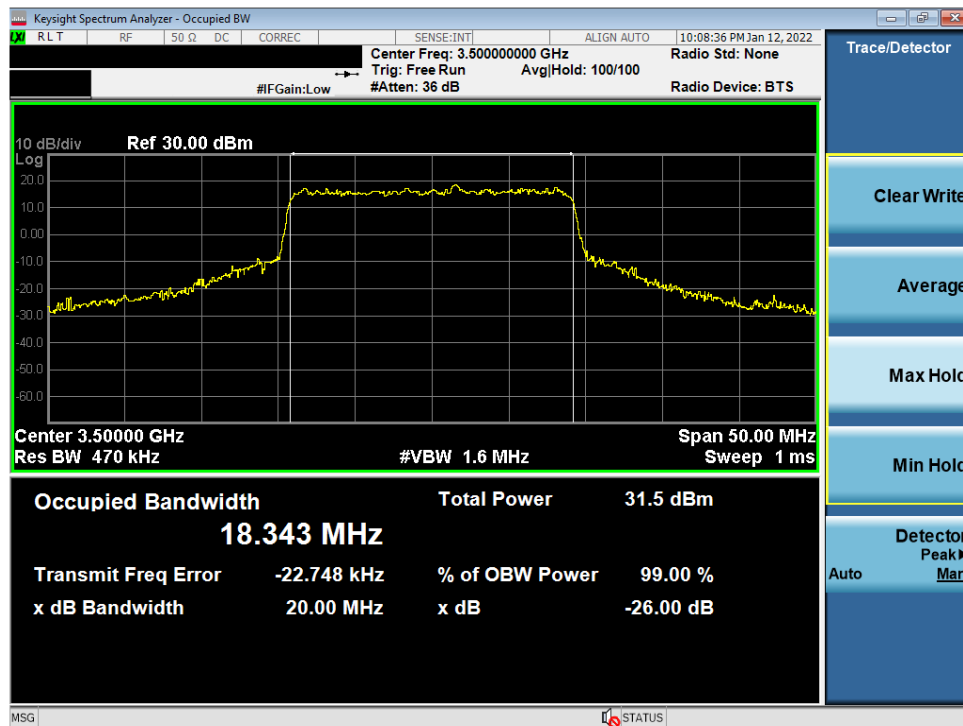
Plot 7-4. Occupied Bandwidth Plot (NR Band n77 DoD Band - 20MHz CP-OFDM 64-QAM - Full RB)
