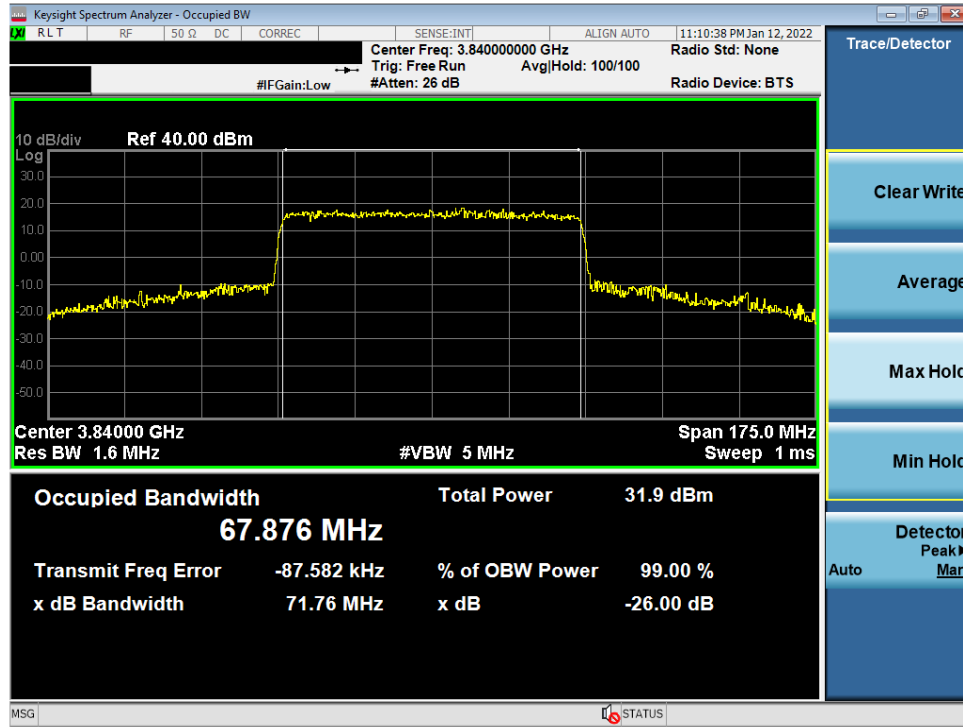
Plot 7-74. Occupied Bandwidth Plot (NR Band n77 C-Band - 70MHz CP-OFDM 64-QAM - Full RB)
