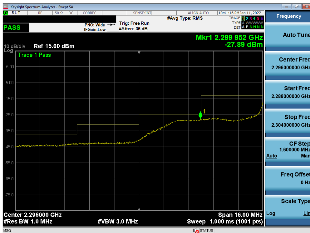
Plot 7-243. Extended Lower Band Edge Plot (NR Band n30 - 10MHz DFT-s-OFDM \pi/2 BPSK – Full RB)
