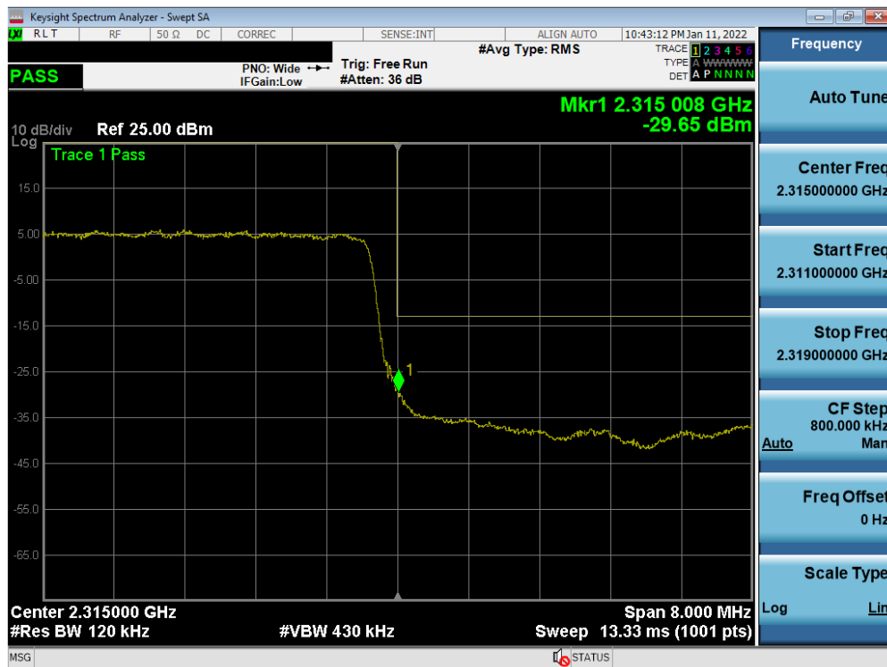
Plot 7-244. Upper Band Edge Plot (NR Band n30 - 10MHz DFT-s-OFDM \pi/2 BPSK – Full RB)
