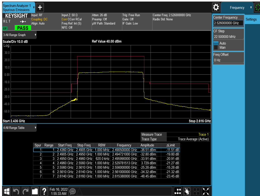
Plot 7-279. Lower ACP Plot (NR Band n41 - 60MHz CP-OFDM QPSK – Full RB)
