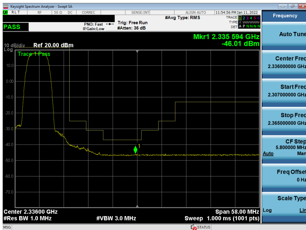
Plot 7-241. Extended Upper Band Edge Plot (NR Band n30 - 5MHz DFT-s-OFDM \pi/2 BPSK – Full RB)
