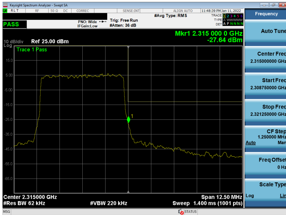
Plot 7-240. Upper Band Edge Plot (NR Band n30 - 5MHz DFT-s-OFDM QPSK – Full RB)
