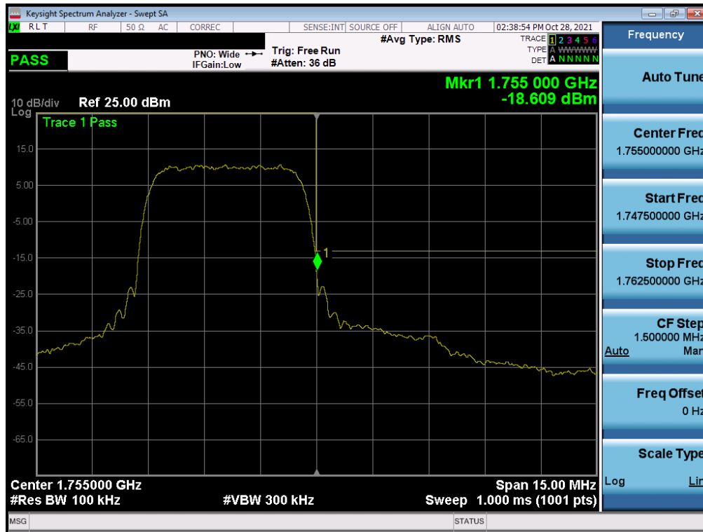
Plot 7-328. Upper Band Edge Plot (WCDMA AWS – Ch. 1513)
