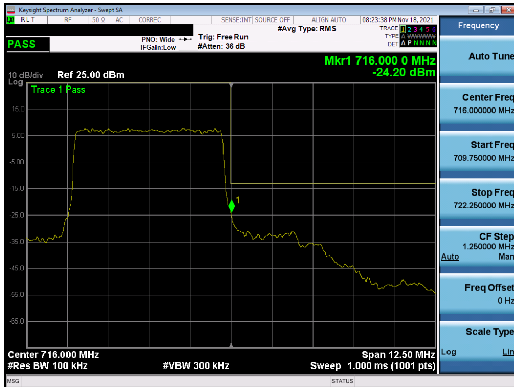
Plot 7-319. Upper Band Edge Plot (NR Band n12 – 5.0MHz DFT-s-OFDM \pi/2 BPSK - Full RB)
