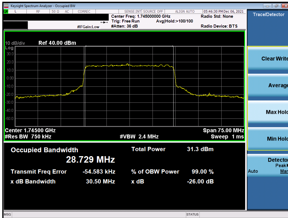
Plot 7-88. Occupied Bandwidth Plot (NR Band n66 - 30.0MHz CP-OFDM 64QAM - Full RB)
