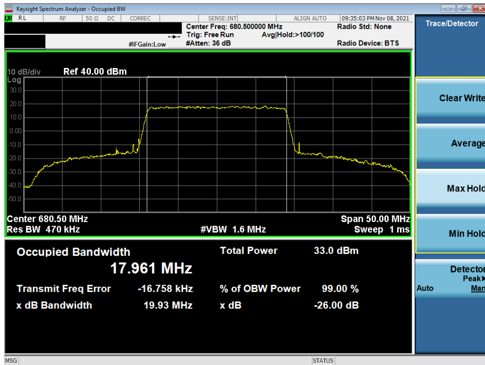
Plot 7-38. Occupied Bandwidth Plot (LTE Band 71 - 20MHz 16-QAM - Full RB)
