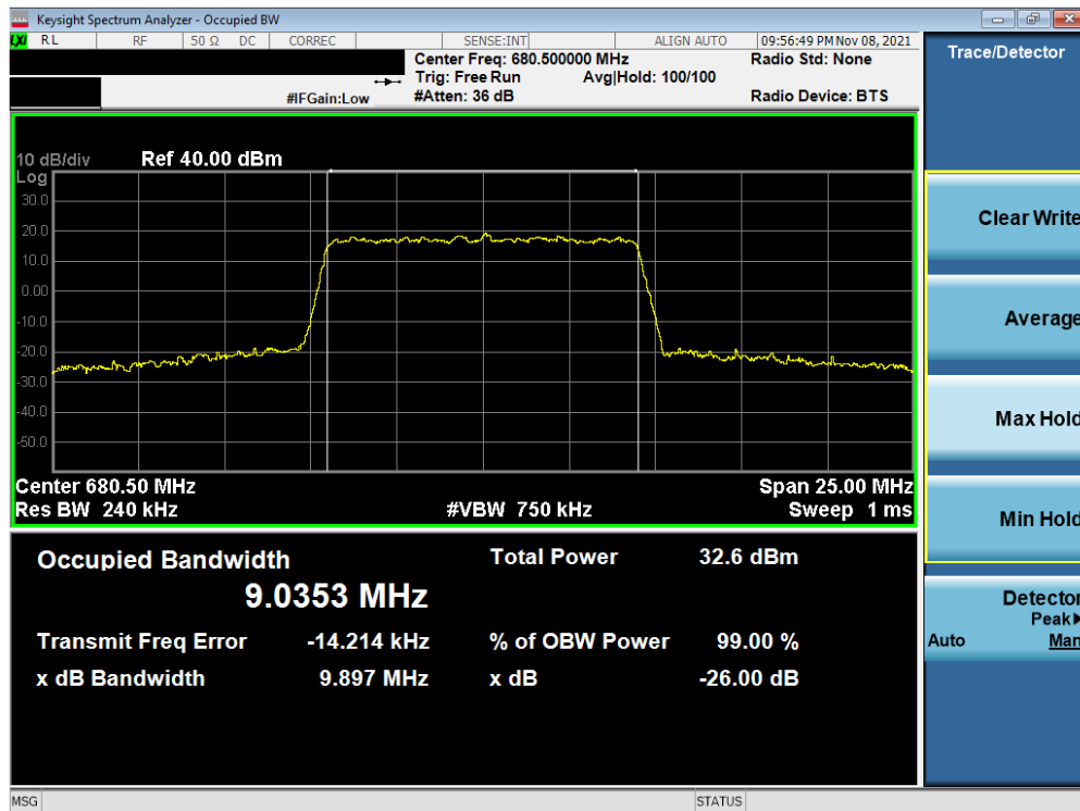
Plot 7-30. Occupied Bandwidth Plot (LTE Band 71 - 10MHz 16-QAM - Full RB)
