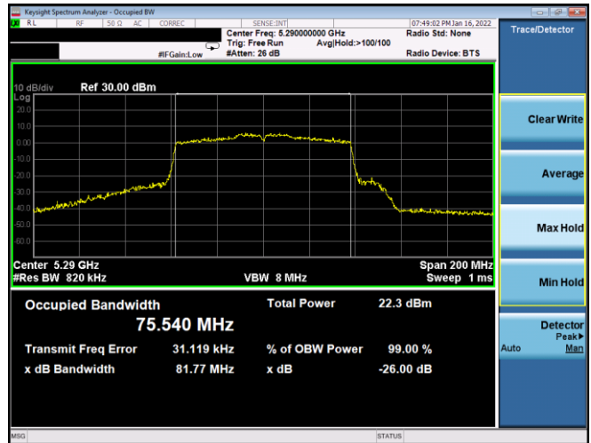
Plot 7-29. 26dB BW & 99% OBW Antenna WF8 (80MHz BW 802.11ac – Ch. 58, MCS3)
