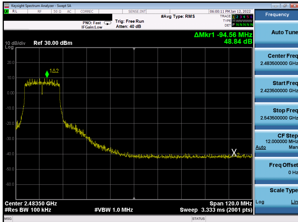
Plot 7-286. Band Edge Plot Antenna WF8 (802.11n (2.4GHz) – Ch. 6 (high)) – MCS5
