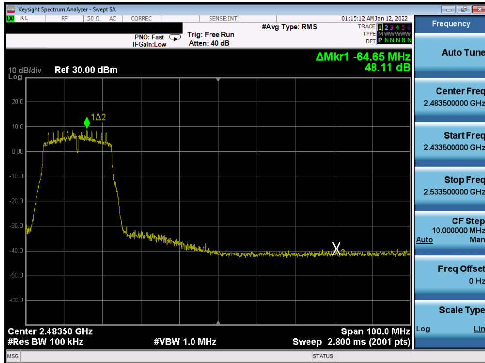
Plot 7-197. Band Edge Plot Antenna WF8 (802.11n (2.4GHz) – Ch. 8) – MCS0
