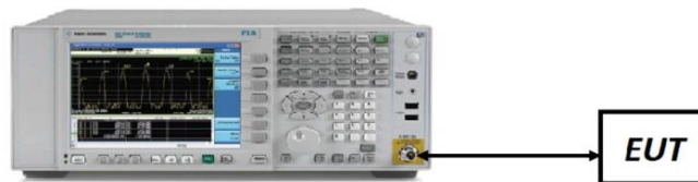
Figure 7-3. Test Instrument & Measurement Setup
