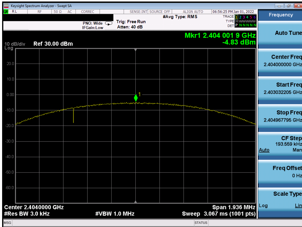
Plot 7-31. Power Spectral Density Plot Antenna WF7b (Bluetooth (LE), 2Mbps, ePA – Ch. 1)
