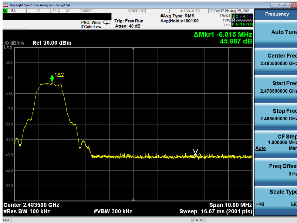
Plot 7-12. Band Edge Plot (Bluetooth with Hopping Disabled, 8DPSK, – Ch. 78)
