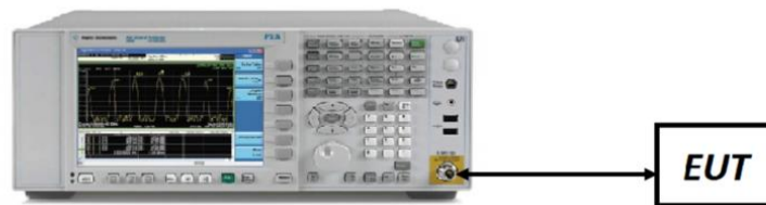
Figure 7-3. Test Instrument & Measurement Setup
