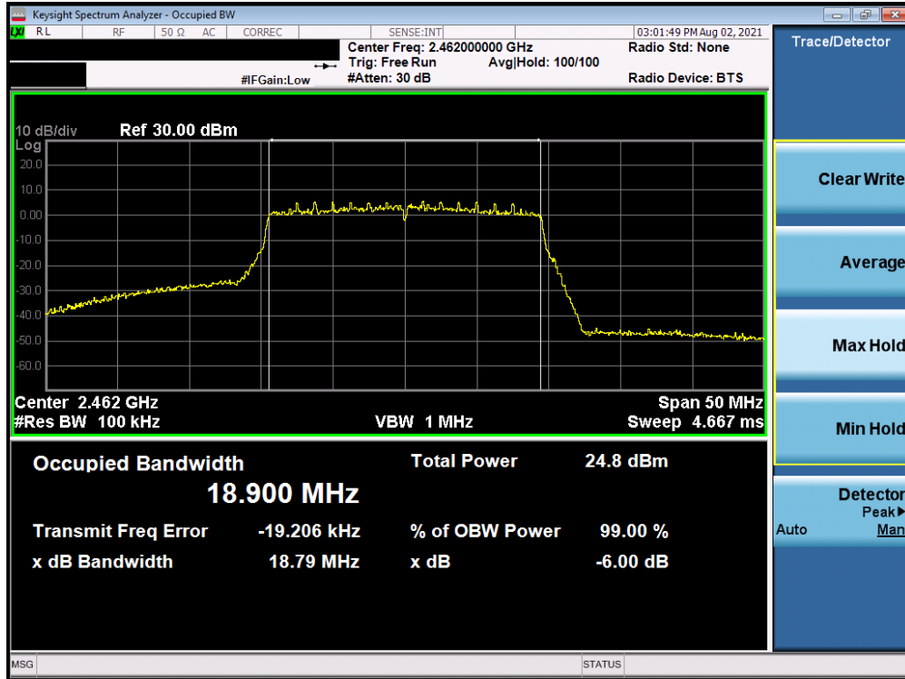
Plot 7-39. 6dB BW and 99% OBW Plot Antenna 1a (802. 11ax (SU - 2.4GHz) – Ch. 11) – MCS2
