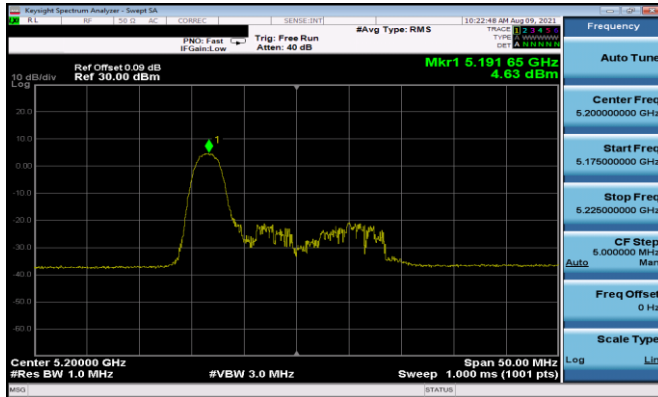
Plot 7-253. ISED PSD Antenna 3b (20MHz BW 11ax Index 0 - RU26 - Ch.40)
