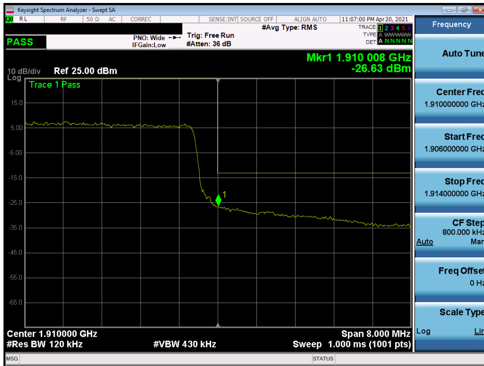
Plot 7-111. Upper Band Edge Plot (LTE Band 2 – 10MHz QPSK – Full RB Configuration)
