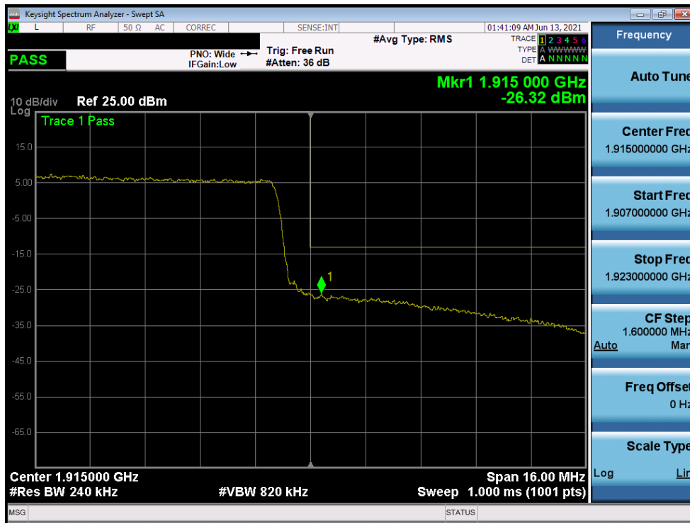
Plot 7-143. Upper Band Edge Plot (LTE Band 25/2 – 20MHz QPSK – Full RB Configuration)
