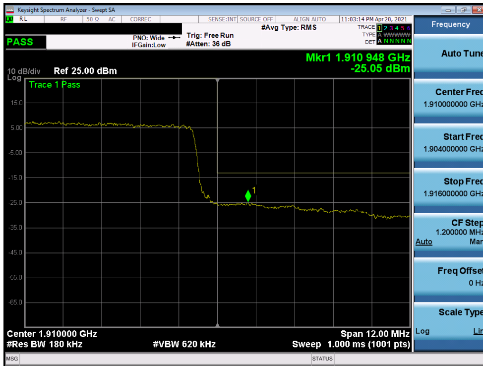
Plot 7-115. Upper Band Edge Plot (LTE Band 2 - 15MHz QPSK - Full RB Configuration)
