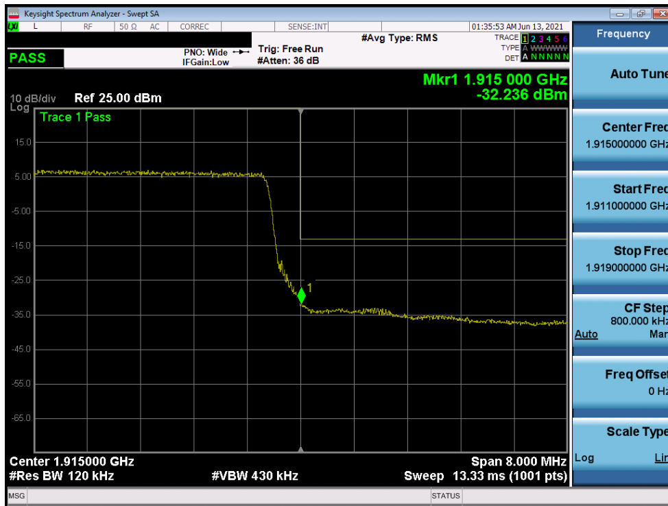
Plot 7-135. Upper Band Edge Plot (LTE Band 25/2 – 10MHz QPSK – Full RB Configuration)
