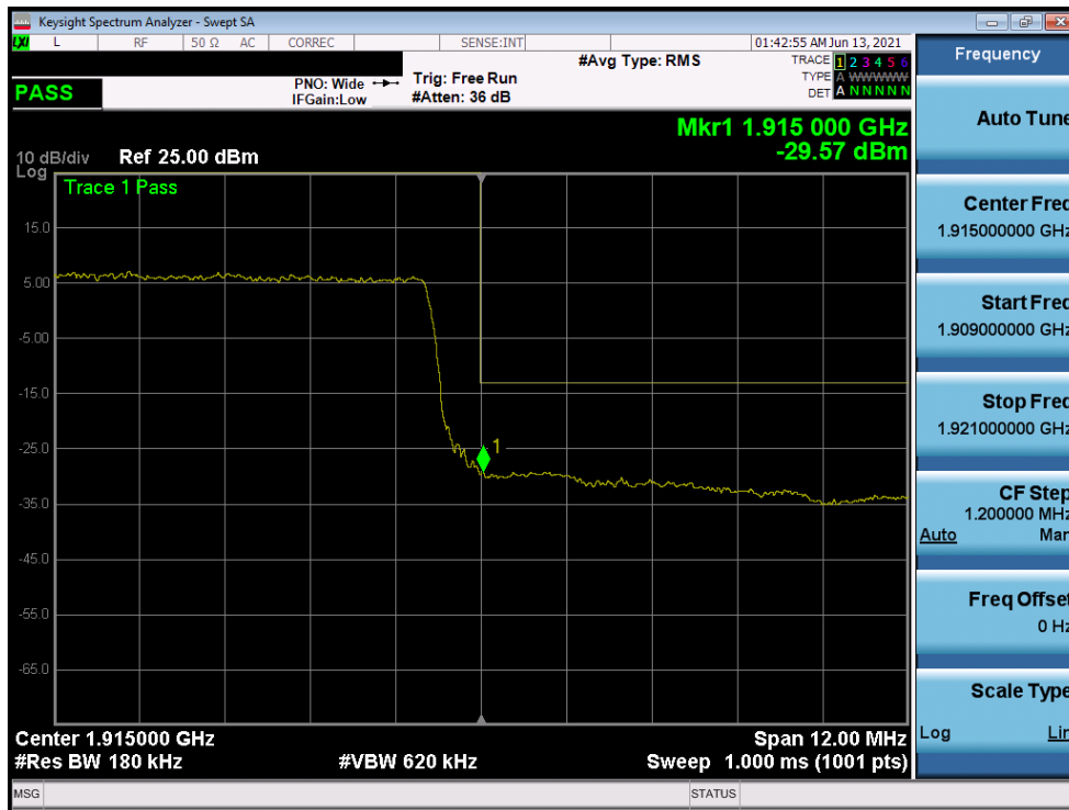
Plot 7-139. Upper Band Edge Plot (LTE Band 25/2 – 15MHz QPSK – Full RB Configuration)
