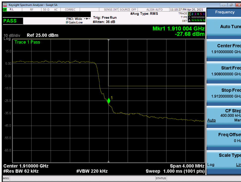
Plot 7-107. Upper Band Edge Plot (LTE Band 2 - 5MHz QPSK - Full RB Configuration)
