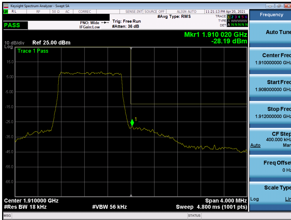
Plot 7-99. Upper Band Edge Plot (LTE Band 2 – 1.4MHz QPSK – Full RB Configuration)
