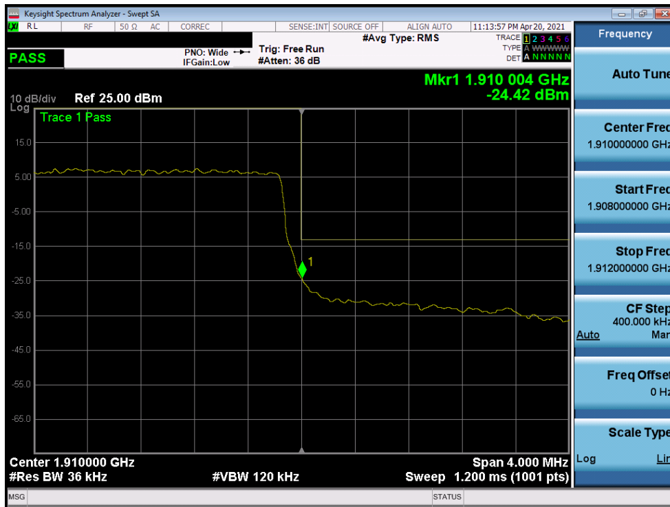
Plot 7-103. Upper Band Edge Plot (LTE Band 2 – 3MHz QPSK – Full RB Configuration)
