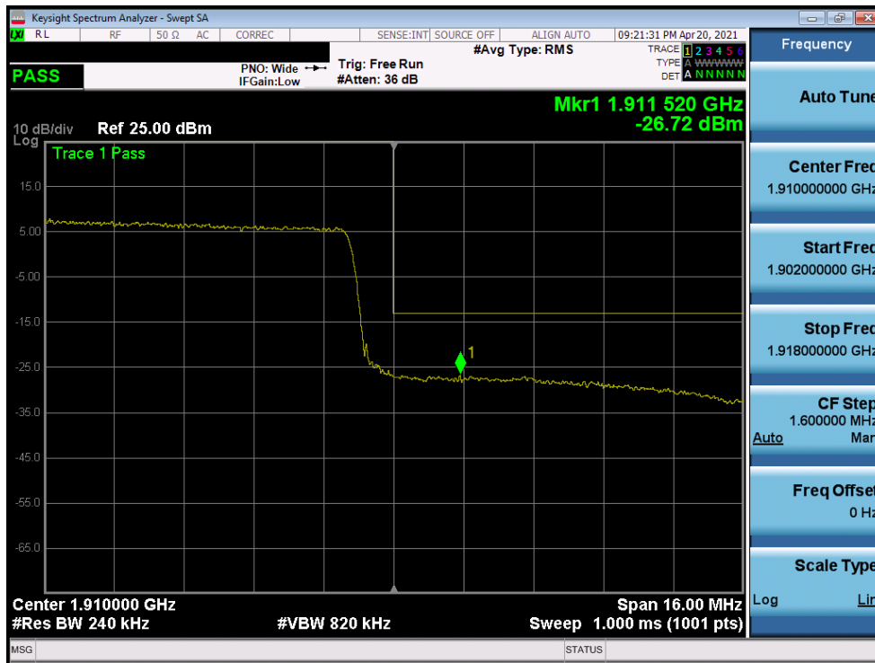
Plot 7-119. Upper Band Edge Plot (LTE Band 2 - 20MHz QPSK - Full RB Configuration)
