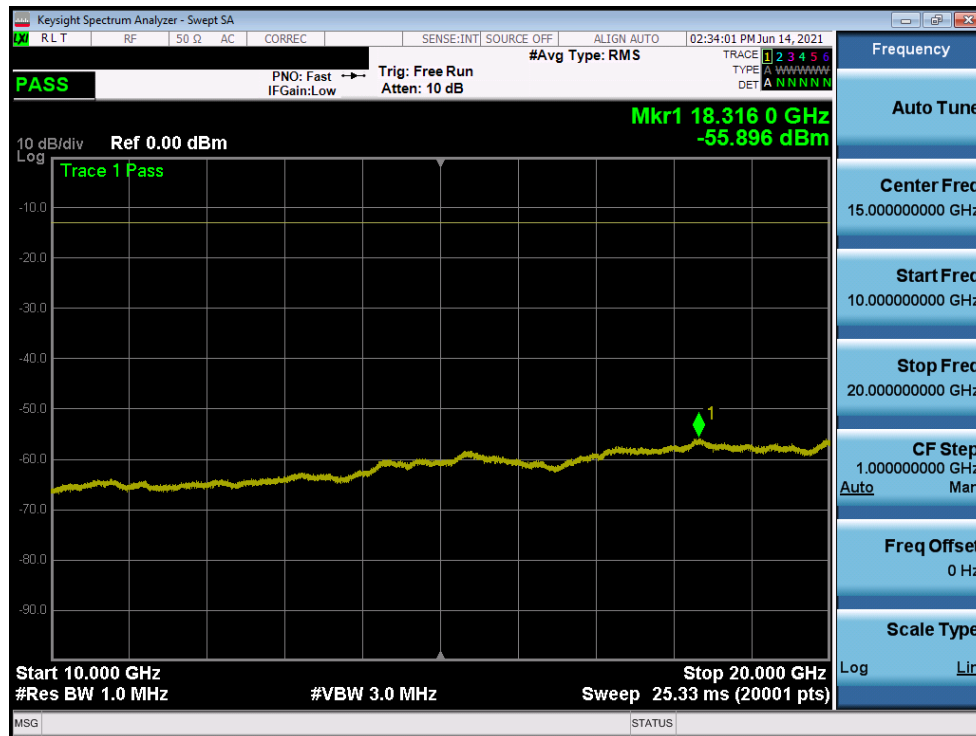
Plot 7-96. Conducted Spurious Plot (WCDMA Ch. 9538)
