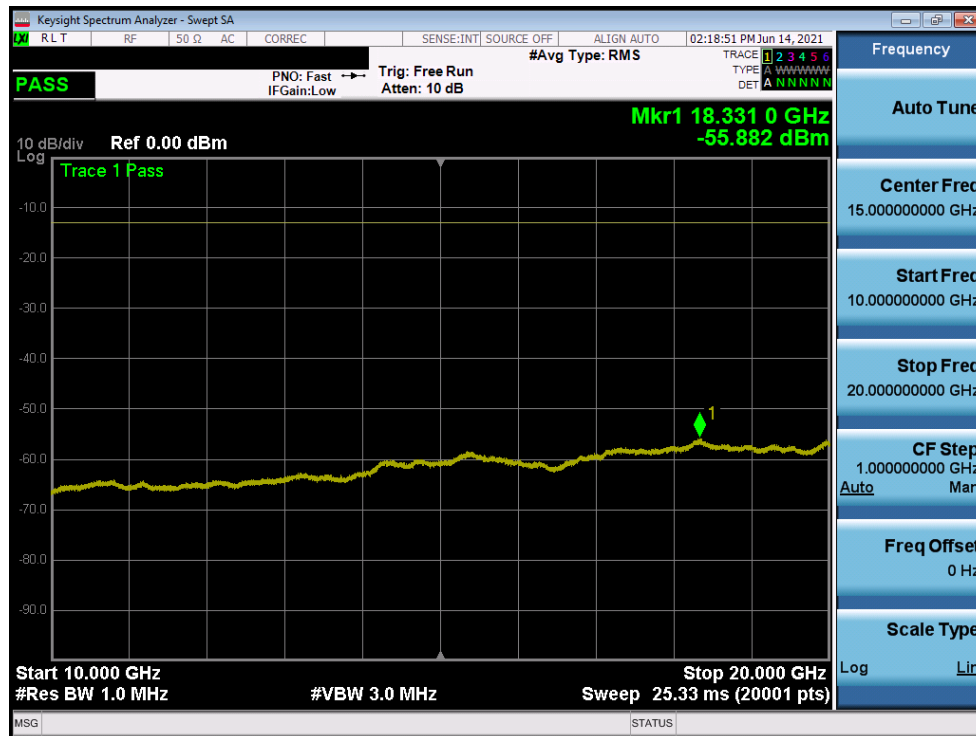
Plot 7-90. Conducted Spurious Plot (WCDMA Ch. 9262)
